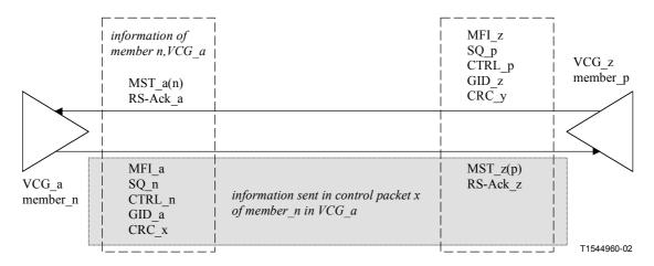
Figure 1/G.7042/Y.1305 – Allocation of information in a control packet
