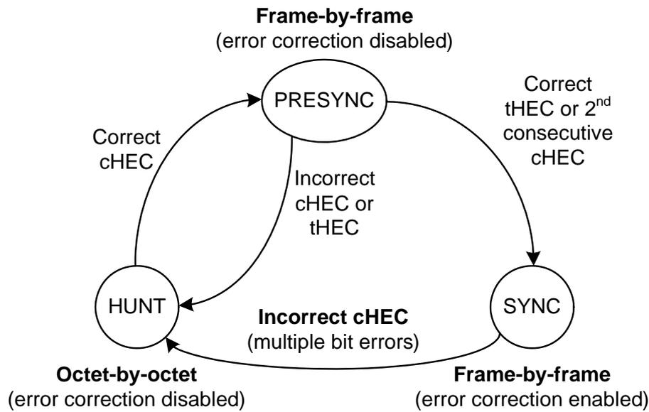
**Figure 6-13bis – GFP frame delineation state diagram using cHEC and tHEC**
