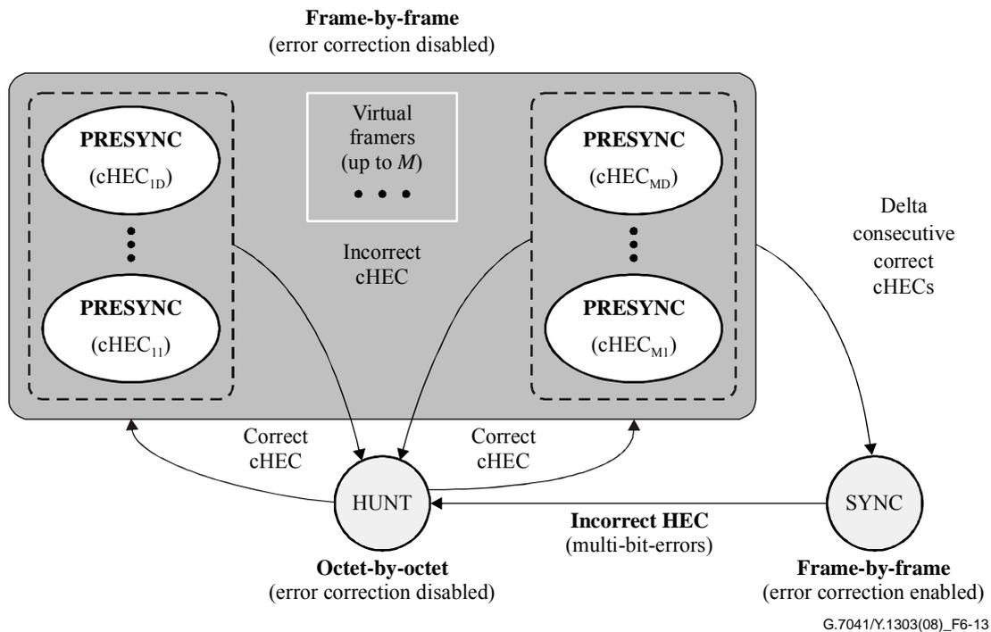
**Figure 6-13 – GFP frame delineation state diagram**
