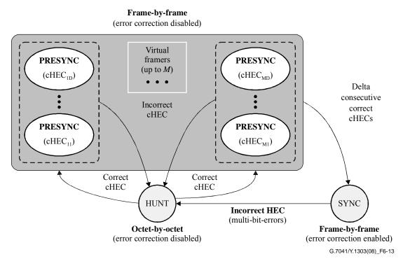
Figure 6-13 – GFP frame delineation state diagram
