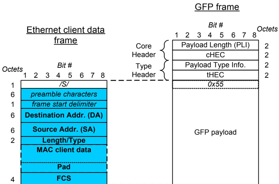
Figure 7-11 – Ethernet client data frame and preamble mapping into GFP-F
