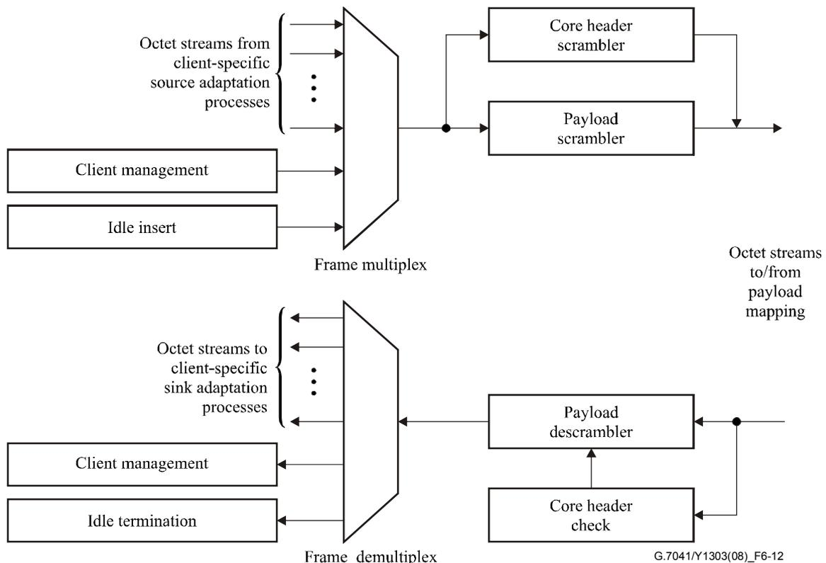
**Figure 6-12 – GFP common (protocol-independent) procedures**
