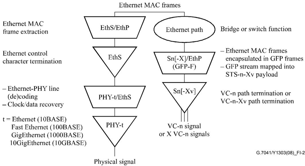
**Figure I.2 – Ethernet tributary interface port using GFP-F mapping in SDH network element**
