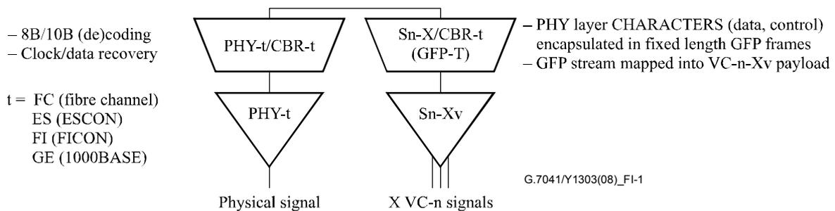
**Figure I.1 – FC/ES/FI/GE tributary interface port using full-rate GFP-T mapping in SDH network element**
