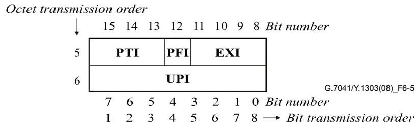
**Figure 6-5 – GFP type field format**
