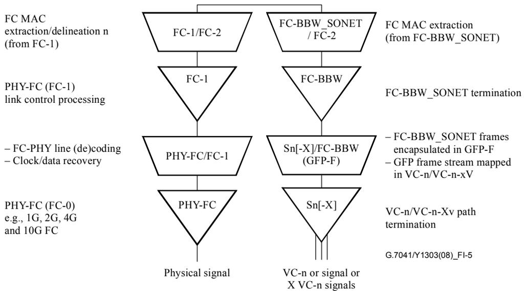
**Figure I.5 – Fibre channel tributary interface port using FC-BBW\_SONET and GFP-F mapping in an SDH network element**
