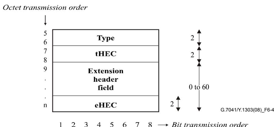
**Figure 6-4 – GFP payload header format**
