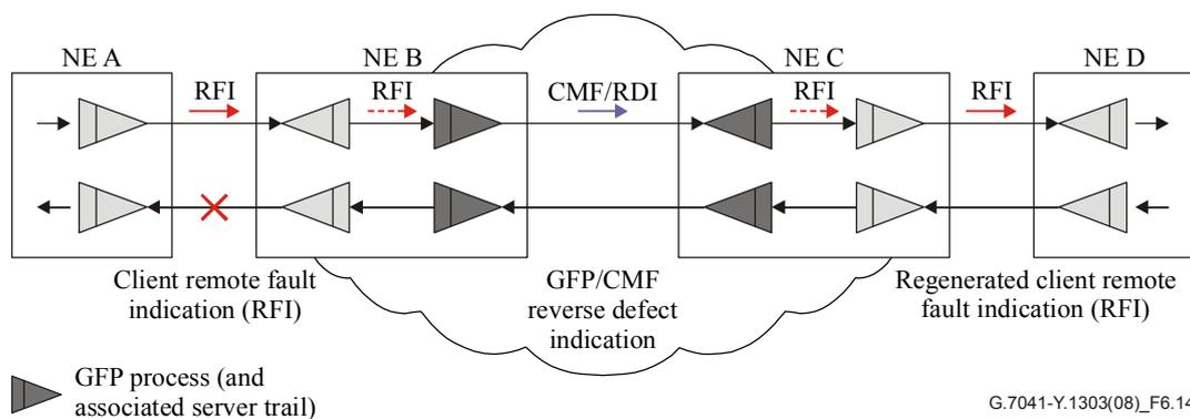
**Figure 6-14 – Examples of a reverse defect indication of a client link fault status indication**
