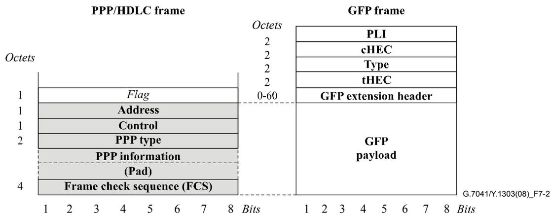
**Figure 7-2 – HDLC/PPP and GFP frame relationships**
