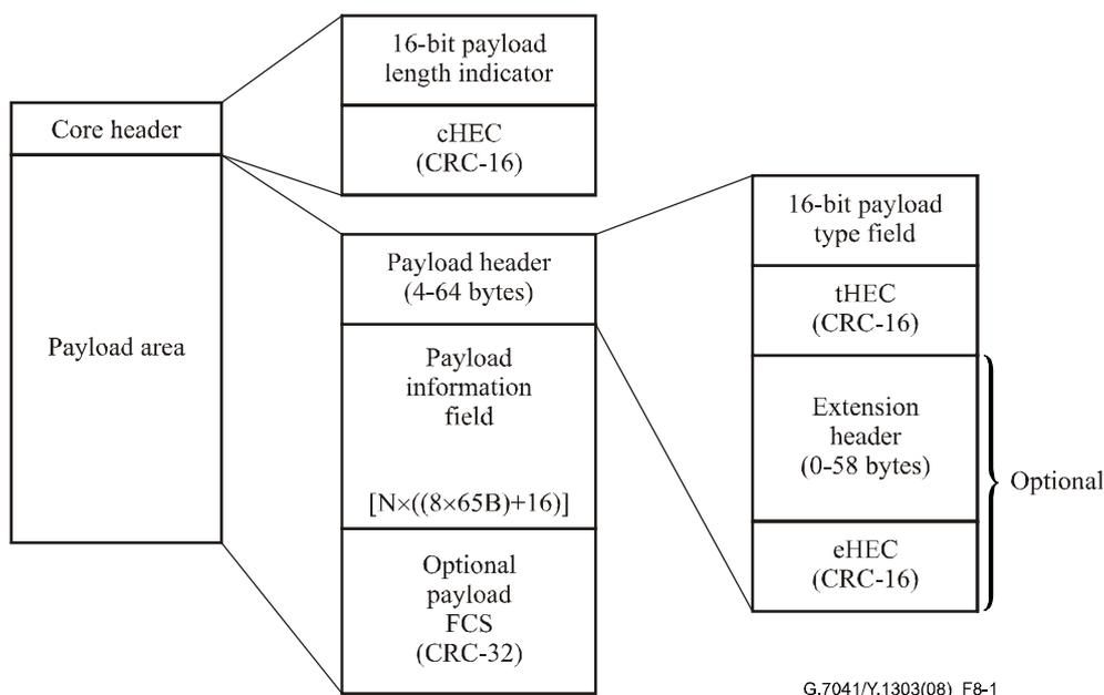
**Figure 8-1 – Transparent GFP frame format**
