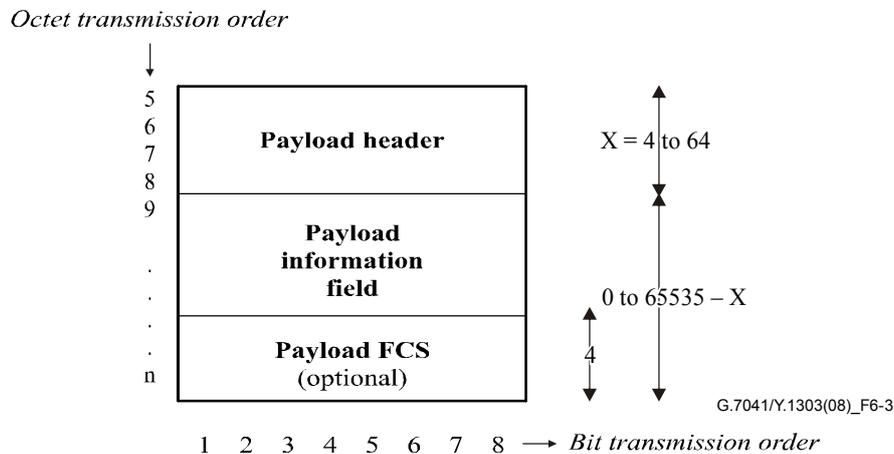
**Figure 6-3 – GFP payload area format**
