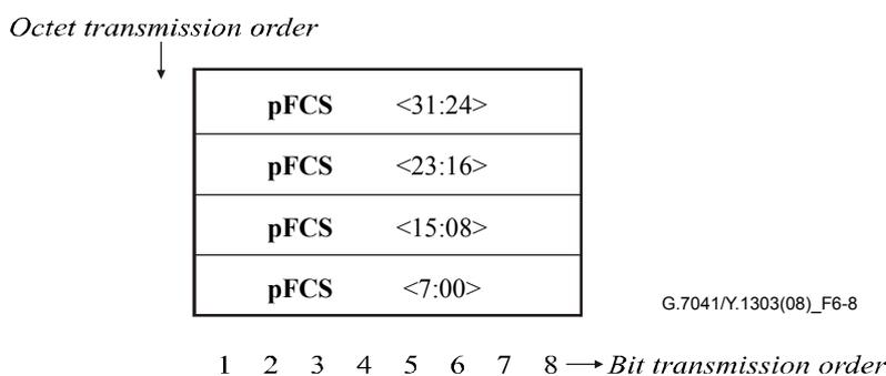
**Figure 6-8 – GFP payload frame check sequence format**
