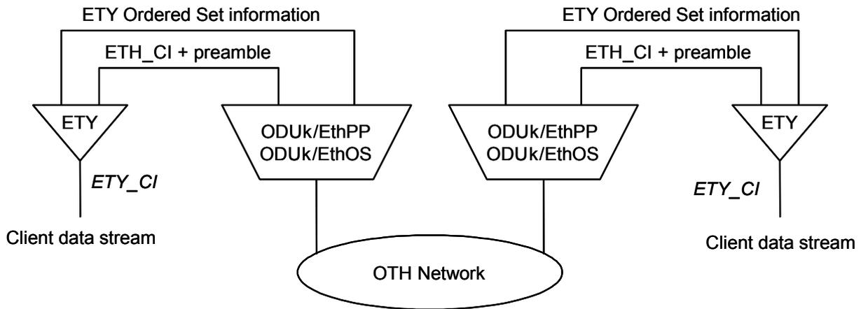
**Figure 7-10 – Functional model for mapping 10GBASE-R information into the ODUk**
