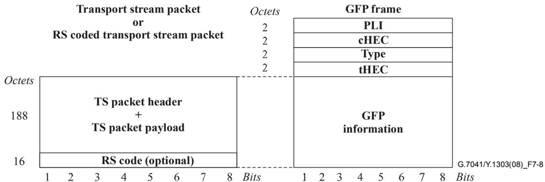
**Figure 7-8 – TS packet and GFP frame relationships**
