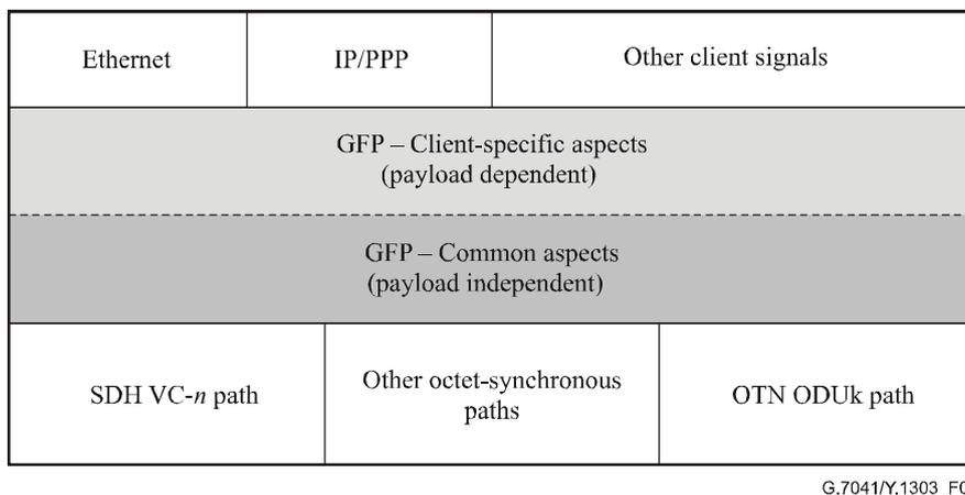
**Figure 1 – GFP relationship to client signals and transport paths**
