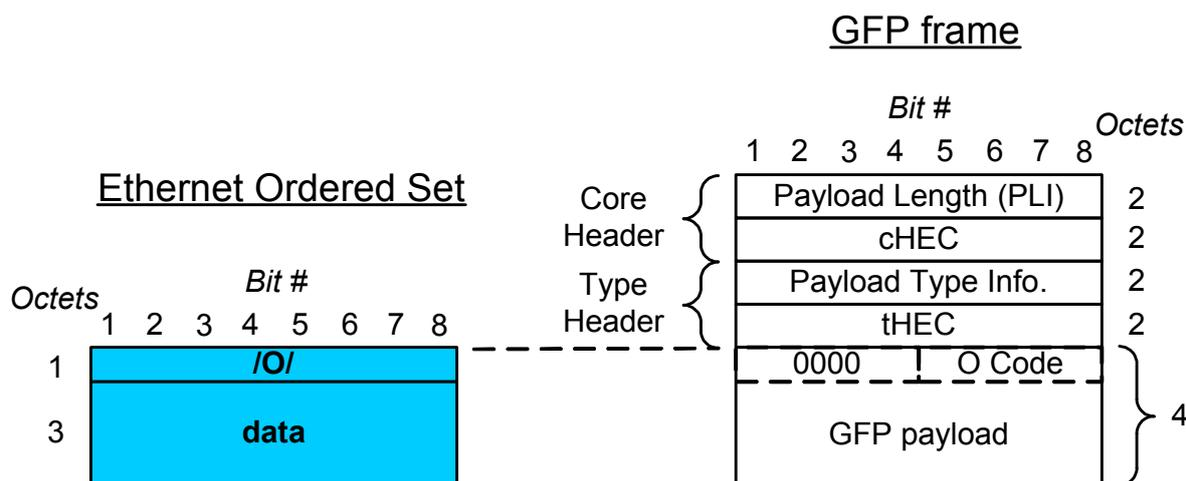
Figure 7-12 – Ethernet ordered set mapping into GFP-F
