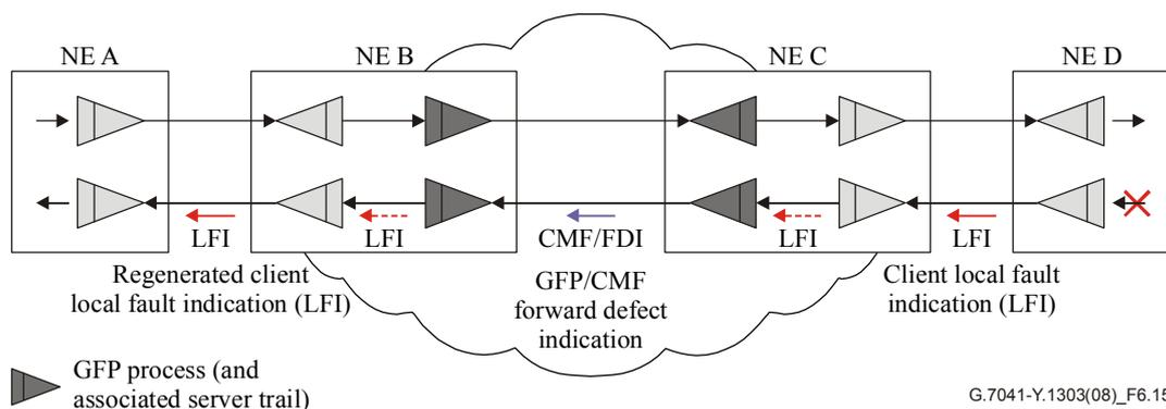
**Figure 6-15 – Examples a forward defect indication of a client link fault status indication**
