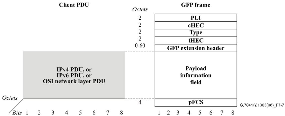
**Figure 7-7 – IPv4/IPv6/OSI network layer PDUs and GFP frame relationships**
