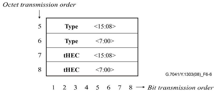
**Figure 6-6 – Payload header for a GFP frame with a null extension header**
