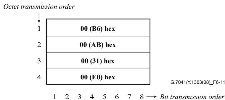
**Figure 6-11 – GFP idle frame (Barker-like scrambled frame)**
