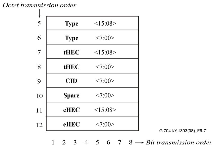
**Figure 6-7 – Payload header for a linear (point-to-point) frame including the extension header**
