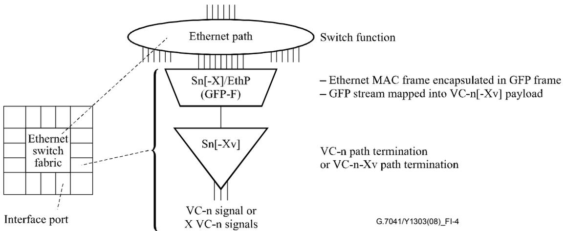
**Figure I.4 – VC-n-Xv port on Ethernet switch or Ethernet switch function embedded in hybrid SDH/Ethernet equipment**
