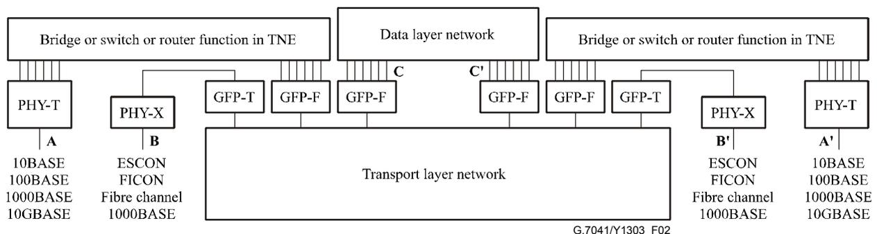
**Figure 2 – GFP functional model (single client)**
