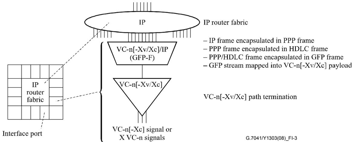
**Figure I.3 – VC-n/VC-n-Xv/VC-n-Xc port on IP router or IP router function embedded in hybrid SDH/IP equipment**
