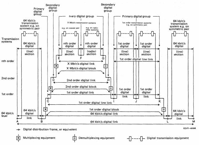
Note 1 — Digital line and radio sections may be at digit rates which are either hierarchical or non-hierarchical.
