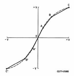
$\label{eq:bound} \textit{Note } - \text{This particular characteristic has 5 linear segments: } C'B', B'A', A'A, AB, BC.$
