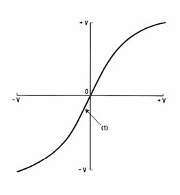
Note - A central linear section (1), if present, must tangentially join on to the curved end-section.
