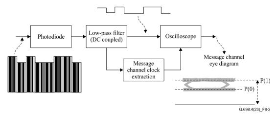
Figure 8-2 – Measurement set-up for the modulation depth of the message channel
