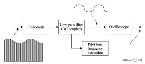
Figure 8-3 – Measurement set-up for the modulation depth of pilot tone
