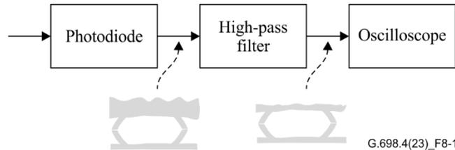
**Figure 8-1 – Measurement set-up for the eye mask**
