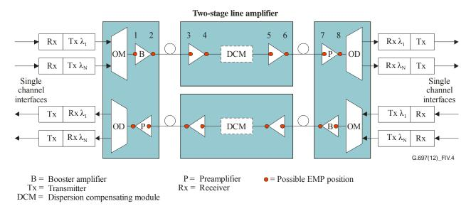
Figure IV.4 – Example of EMP positioning inside a long-distance DWDM line segment
