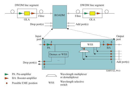
Figure IV.3 – Example of EME positioning inside a ROADM
