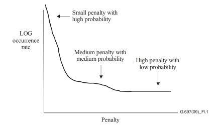
Figure I.1 – Example curve of penalty versus occurrence rate due to attenuation variation
