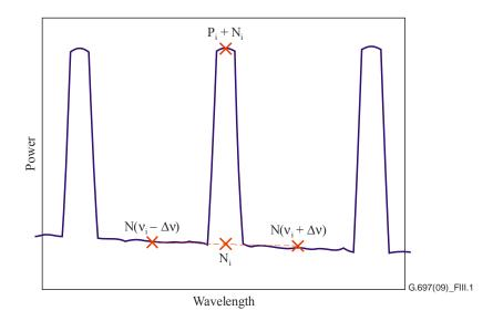
Figure III.1 – OSNR measurement method
