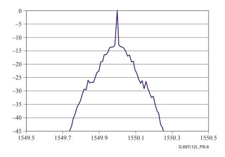
Figure III.6 – Optical spectrum where signal occupies full channel bandwidth
