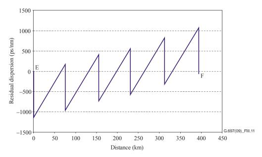
Figure III.11 - Residual dispersion versus distance for a more complex system
