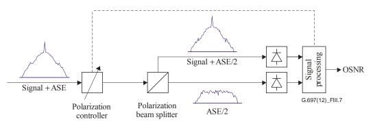
Figure III.7 – Polarization extinction method block diagram
