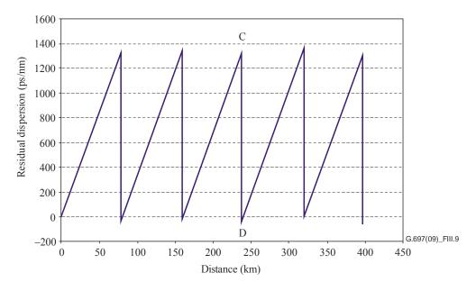
Figure III.9 – Residual dispersion versus distance for a simple system
