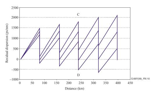
Figure III.10 – Residual dispersion versus distance for a simple system with a wide wavelength range
