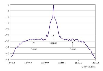
Figure III.5 – Optical spectrum where signal does not occupy full channel bandwidth
