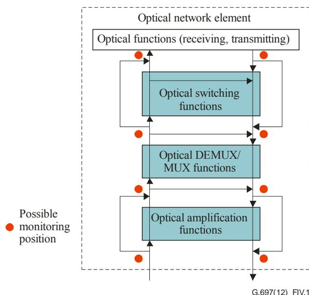
Figure IV.1 – Example of EME positioning inside an optical network element
