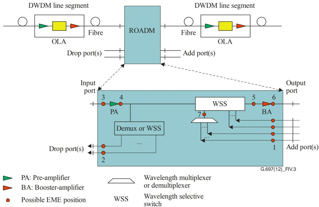
**Figure IV.3 – Example of EME positioning inside a ROADMs**
