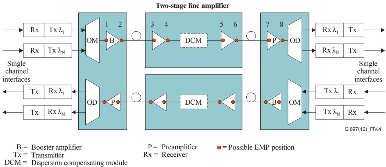
**Figure IV.4 – Example of EMP positioning inside a long-distance DWDM line segment**
