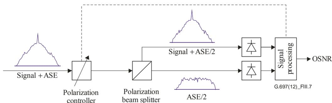
**Figure III.7 – Polarization extinction method block diagram**
