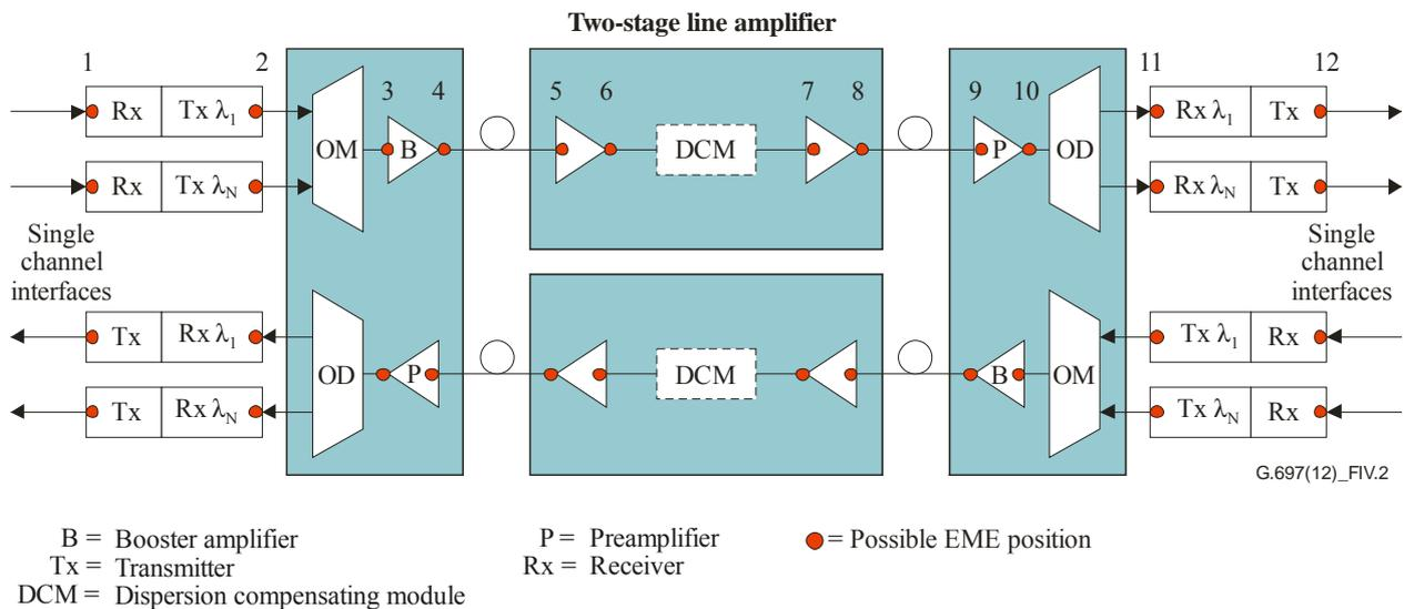
**Figure IV.2 – Example of EME positioning inside a long-distance DWDM line segment**
