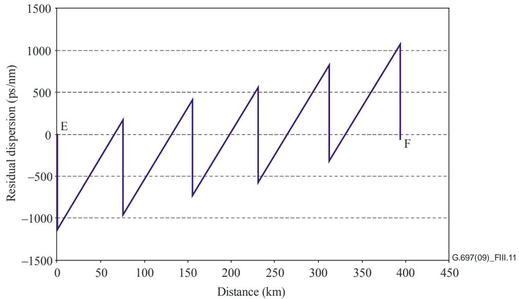
**Figure III.11 – Residual dispersion versus distance for a more complex system**
