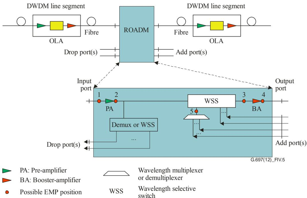
**Figure IV.5 – Example of EMP positioning inside an example ROADM**
