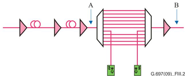
**Figure III.2 – Section of a DWDM system with an OADM**
