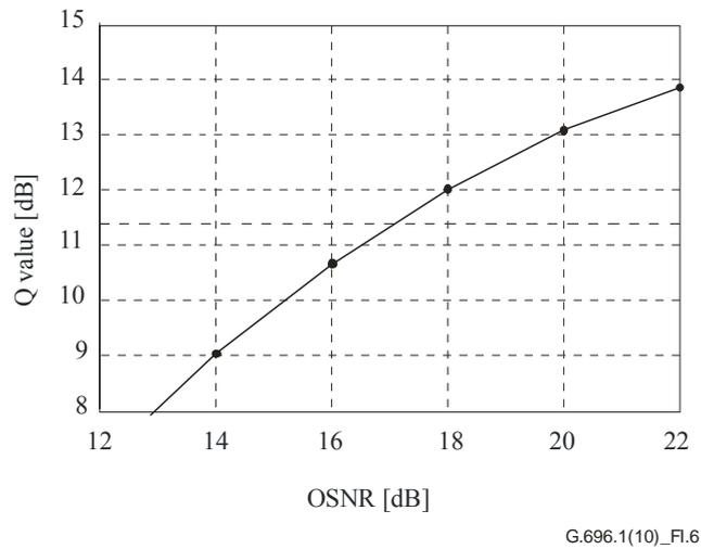
**Figure I.6 – Example of the Q value versus OSNR for 112 Gbit/s DP-QPSK signal**
