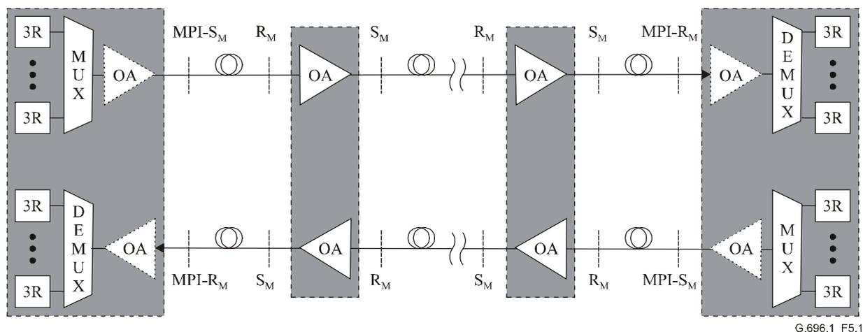
Figure 5-1 – Reference configuration for a multi-span DWDM system
