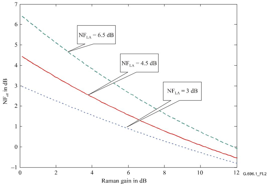
**Figure I.2 –  $NF_{\text{eff}}$  as a function of Raman gain**
