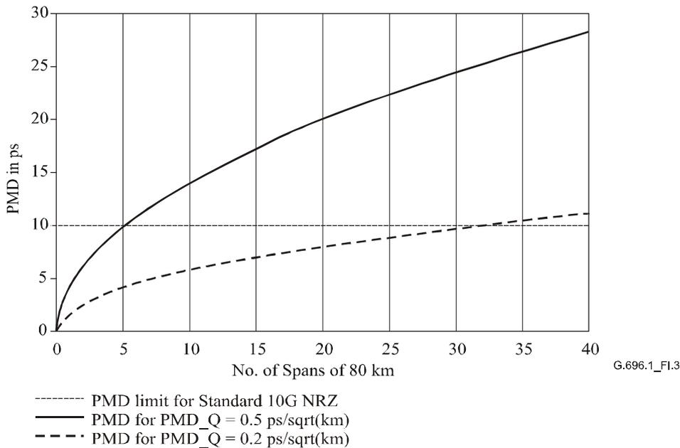
**Figure I.3 – PMD vs distance for different PMD coefficients and PMD limit for 10 Gbit/s NRZ systems with 99.999% availability**
