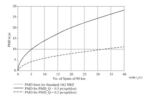
Figure I.3/G.696.1 – PMD vs distance for different PMD coefficients and PMD limit for 10 Gbit/s NRZ systems with 99.999% availability
