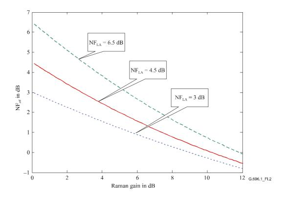
Figure I.2/G.696.1 – NF<sub>eff</sub> as a function of Raman gain
