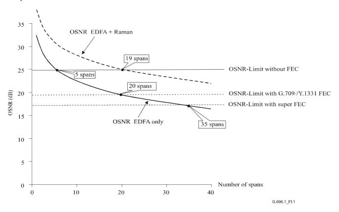
Figure I.1/G.696.1 – OSNR limits for a reference system, OSNR as a function of span number with and without Raman amplification
