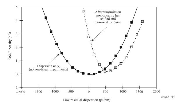
Figure I.4/G.696.1 – Example of the effect of non-linearity on dispersion tolerance after transmission
