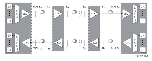
Figure 5-1/G.696.1 – Reference configuration for a multi-span DWDM system
