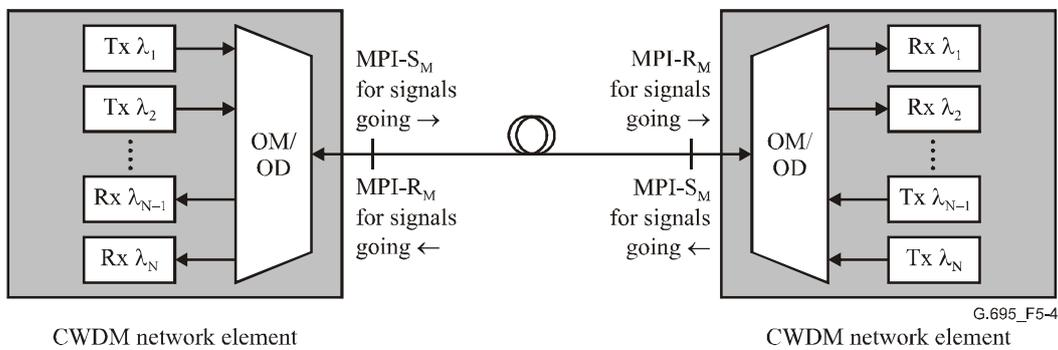
**Figure 5-4 – "Black box" approach for bidirectional applications**
