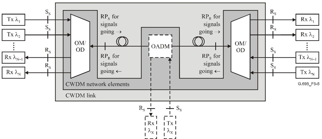
**Figure 5-5 – Linear "black link" approach for bidirectional applications**
