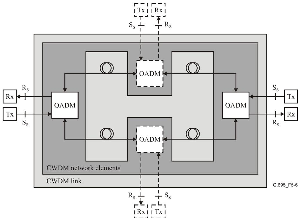
**Figure 5-6 – Ring "black link" approach for bidirectional applications**
