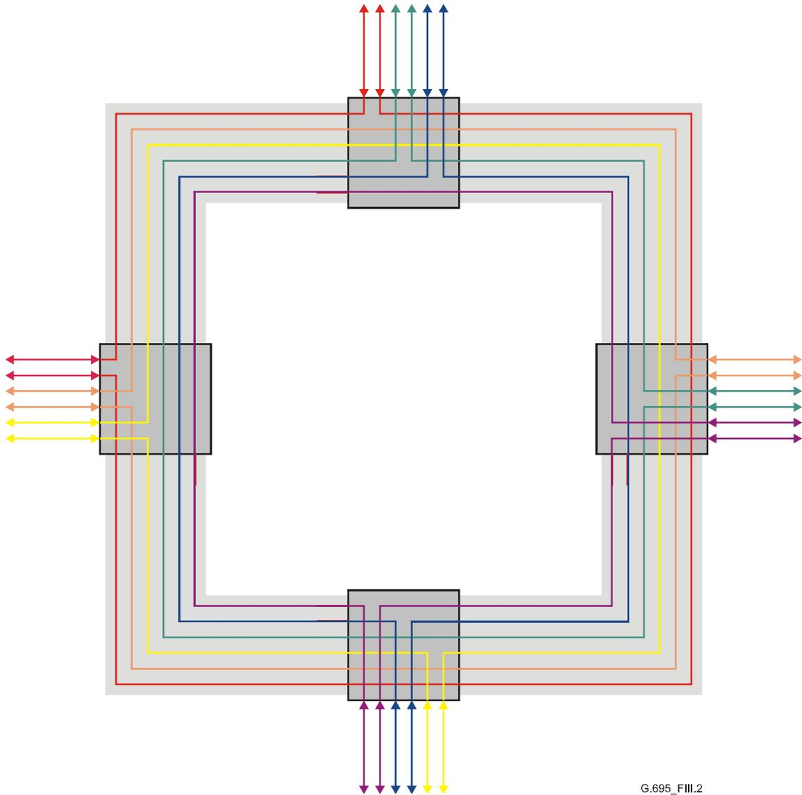
**Figure III.2 – Complex example of ring black-link topology**
