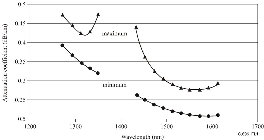
**Figure I.1 – Assumed attenuation coefficient values for G.652.A&B cable**
