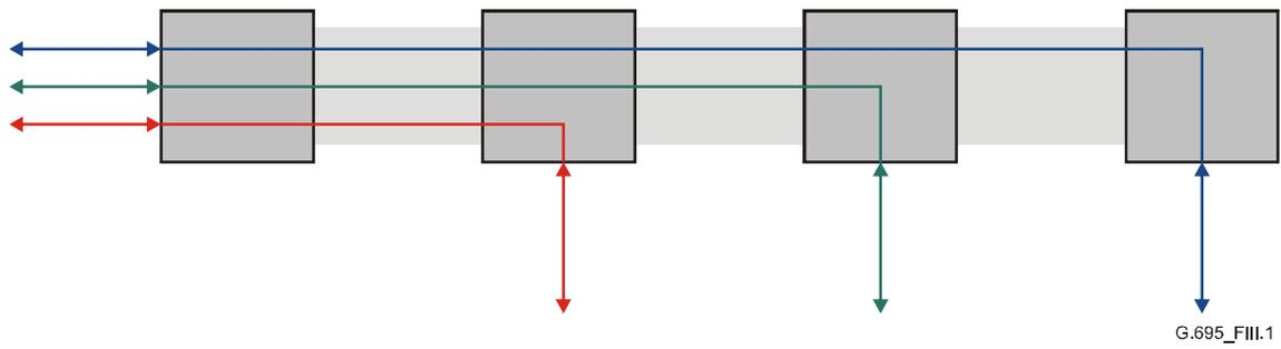
**Figure III.1 – Simple example of linear black-link topology**
