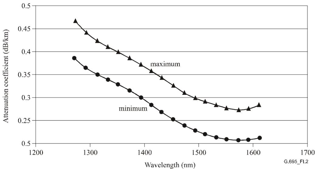
**Figure I.2 – Assumed attenuation coefficient values for G.652.C&D cable**
