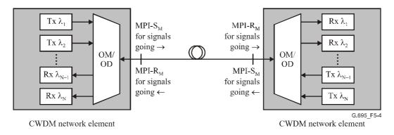
Figure 5-4 – "Black box" approach for bidirectional applications
