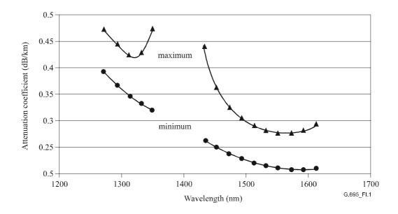
Figure I.1 – Assumed attenuation coefficient values for G.652.A&B cable
