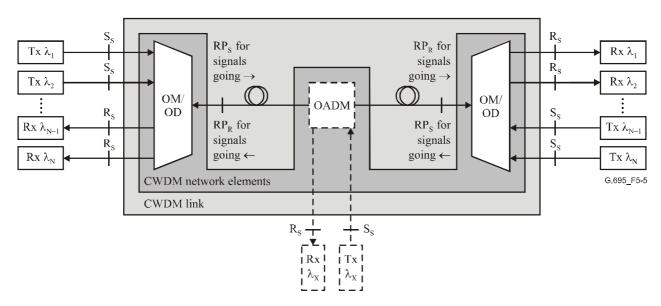
Figure 5-5 – Linear "black-link" approach for bidirectional applications
