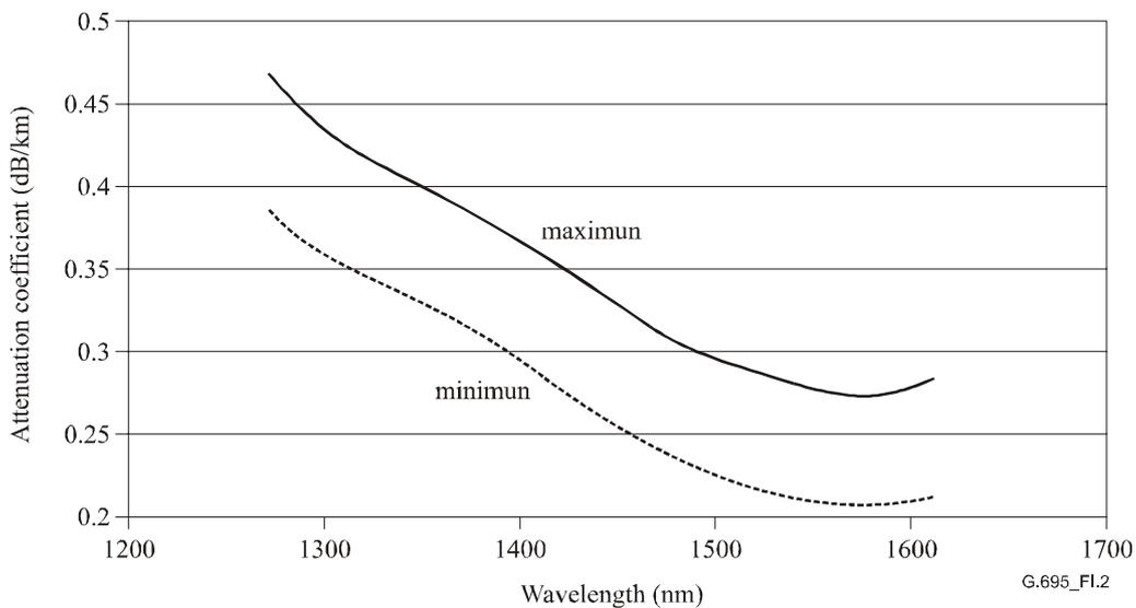
**Figure I.2/G.695 – Assumed attenuation coefficient values for G.652.C&D cable**
