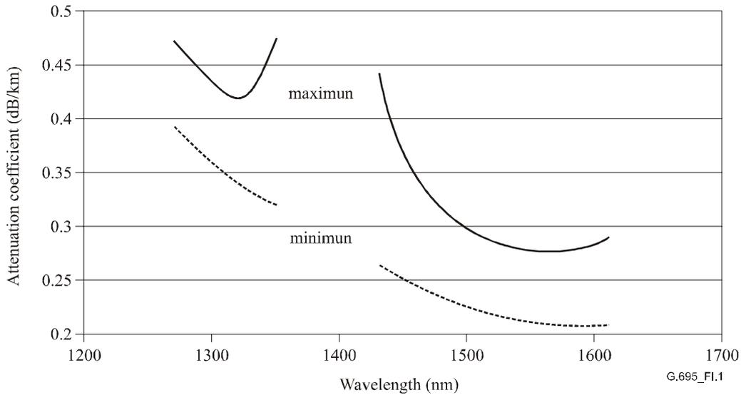
**Figure I.1/G.695 – Assumed attenuation coefficient values for G.652.A&B cable**
