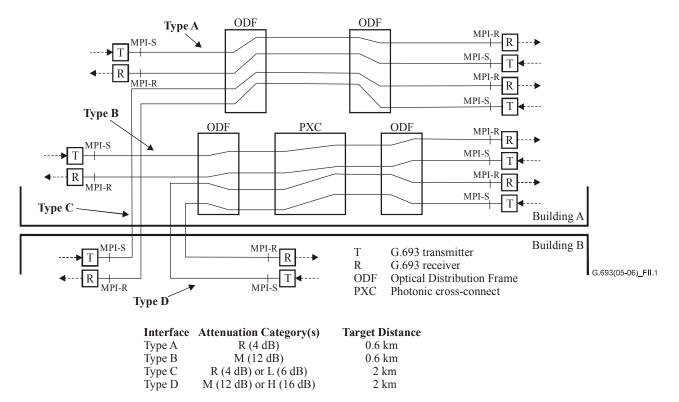
Figure II.1 – Examples of system configurations using applications defined in this Recommendation
