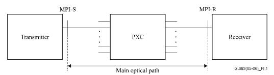
Figure I.1 – Optical link example showing use of a passive photonic cross-connect (PXC) between MPI-S and MPI-R
