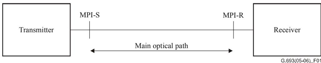
NOTE – The main optical path includes fibre and connectors, and may include other passive optical devices such as photonic cross-connects.
