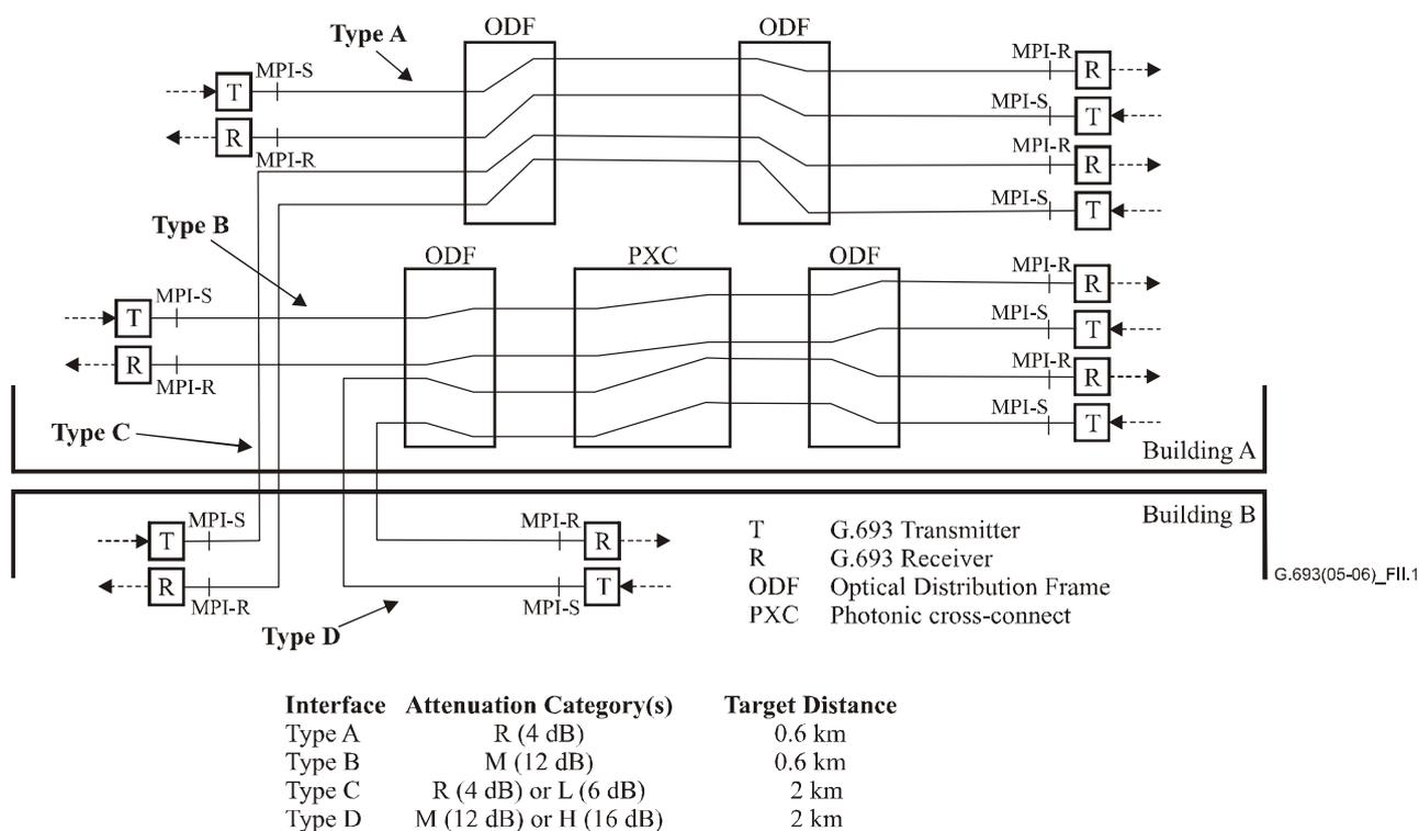
**Figure II.1/G.693 – Examples of system configurations using applications defined in this Recommendation**
