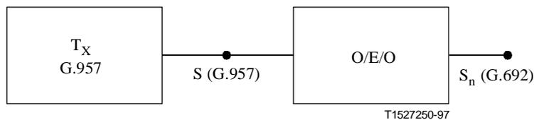
**Figure 2/G.692 – Possible implementation of a G.692 transmitter using a G.957 compliant transmitter and a transponder**
