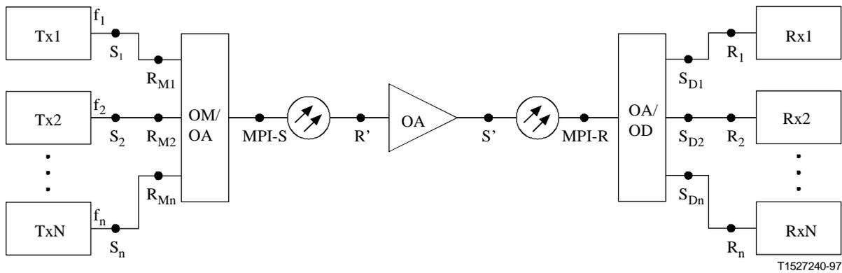
**Figure 1/G.692 – Representation of optical line system interfaces**
