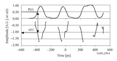
Figure IV.4/G.691 – Plot of the calculated values for P(t) and  $\alpha$ (t); The arrows show how to find the chirp parameter
