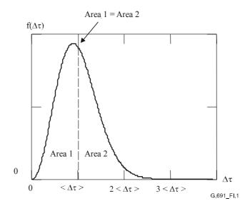
Figure I.1/G.691 – The Maxwell distribution function (illustration) – Probability density function  $f(\Delta \tau)$  vs differential group delay,  $\Delta \tau$
