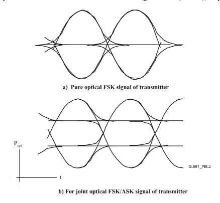
Figure III.2/G.691 – Receiver eye diagrams after dispersive fibre
