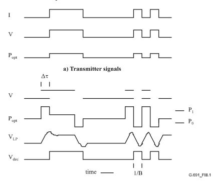
b) Receiver signals after dispersive fibre of length L
