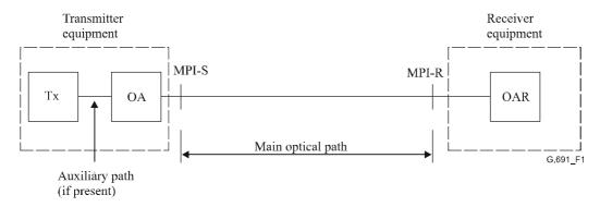
Figure 1/G.691 – An example of an optical link showing the interface points defined in this Recommendation
