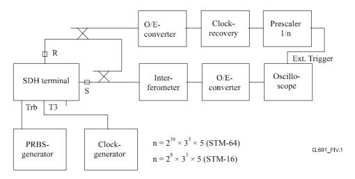
Figure IV.1/G.691 – Measurement set-up
