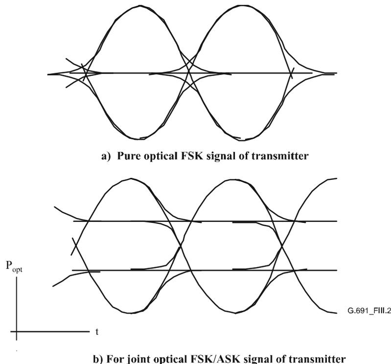
Figure III.2/G.691 – Receiver eye diagrams after dispersive fibre
