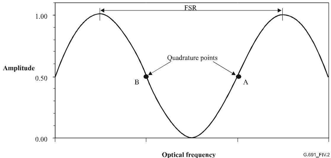
**Figure IV.2/G.691 – Sketch of the transfer function of the two-beam interferometer showing the quadrature points A and B and defining the free spectral range**
