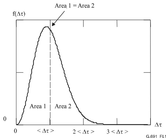
**Figure I.1/G.691 – The Maxwell distribution function (illustration) – Probability density function  $f(\Delta\tau)$  vs differential group delay,  $\Delta\tau$**
