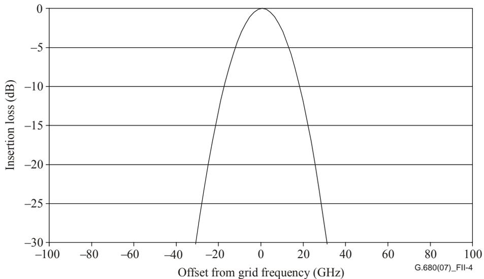
**Figure II.4 – Resulting filter function of eight concatenated Gaussian filters**
