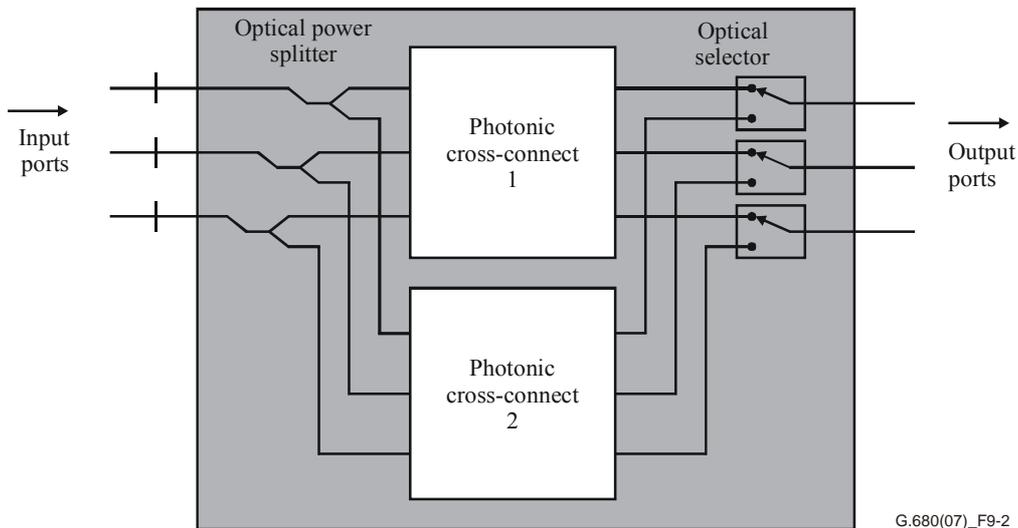
**Figure 9-2 – Photonic cross-connect (PXC) with redundancy**
