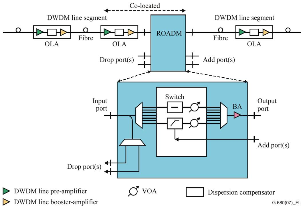
**Figure I.2 – Configuration of Example 3 – ROADMs with amplifiers**
