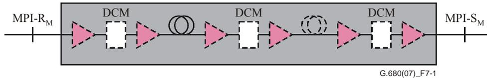
Figure 7-1 – DWDM line segment reference diagram
