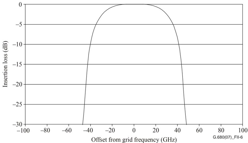
**Figure II.6 – Resulting filter function of eight concatenated flat-topped filters**
