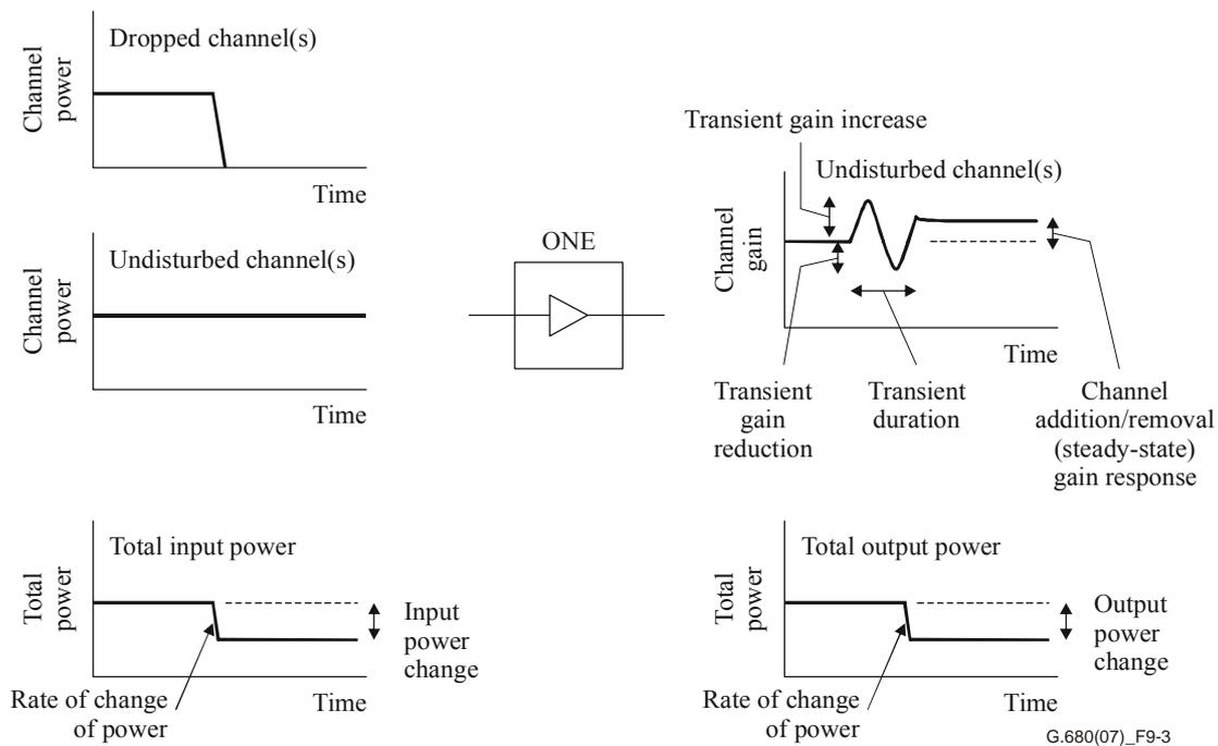
**Figure 9-3 – Illustration of optical transients in a single ONE**
