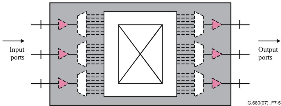
**Figure 7-5 – Photonic cross-connect (PXC) reference diagram including amplifiers**
