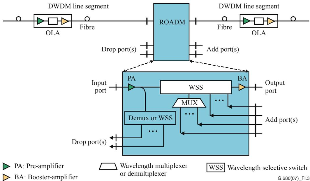
**Figure I.3 – Configuration of Example 4 – ROADM with amplifiers**
