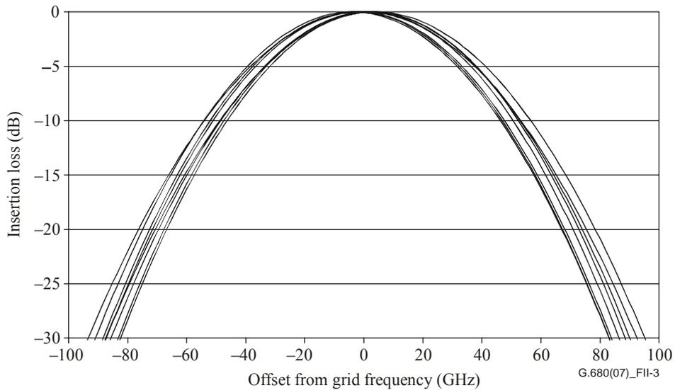
**Figure II.3 – Superimposed filter shapes of eight Gaussian filters**
