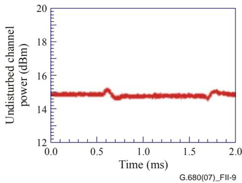
**Figure II.9 – Output power of undisturbed channel with gain control on**
