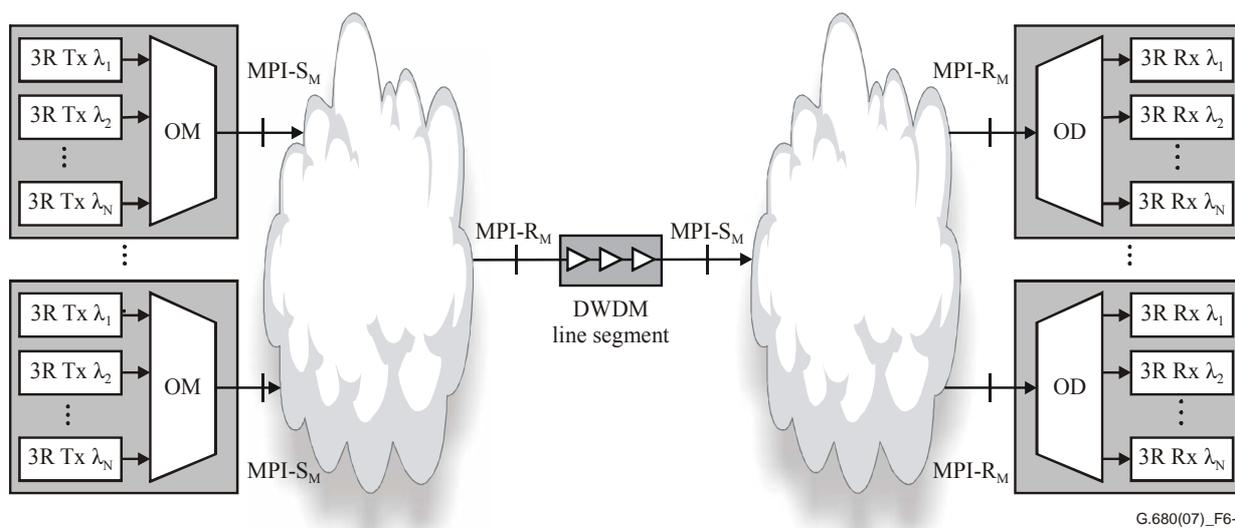
**Figure 6-1 – DWDM line segment reference points**
