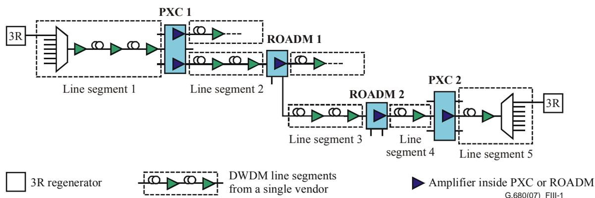
Figure III.1 – Example optical transmission system
