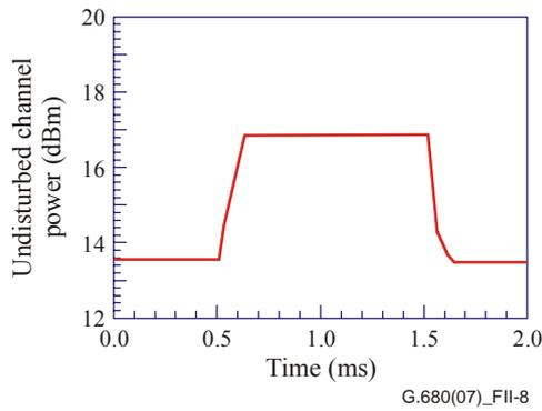
**Figure II.8 – Output power of undisturbed channel with gain control off (constant pump power)**
