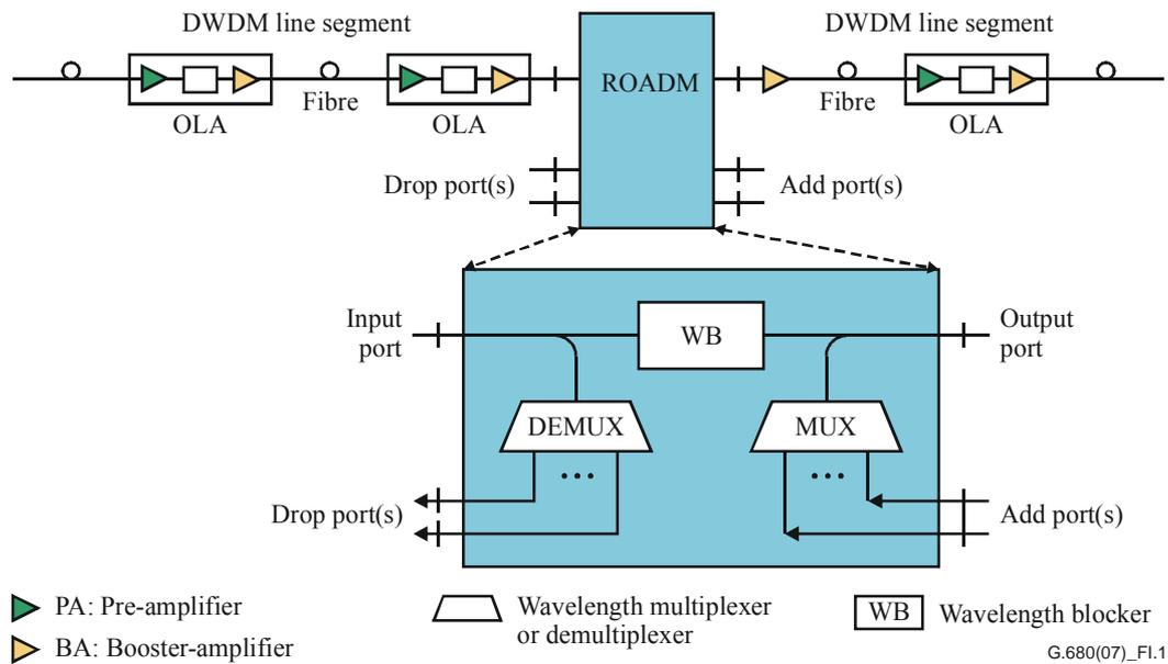
**Figure I.1 – Configuration of Example 2 – ROADM without amplifiers**
