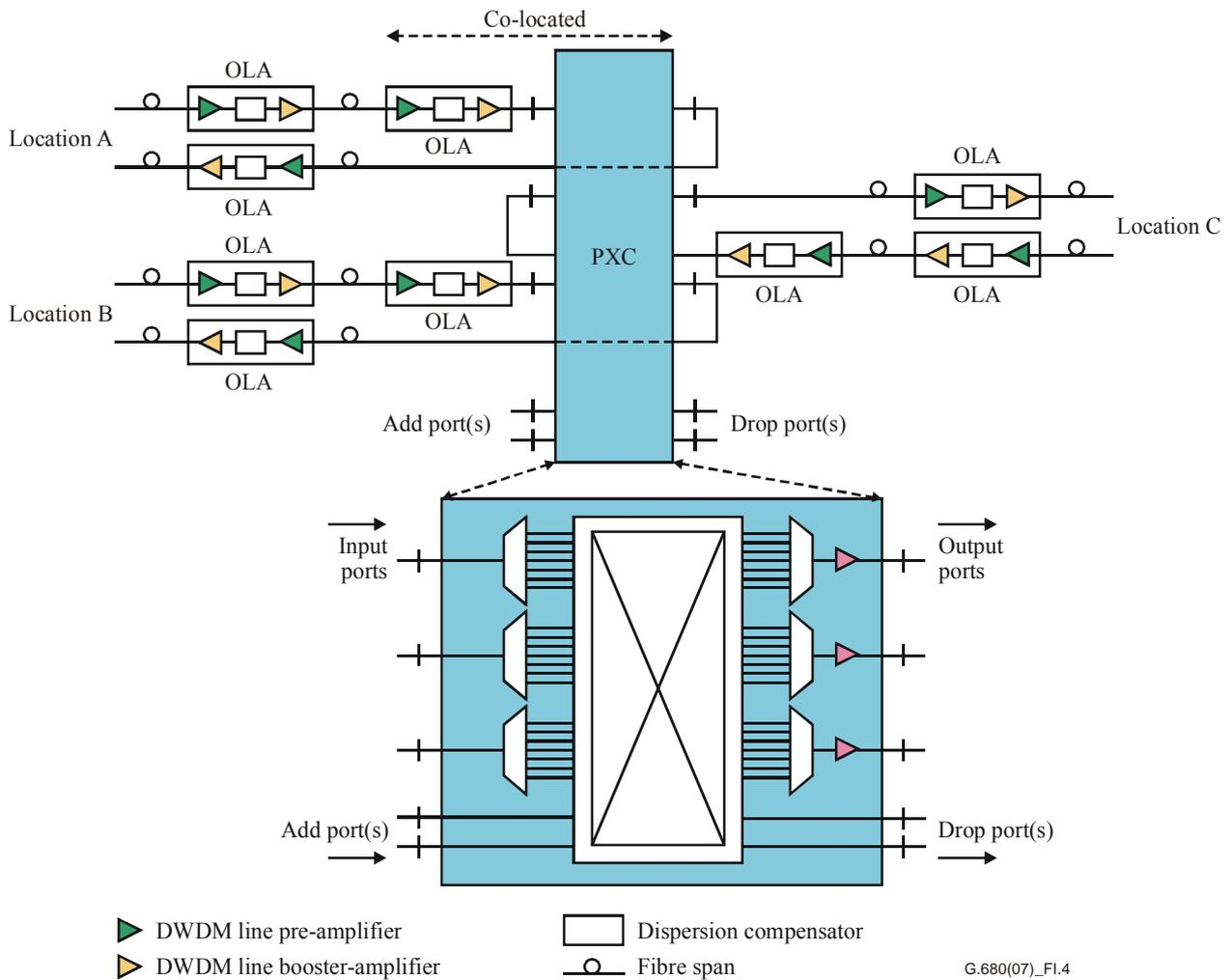
**Figure I.4 – Configuration of Example 5 – PXC with amplifiers**
