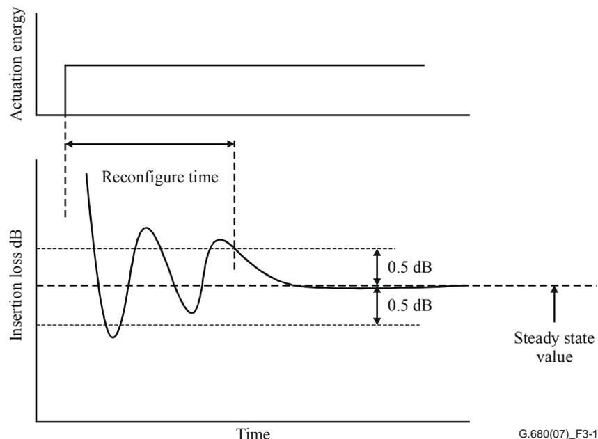
**Figure 3-1 – Illustration of reconfigure time**
