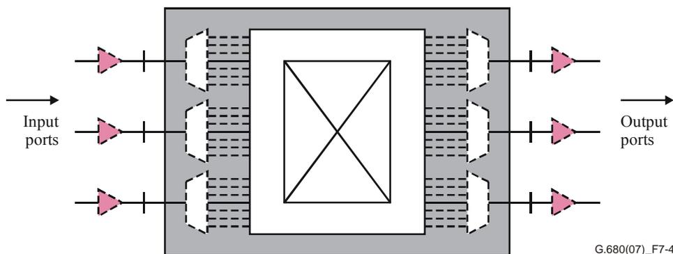
**Figure 7-4 – Photonic cross-connect (PXC) reference diagram without amplifiers**
