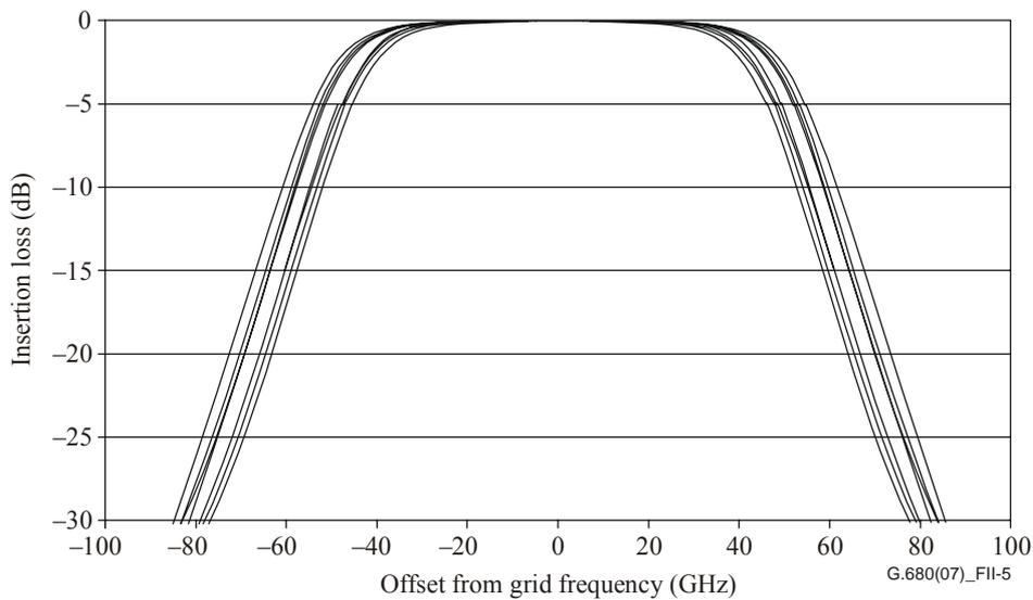
**Figure II.5 – Superimposed filter shapes of eight flat-topped filters**
