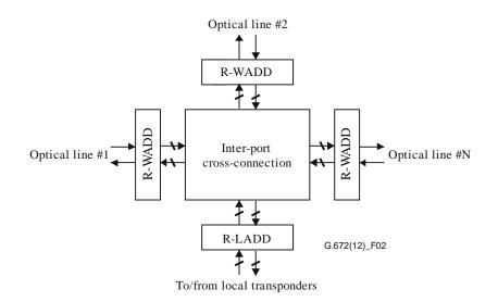
Figure 2 – MD-ROADM reference diagram
