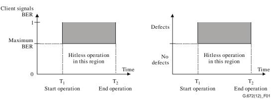
**Figure 1 – Illustration of hitless operation conditions**
