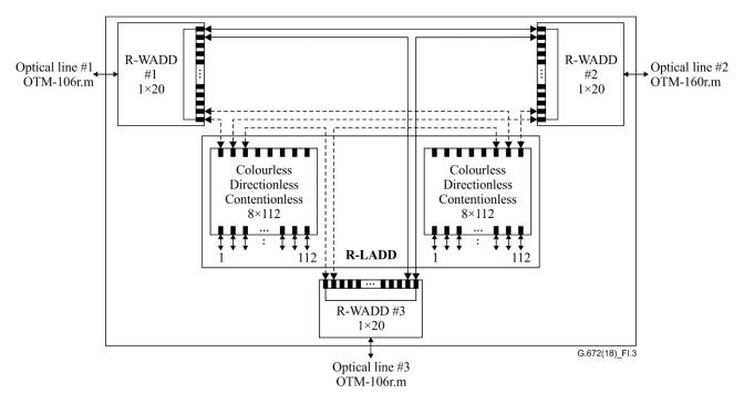
Figure I.3 – MD-ROADM scheme for example 3
