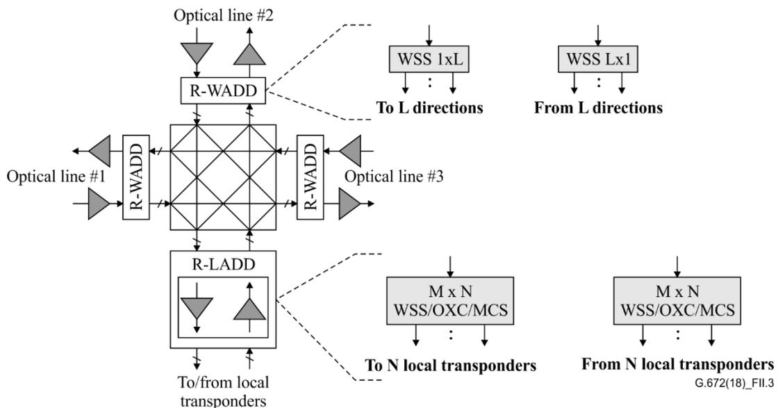
**Figure II.3 – Configuration of an MD-ROADM with the colourless, directionless, contentionless (and flexible grid) feature**
