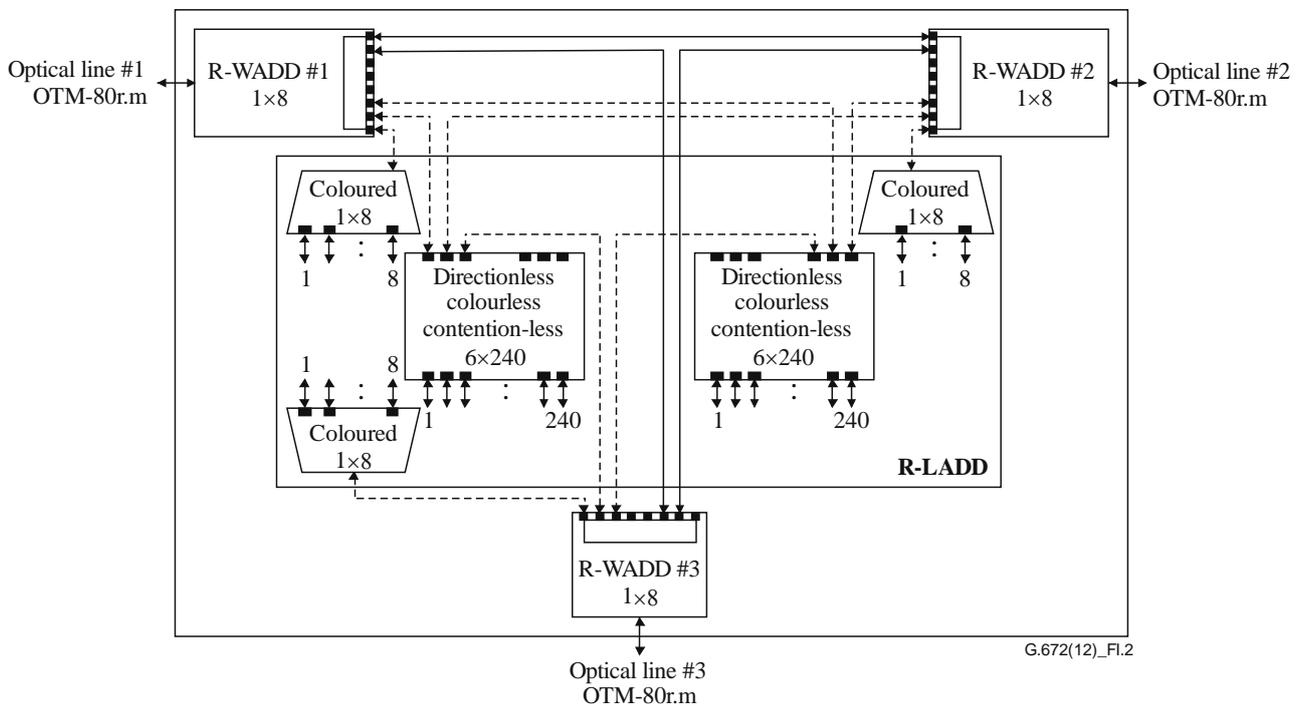
**Figure I.2 – MD-ROADM scheme for example 2**
