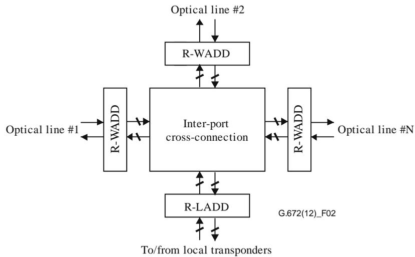
**Figure 2 – MD-ROADM reference diagram**
