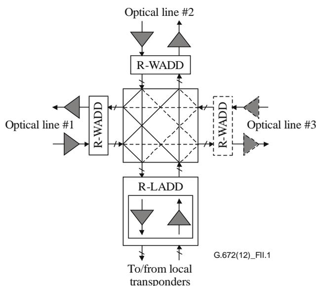
Figure II.1 – Configuration of the direction/degree expansion example
