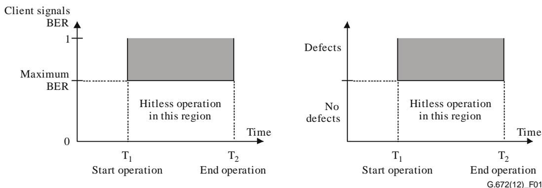
**Figure 1 – Illustration of hitless operation conditions**
