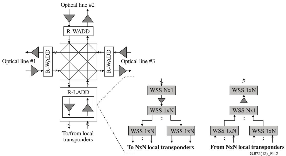
**Figure II.2 – Configuration of an MD-ROADM with the directionless and colourless feature**
