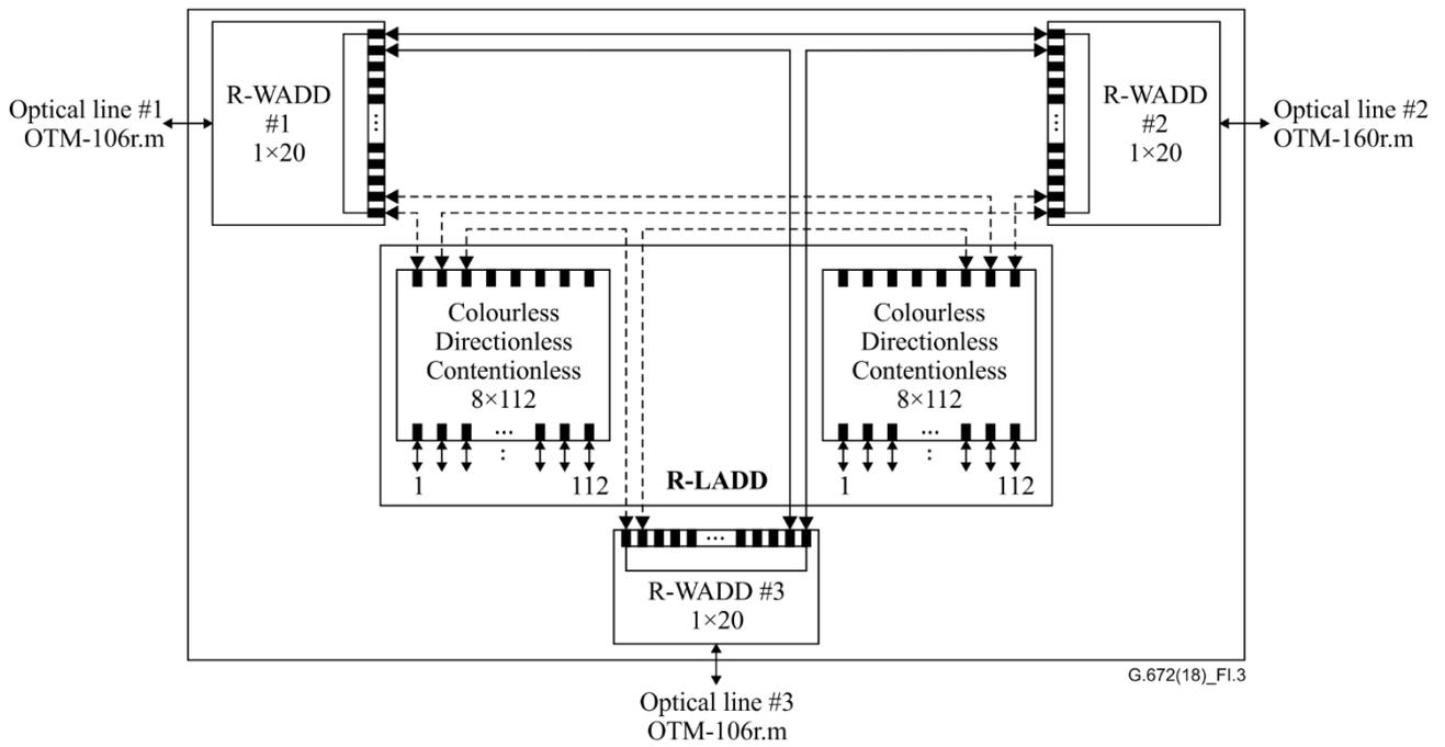
**Figure I.3 – MD-ROADM scheme for example 3**
