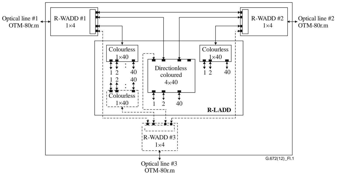
Figure I.1 – MD-ROADM scheme for example 1
