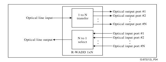
Figure 4 – R-WADD 1xN reference diagram
