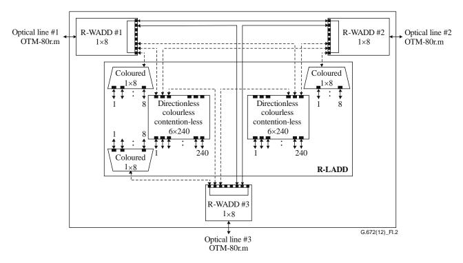
Figure I.2 – MD-ROADM scheme for Example 2
