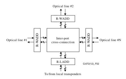
Figure 2 – MD-ROADM reference diagram
