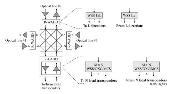
Figure II.3 – Configuration of an MD-ROADM with the colourless, directionless, contentionless (and flexible grid) feature
