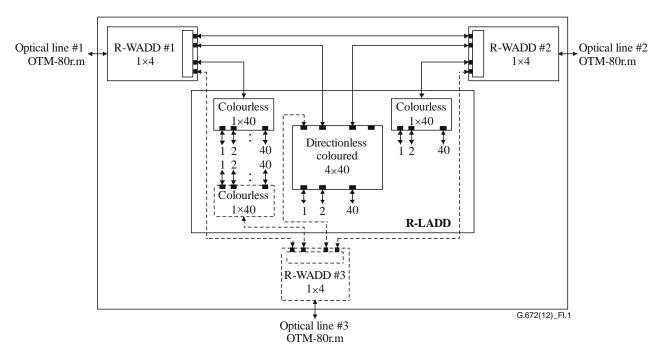
Figure I.1 – MD-ROADM scheme for example 1
