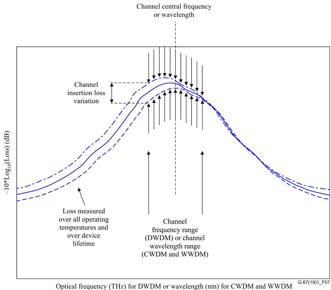
**Figure 7 – Illustration of channel insertion loss variation of a WDM device**
