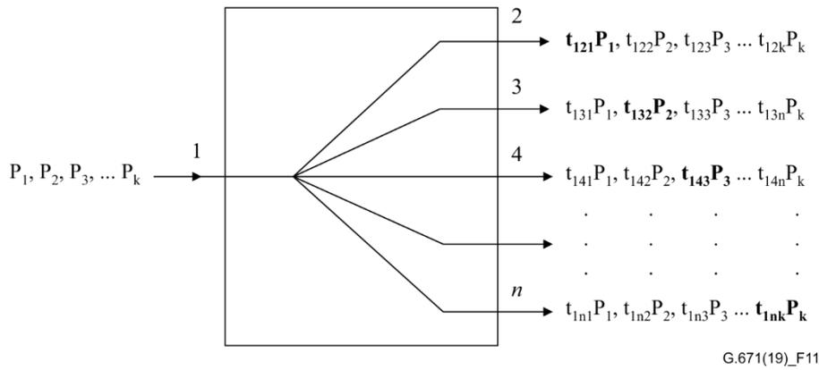
**Figure 11 – Example of WDM demultiplexer device**
