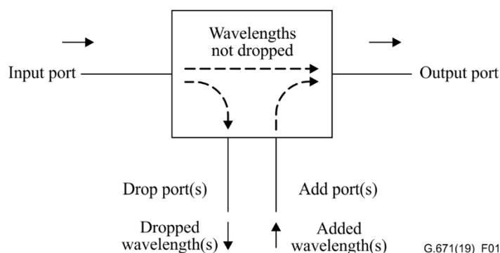
**Figure 1 – Optical add/drop multiplexer (OADM) subsystem**
