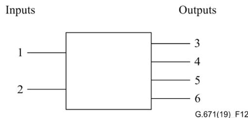
**Figure 12 – An example of the port assignments for the transfer matrix**
