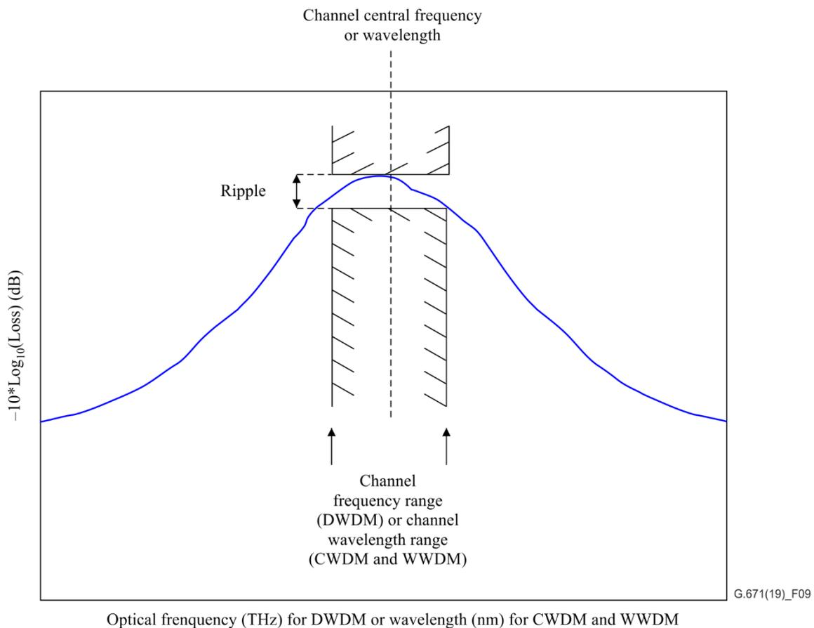
**Figure 9 – Illustration of ripple for a WDM device**
