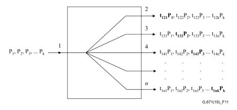
Figure 11 – Example of WDM demultiplexer device
