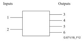
Figure 12 – An example of the port assignments for the transfer matrix
