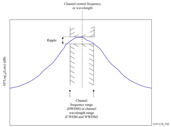
Optical frenquency (THz) for DWDM or wavelength (nm) for CWDM and WWDM
