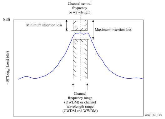
Optical frequency (THz) for DWDM or wavelength (nm) for CWDM and WWDM
