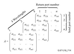
Figure 14 – Logarithmic transfer matrix
