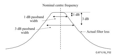
Figure 2 – Illustration of 1 dB and 3 dB passband width
