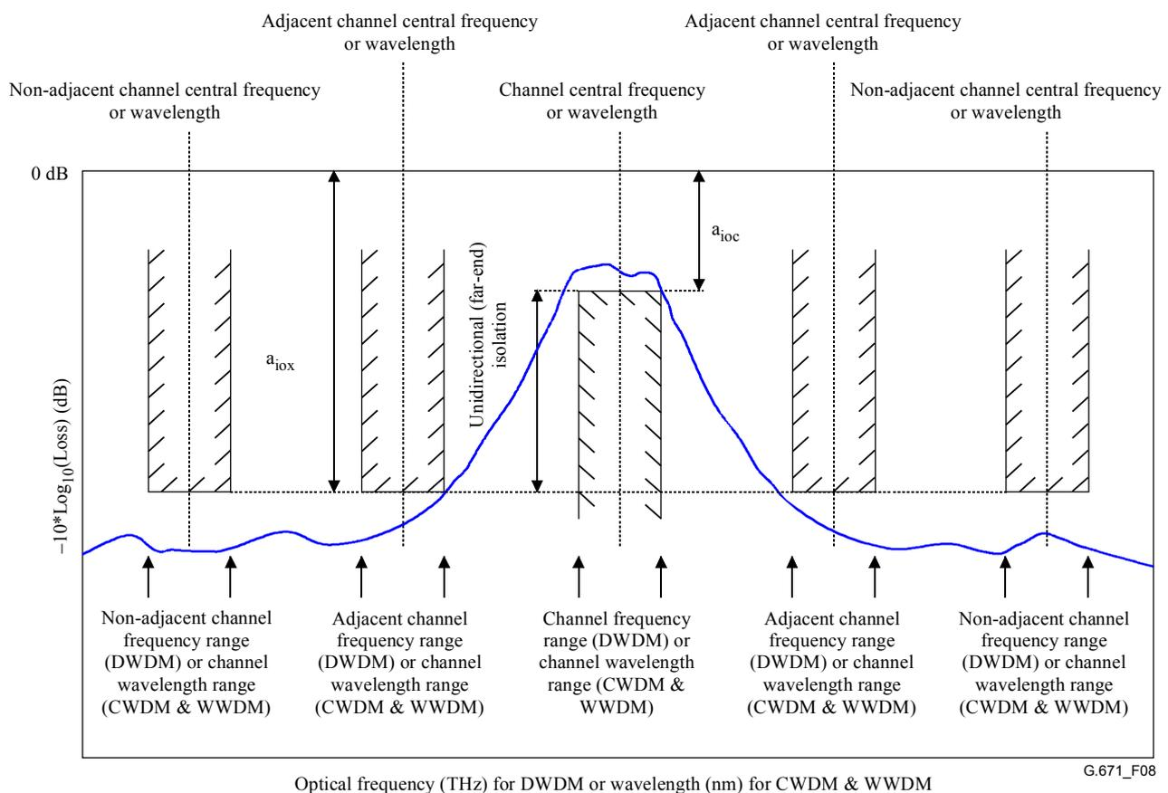
**Figure 8/G.671 – Illustration of unidirectional (far-end) isolation of a WDM device**
