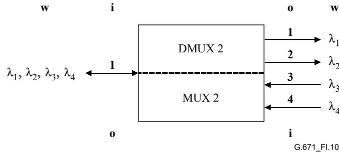
**Figure I.10/G.671 – 4λ-DMUX/MUX2 port numbering**
