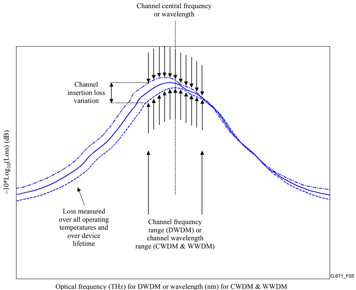
**Figure 5/G.671 – Illustration of channel insertion loss variation of a WDM device**
