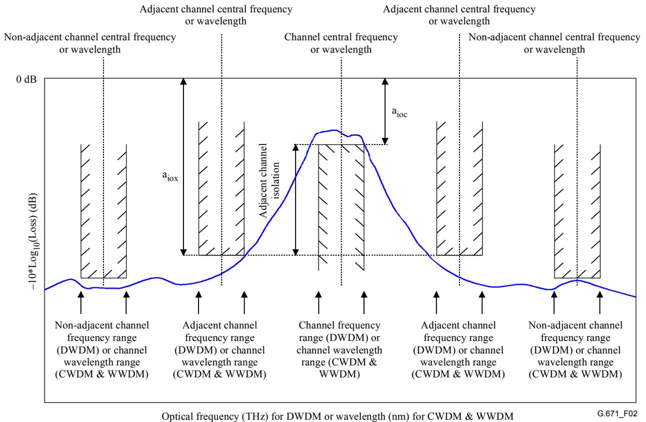
**Figure 2/G.671 – Illustration of adjacent channel isolation for a WDM device**
