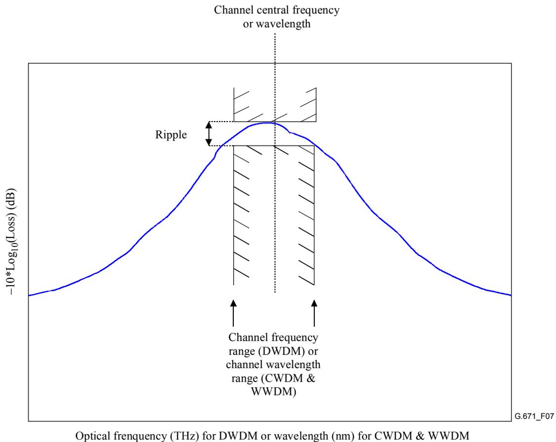
**Figure 7/G.671 – Illustration of ripple for a WDM device**
