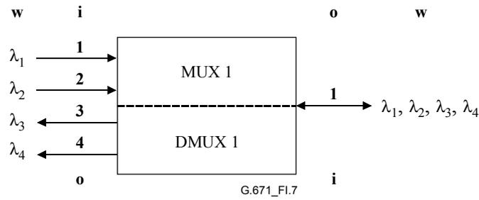
**Figure I.7/G.671 – 4λ-MUX/DMUX1 port numbering**
