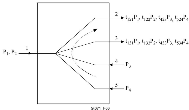
**Figure 3/G.671 – Example of bidirectional (near-end) isolation**
