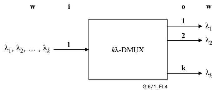
Figure I.4/G.671 –  $k\lambda$ -DMUX port numbering
