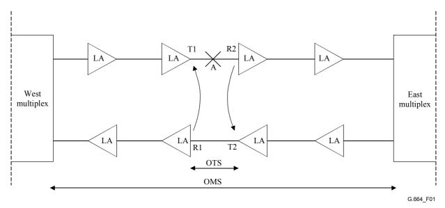
Figure 1/G.664 – Description of APR capability in the case of cable break
