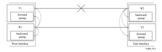
Figure II.2/G.664 – Possible actions in the case of a cable break
