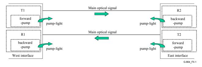
Figure II.1/G.664 – Configuration with forward and backward pump lasers in a section within multi-span transmission system employing distributed Raman amplification
