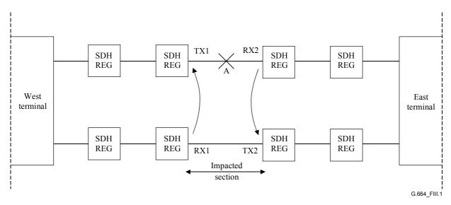
Figure III.1/G.664 – Clarification of ALS operation in the case of a cable break in a chain of SDH regenerators
