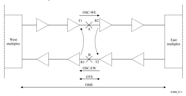
Figure I.1/G.664 – Description of APR capability in the case of cable break in a configuration with co-propagating OSC
