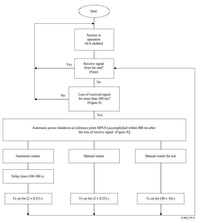
NOTE – "Receive signal from far end?" is also active when the transmitter is in the shutdown situation.
