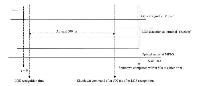
Figure III.4/G.664 – Clarification of shutdown timing requirements
