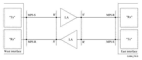
Figure III.5/G.664 – Reference configuration for description of ALS capability in the case that line amplifiers are present
