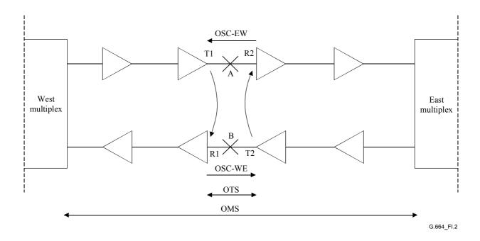
Figure I.2/G.664 – Description of APR capability in the case of cable break in a configuration with counter-propagating OSC
