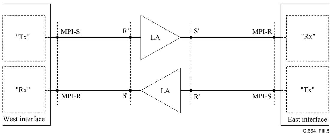
**Figure III.5/G.664 – Reference configuration for description of ALS capability in the case that line amplifiers are present**
