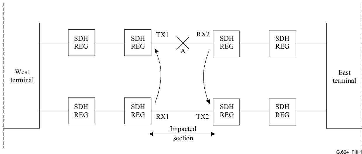
**Figure III.1/G.664 – Clarification of ALS operation in the case of a cable break in a chain of SDH regenerators**
