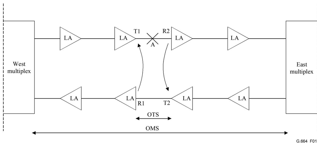
**Figure 1/G.664 – Description of APR capability in the case of cable break**
