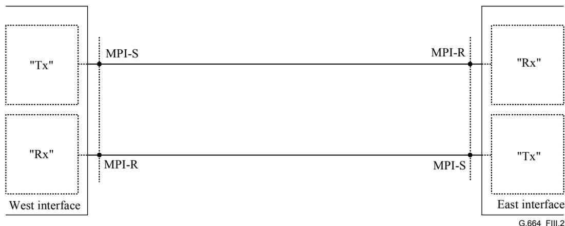
**Figure III.2/G.664 – Reference configuration for description of ALS capability**
