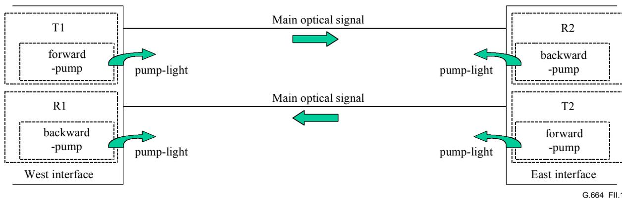
**Figure II.1/G.664 – Configuration with forward and backward pump lasers in a section within multi-span transmission system employing distributed Raman amplification**
