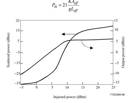
Figure II.3-6 – Stimulated Brillouin scattering effect for narrow-band source
