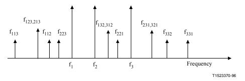
Figure II.3-4 – Mixing products generated due to four-wave mixing of three signals
