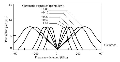
Figure II.3-3 – Calculated MI gain versus frequency detuning, from 30 km-long fibres (0.24 dB/km loss) with five different dispersion coefficient values, for +16 dBm CW signal launched power
