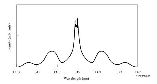
Figure II.3-2 – Power spectrum of a pulse after propagation in 1 km-long fibre (input pulse width: 100 ps, peak power: 7 W). Spectral side lobes appeared due to MI
