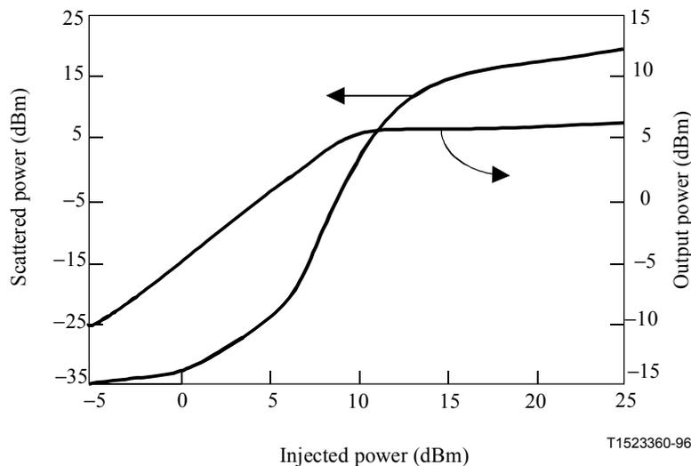
**Figure II.3-6/G.663 – Stimulated Brillouin scattering effect for narrow-band source**
