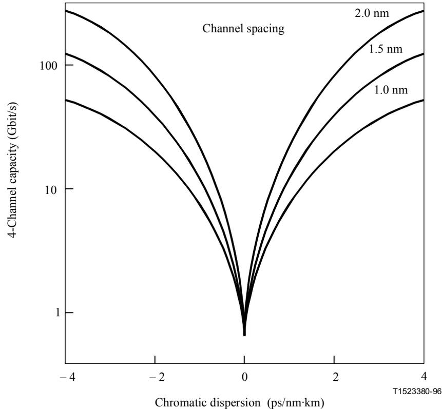
**Figure II.3-5/G.663 – Impact of dispersion on system capacity in the presence of FWM**
