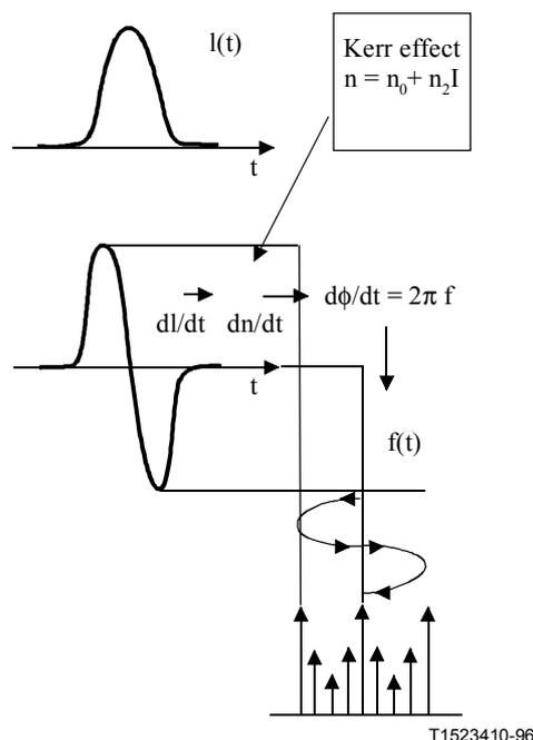
**Figure II.3-1/G.663 – Spectral broadening mechanism due to self phase modulation**
