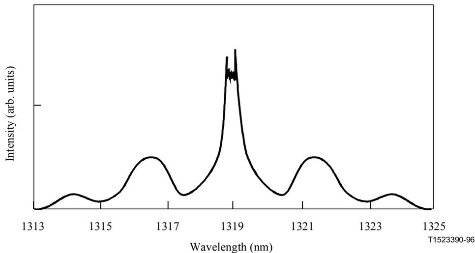
**Figure II.3-2/G.663 – Power spectrum of a pulse after propagation in 1 km-long fibre (input pulse width: 100 ps, peak power: 7 W). Spectralside lobes appeared due to MI**
