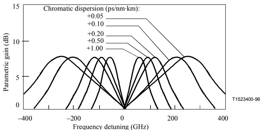
**Figure II.3-3/G.663 – Calculated MI gain versus frequency detuning, from 30 km long fibres (0.24 dB/km loss) with five different dispersion coefficient values, for +16 dBm CW signal launched power**
