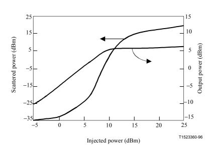
Figure II.3-6/G.663 – Stimulated Brillouin scattering effect for narrow-band source
