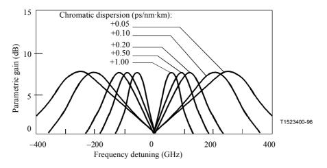
Figure II.3-3/G.663 – Calculated MI gain versus frequency detuning, from 30 km long fibres (0.24 dB/km loss) with five different dispersion coefficient values, for +16 dBm CW signal launched power
