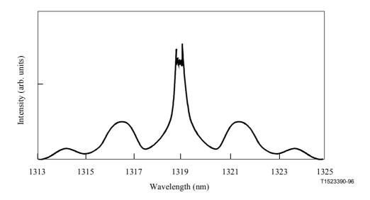
Figure II.3-2/G.663 – Power spectrum of a pulse after propagation in 1 km-long fibre (input pulse width: 100 ps, peak power: 7 W). Spectralside lobes appeared due to MI
