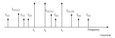
Figure II.3-4/G.663 – Mixing products generated due to four-wave mixing of three signals
