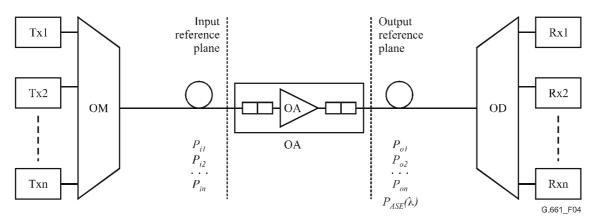
Figure 4/G.661 – An optical amplifier in a multichannel application
