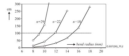
Figure I.2 – Maximum storage length for a bent fibre and different values of the fatigue parameter n
