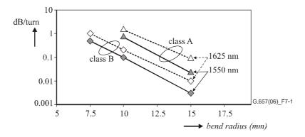
Figure 7-1 – Macrobending loss data from Tables 7-1 and 7-2, class A and B
