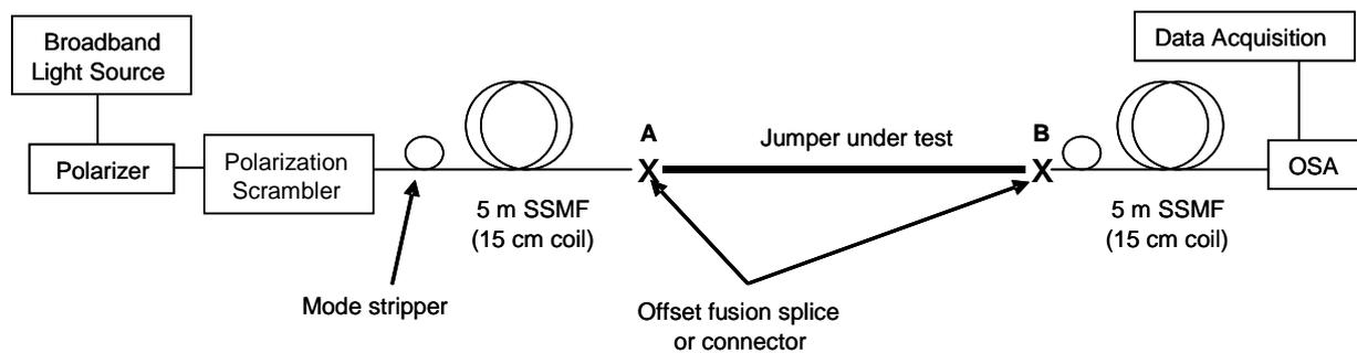
**Figure IV.2 – Schematic of set-up for the wideband LED/OSA method. The polarizer is not necessary if the broadband light source has an internal polarizer**
