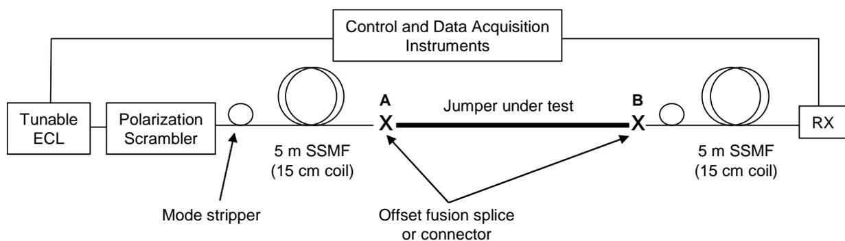
**Figure IV.1 – Schematic of set-up for narrowband ECL/PM method.**
