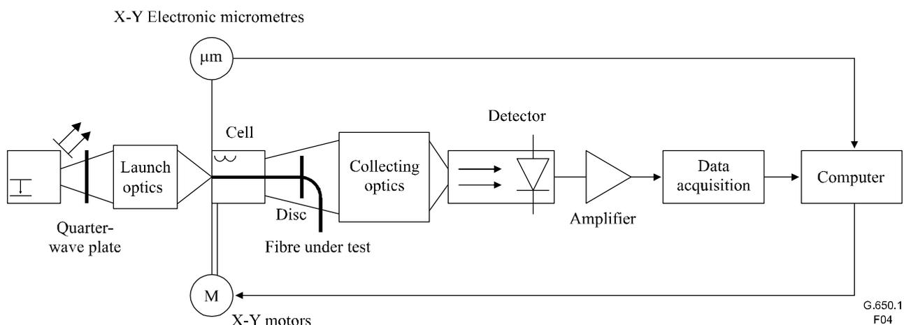
Figure 4/G.650.1 – Typical arrangement of the refracted near-field test set-up
