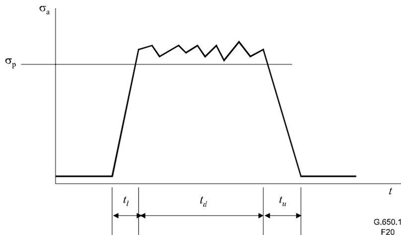
Figure 20/G.650.1 – Stress  $\sigma$  versus time  $t$  during proofstesting
