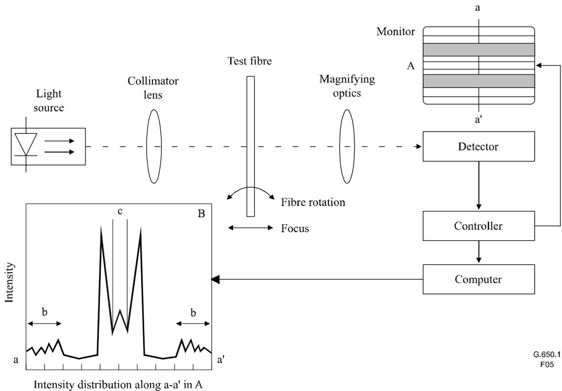
**Figure 5/G.650.1 – Schematic diagram of side-view measurement system**
