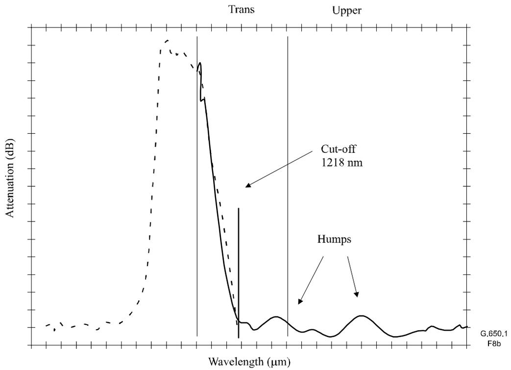
**Figure 8b/G.650.1 – Single-mode reference cut-off plot with humps**
