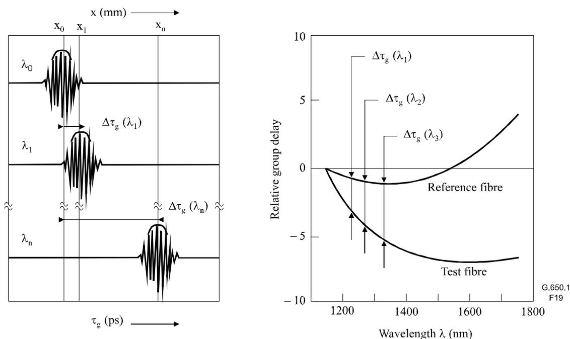
**Figure 19/G.650.1 – Determination of the spectral group delay**
