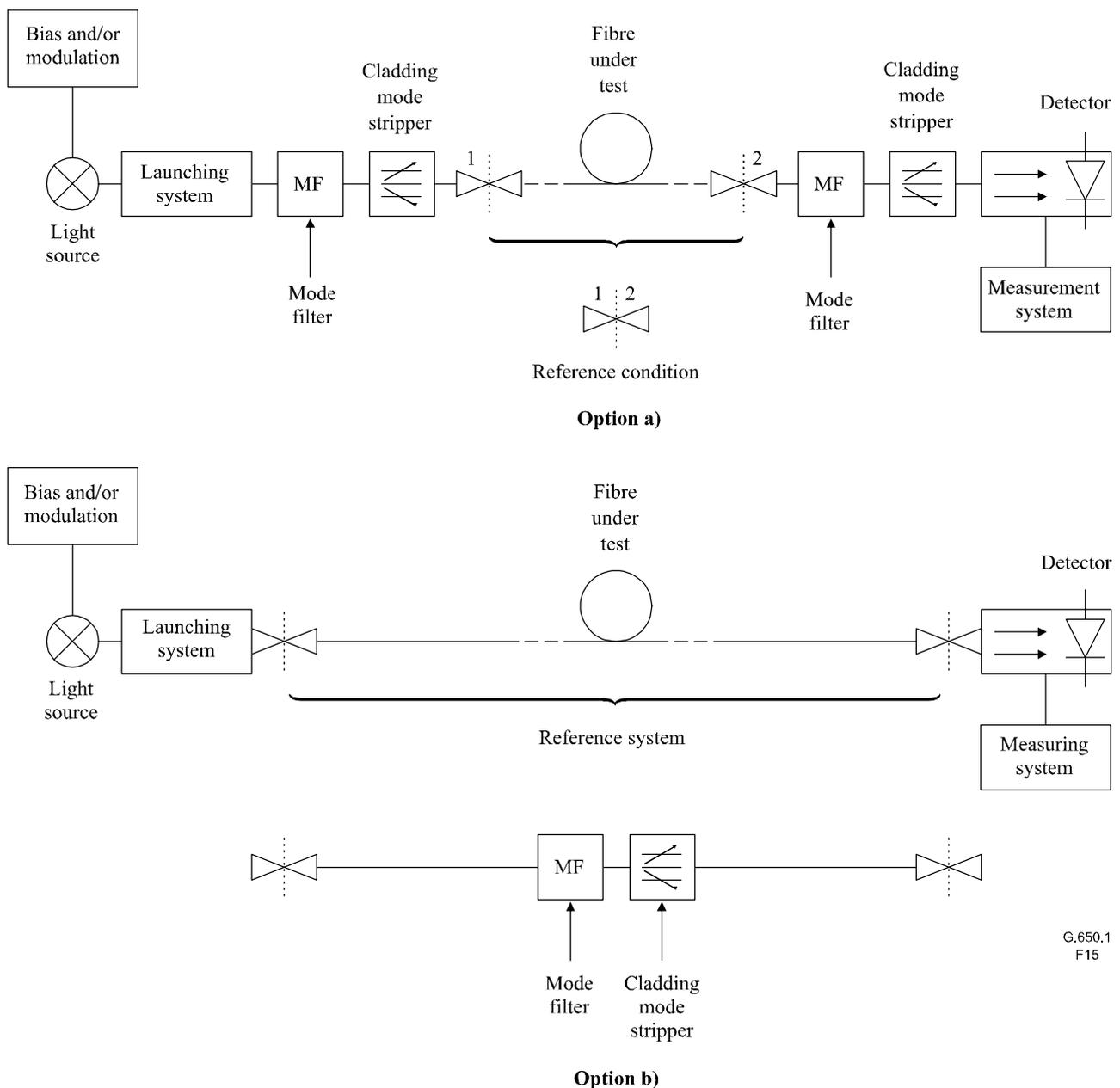
**Figure 15/G.650.1 – Typical arrangements for the insertion loss technique**
