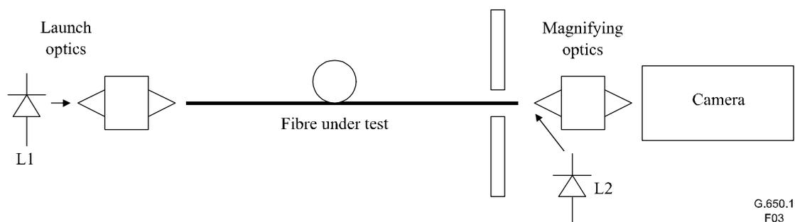
Figure 3/G.650.1 – A scheme for the test apparatus
