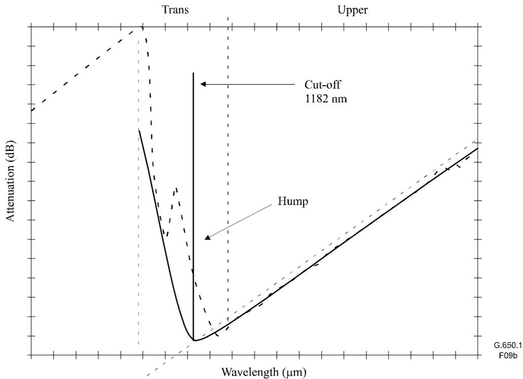
**Figure 9b/G.650.1 – Multimode reference cut-off plot with hump**
