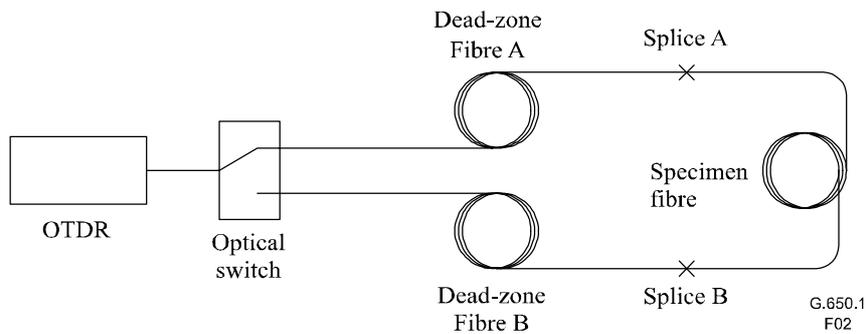
**Figure 2/G.650.1 – Optional apparatus for bidirectional backscatter**
