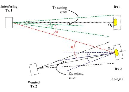
Figure I.6/G.640 – Example 3 crosstalk reference diagram for link 2
