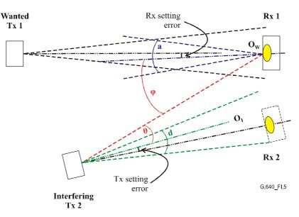
Figure I.5/G.640 – Example 3 crosstalk reference diagram for link 1
