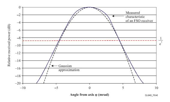
Figure 6-6/G.640 – Example measured curve of received power vs angle showing a Gaussian shape
