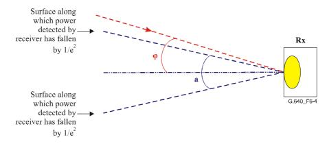
Figure 6-4/G.640 – Reference diagram for an FSO receiver
