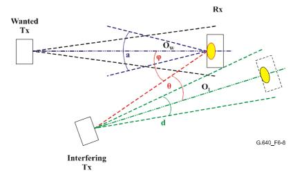
Figure 6-8/G.640 – FSO system crosstalk reference diagram
