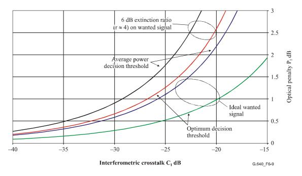
Figure 6-9/G.640 – Graph of optical penalty vs interferometric crosstalk for a single interferer (bounded model)
