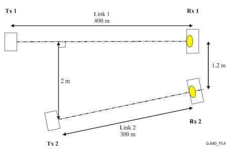
Figure I.4/G.640 – Example 3 configuration
