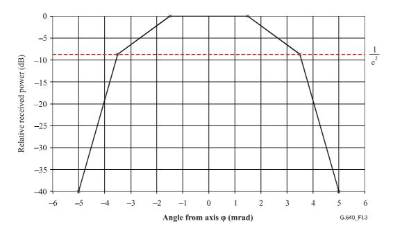
Figure I.3/G.640 – Worst-case curve of optical power detected by the receiver vs angle
