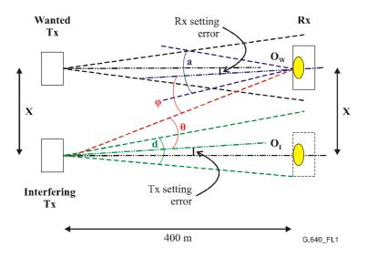
Figure I.1/G.640 – Example 1 crosstalk reference diagram
