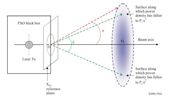
Figure 6-2/G.640 – Gaussian beam reference diagram for an FSO transmitter
