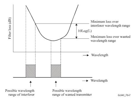
Figure 6-7/G.640 – Illustration of reduction of the interfering power due to optical filtering
