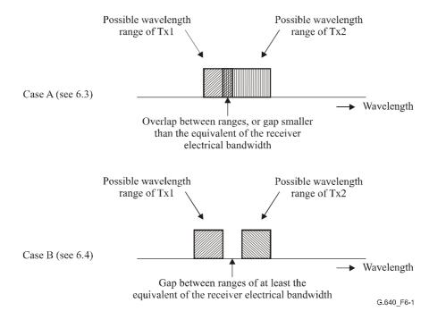
Figure 6-1/G.640 – Illustration of the difference between the cases covered by clauses 6.3 and 6.4
