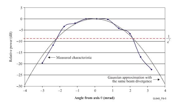
Figure 6-3/G.640 – Example measured curve of power density vs angle
