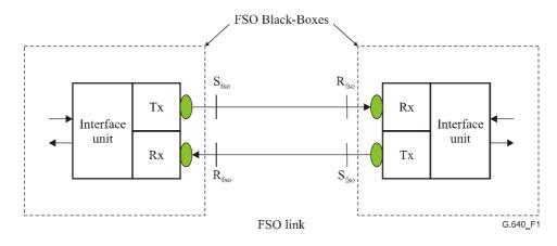
Figure 5-1/G.640 – Free space optical link reference diagram
