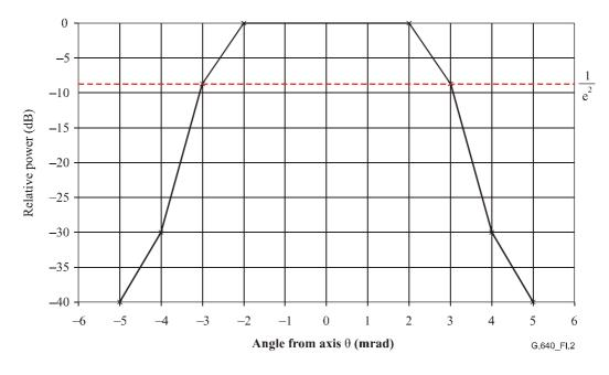
Figure I.2/G.640 – Worst-case curve of power density vs angle for the transmitters
