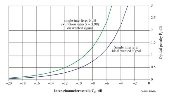
Figure 6-10/G.640 – Graph of optical penalty vs inter-channel crosstalk for a single interferer
