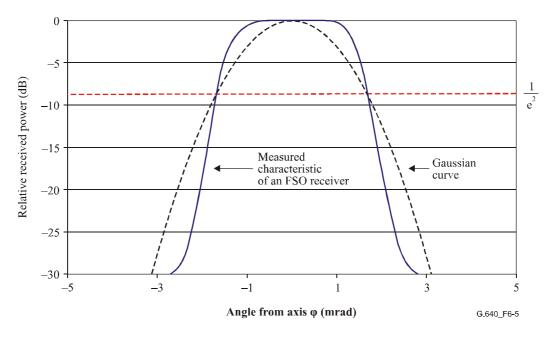
Figure 6-5/G.640 – Example measured curve of received power vs angle showing a rectangular shape
