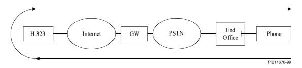
Figure 2/G.177 – Acoustic echo generated at the 4-wire H.323 terminal
