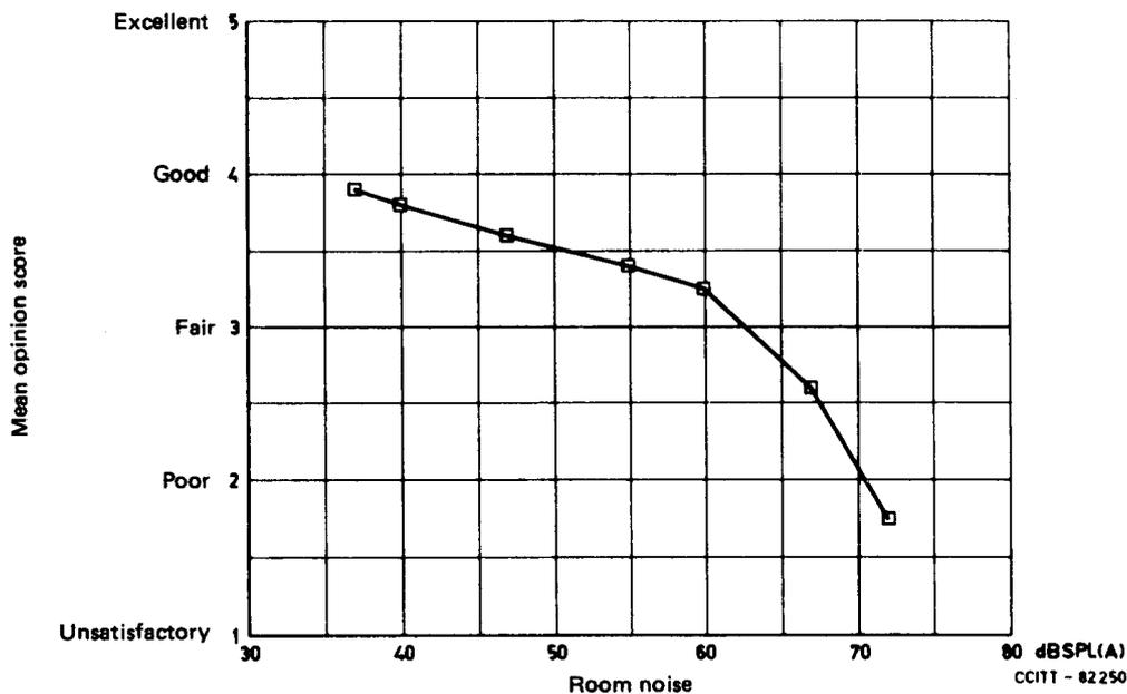
Note - This curve represents the opinion of customers listening over the telephone in room noise from 37 dB SPL(A) to 72 dB SPL(A). Each point is an average over all values of speech level and circuit noise given at that room noise level.
