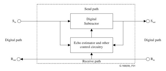
Figure 1 – Digital transmission echo canceller using digital subtraction
