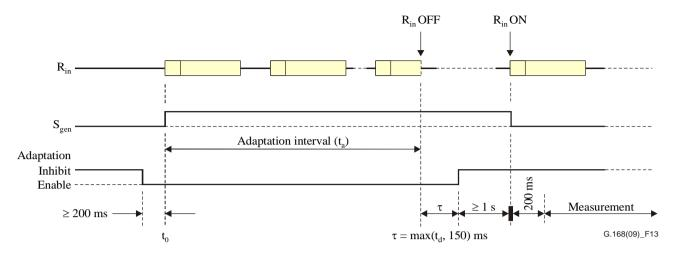
Figure 13 – Test No. 2C signal and time relationships
