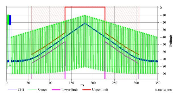
Figure 23a – Dynamic comfort noise level matching at ≥40 dB ERL
