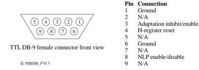
Figure VI.1 – Connector wiring for echo canceller cable
