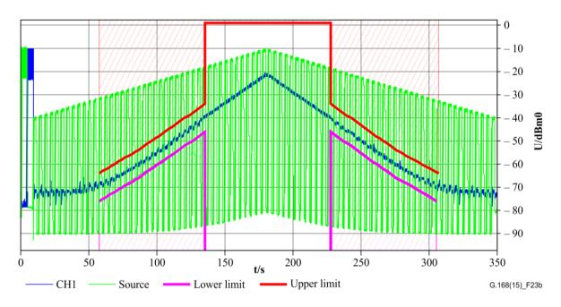
Figure 23b – Dynamic comfort noise level matching at 15 dB ERL
