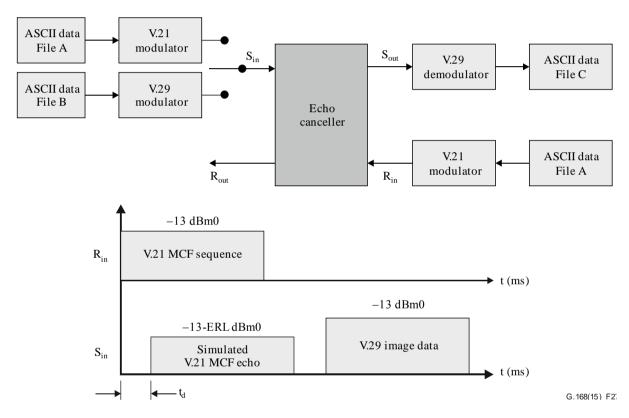
Figure 27 – Canceller operation during page transmission and page breaks
