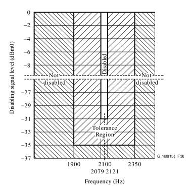
Figure 38 – Required disabling band characteristics
