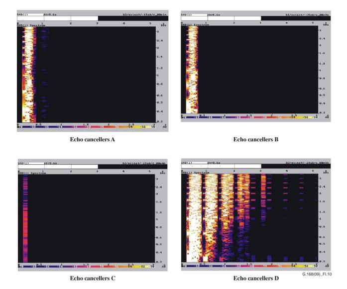
Figure I.10 – Spectral analysis of residual echo during initial convergence
