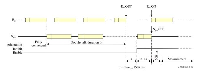
Figure 18 – Test No. 3B signal and time relationships
