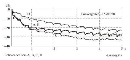
Figure I.7 – Convergence test versus time, digital echo path, ERL 6 dB, no cancelled end background noise, receive level –15 dBm0, NLP disabled
