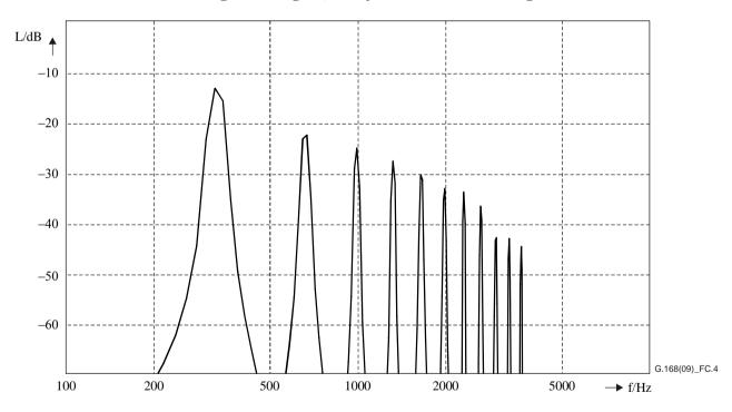
Figure C.4 – Power density spectrum of the bandlimited voiced signal (single talk signal, analysis window: Hanning)
