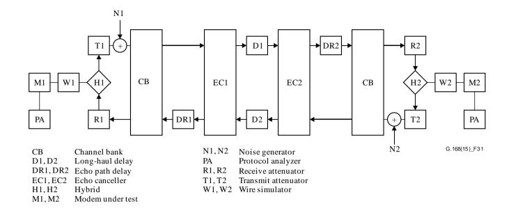
Figure 31 – Test No. 14 configuration
