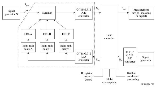
NOTE – The sum of the absolute values of the gains  $G_A$ ,  $G_B$ ,  $G_C$  that correspond to ERL A, B, C, respectively, taken in dB, should be less than or equal to –6 dB (i.e.,  $20\log(|G_A| + |G_B| + |G_C| \le -6$  dB), and echo path delay  $A \le \Delta$  ms, echo path delay  $A \le \Delta$  ms, and echo path delay  $A \le \Delta$  ms.
