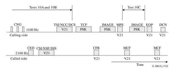
Figure 26 – Sequence of message exchange for a typical 2-page fax transmission
