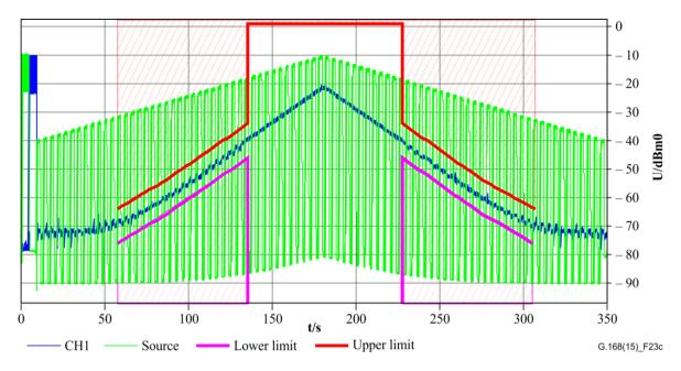
Figure 23c – Dynamic comfort noise level matching at 6 dB ERL
