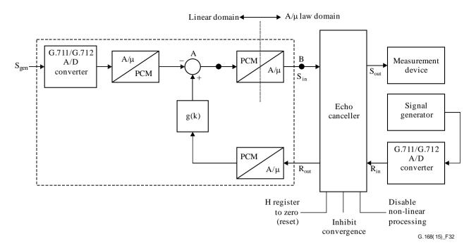
Figure 32 – Test configuration for S<sub>in</sub> PCM offset test
