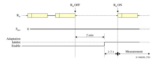
Figure 20 – Test No. 4 signal and time relationships
