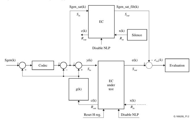
Figure I.2 – Test to subtract the double talk component from the send-out signal
