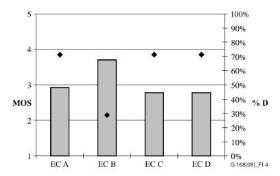
Figure I.4 – Results from *conversational tests*, overall quality mean opinion score (MOS) and % D (rhombus) for the 4 echo cancellers, ERL 7 dB, room noise level 40 dB(A), corresponding level –61 dBm0
