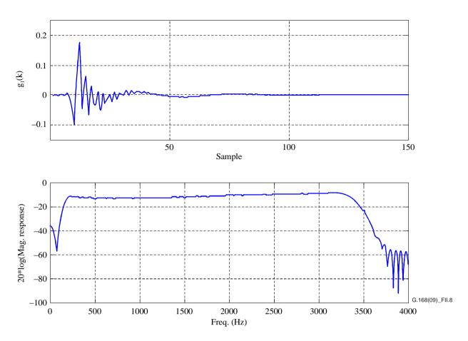
Figure II.8 – Echo path impulse response  $g_1$ , an ERL of 12 dB was used in the magnitude response plot
