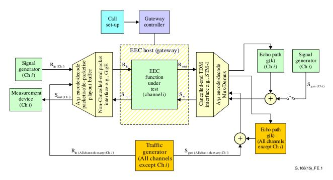
Figure E.1 – Test set-up for use with EECs
