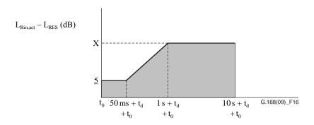
Figure 16 – Test No. 2C Convergence requirements NLP disabled
