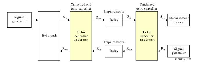
Figure 28 – Test No. 11 configuration
