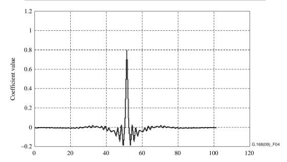
Figure 4 – Impulse response of frequency weighting network
