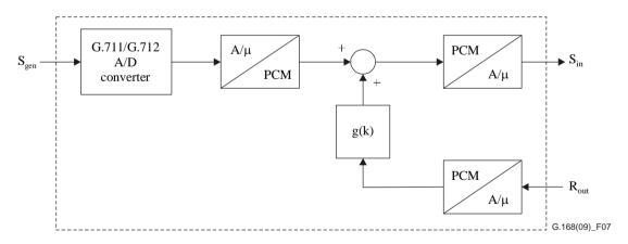
Figure 7 – Echo path model using g(k)
