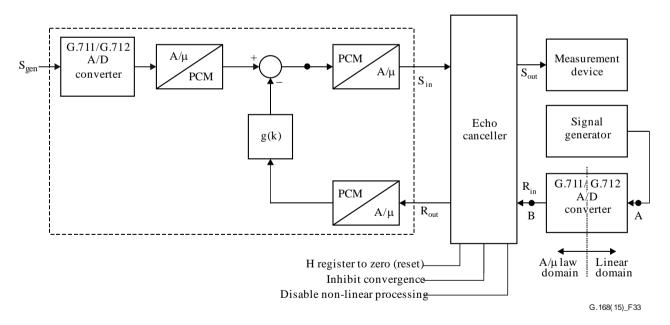
Figure 33 – Test configuration for Rin PCM offset test
