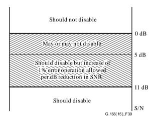
Figure 39 – Guardband and noise tolerance requirements
