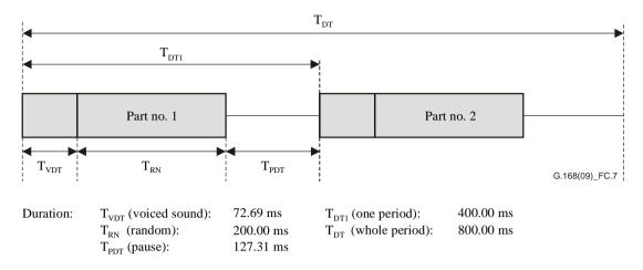
Figure C.7 – Composite source signals to simulate double talk (schematic)
