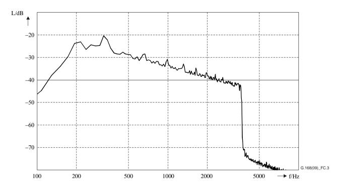
Figure C.3 – Power density spectrum of the bandlimited CSS (single talk signal, analysis window: Hanning)
