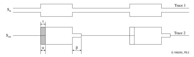
Figure B.2 – Traces for NLP operate and hangover time,  $L_{Rin}$  constant
