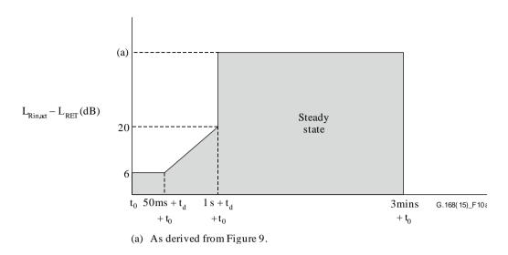
Figure 10a – Convergence characteristics with NLP enabled
