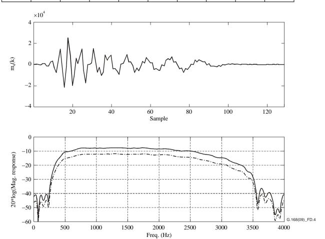
NOTE-12 dB ERL, CSS input with scaling factor from Table D.1a (solid line), tones(s) input with scaling factor from Table D.1b (dashed line).
