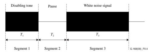
Figure II.4 – Test signal for echo-path measurement
