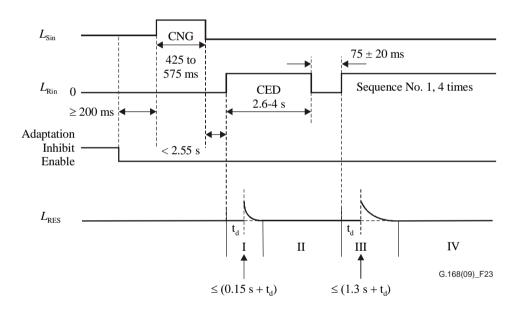
Figure 24 – Test No. 10A signal and time relationships
