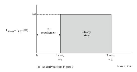
Figure 10b – Re-convergence characteristics with NLP enabled
