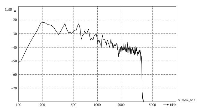
Figure C.5 – Power density spectrum of the bandlimited double-talk CSS (analysis window: Hanning)
