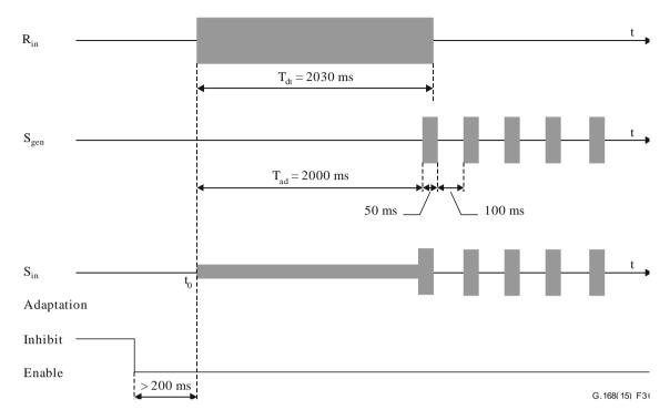
Figure 36 – Test timing version 2: a "typical" DTMF reaction and an almost instantaneous removal of the dial tone upon detection of the first DTMF digit by the system
