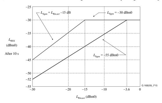
Figure 15 - Test No. 2C steady state requirements NLP disabled
