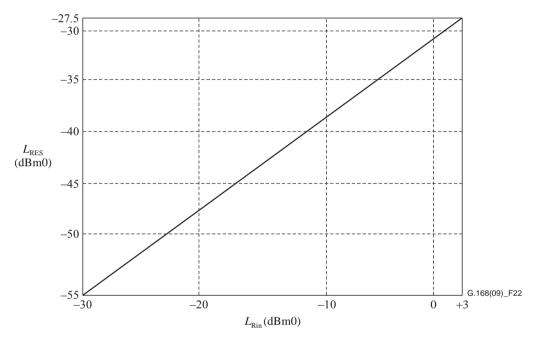
Note that the equation for the line in Figure 22 is:  $L_{Res} = 0.83L_{Rin} - 30$ .
