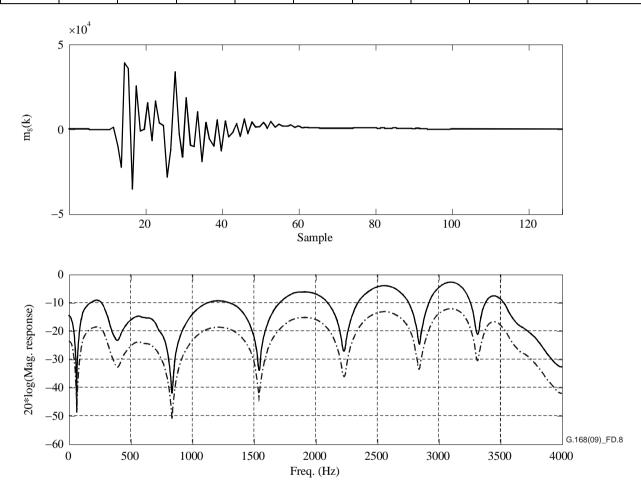
$NOTE-12\ dB\ ERL$ , CSS input with scaling factor from Table D.1a (solid line), tones(s) input with scaling factor from Table D.1b (dashed line).
