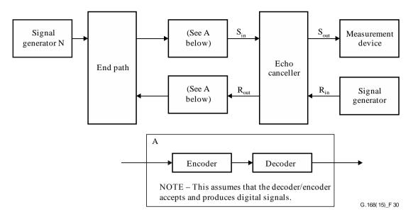
Figure 30 – Test No. 13 configuration
