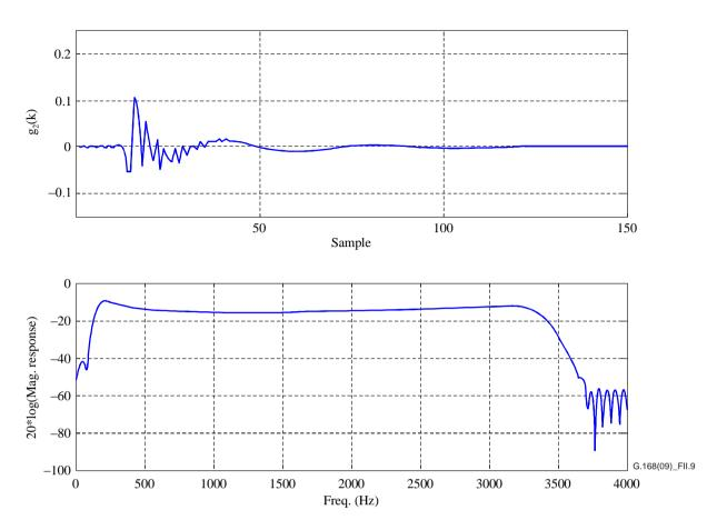
Figure II.9 – Echo path impulse response  $g_2$ , an ERL of 12 dB was used in the magnitude response plot
