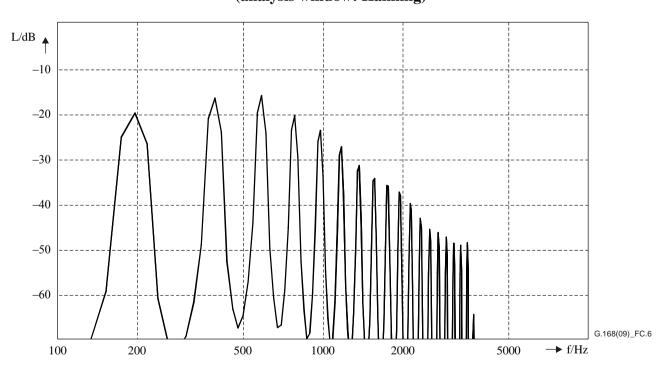
Figure C.6 – Power density spectrum of the bandlimited double talk-voiced signal (analysis window: Hanning)
