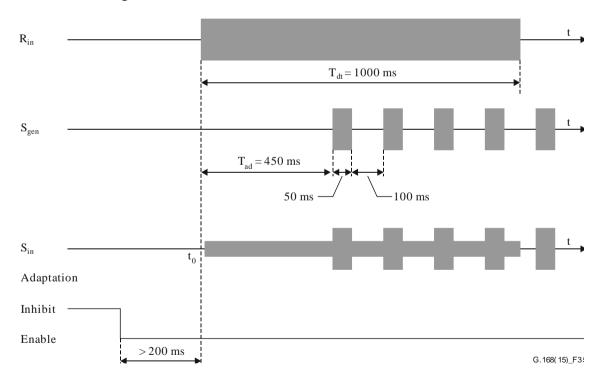
Figure 35 – Test timing version 1: "fast" DTMF reaction and a "slow" removal of the dial tone
