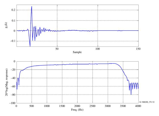
Figure II.10 – Echo path impulse response *g*<sub>3</sub>, an ERL of 12 dB was used in the magnitude response plot
