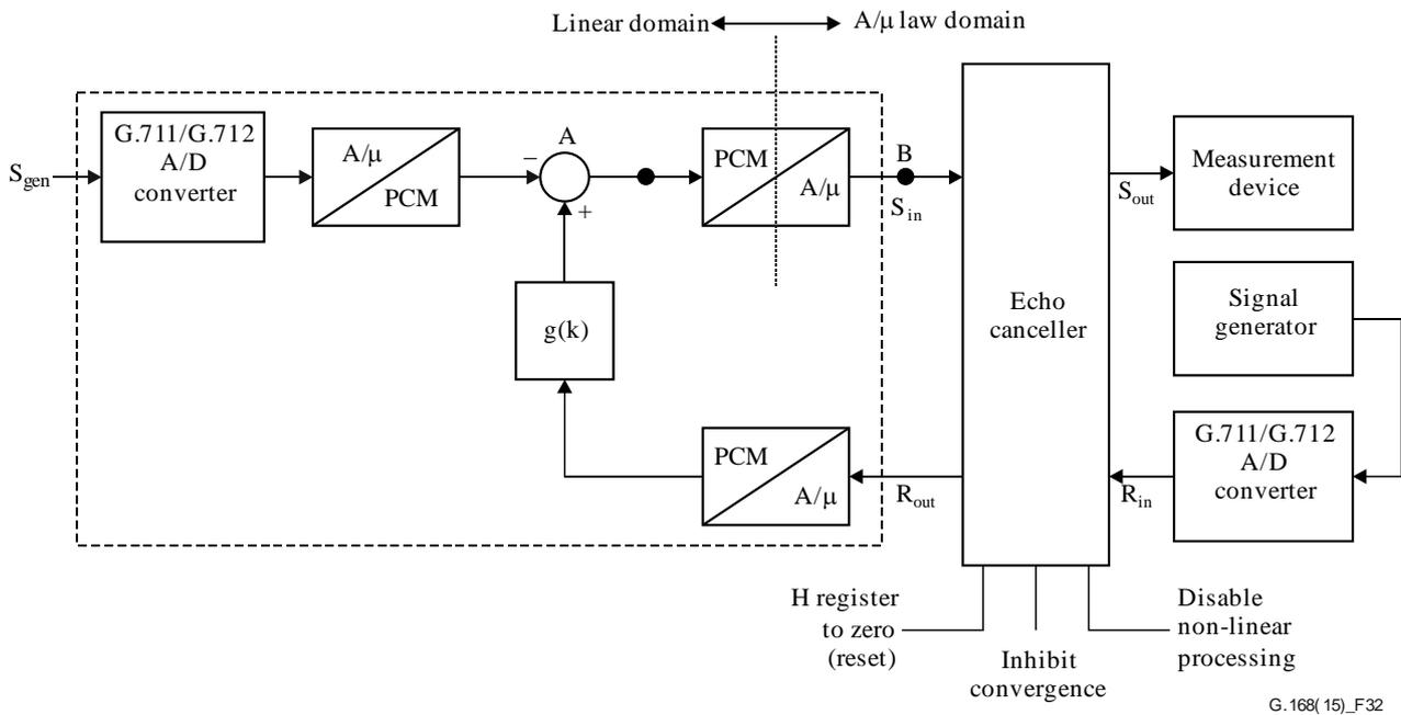
**Figure 32 – Test configuration for  $S_{in}$  PCM offset test**
