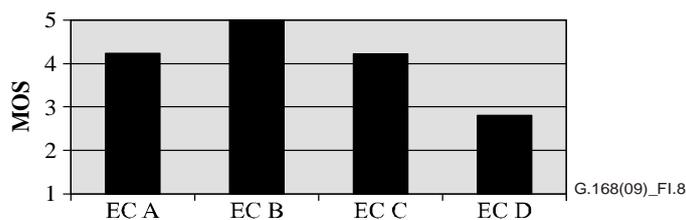
**Figure I.8 – Results from *talking and listening tests*, MOS, disturbance caused by echoes, digital echo path, ERL 6 dB, background noise  $-55\text{ dBm}_0$ , NLP enabled**
