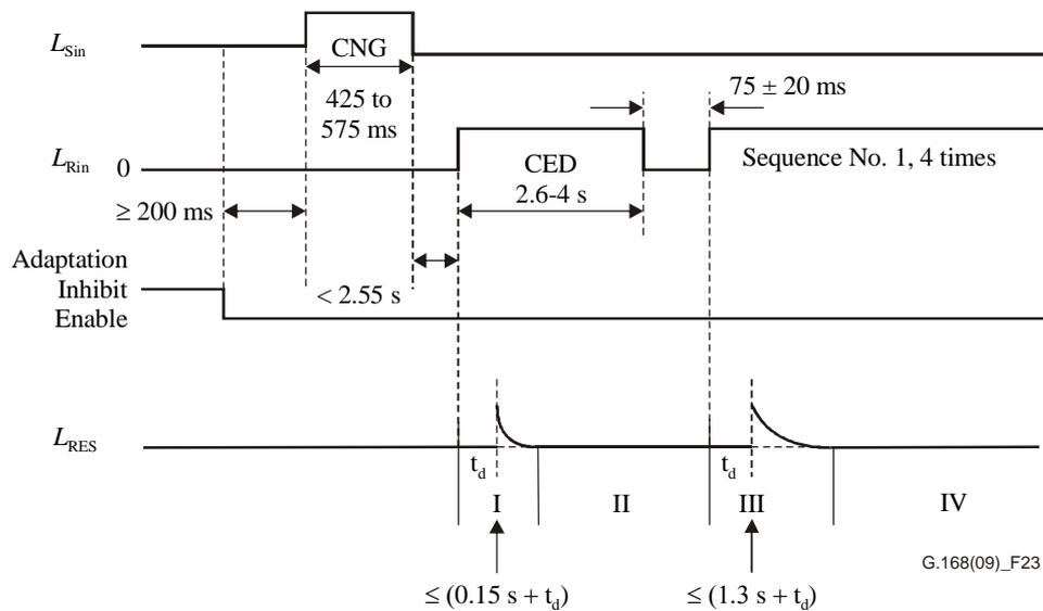
**Figure 24 – Test No. 10A signal and time relationships**
