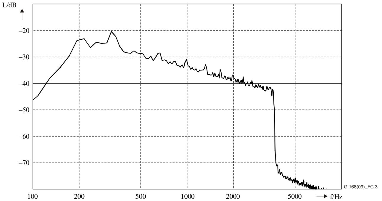
**Figure C.3 – Power density spectrum of the bandlimited CSS
