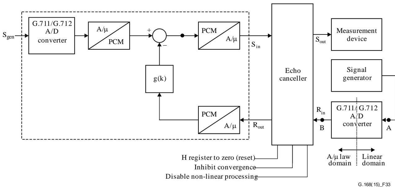
**Figure 33 – Test configuration for  $R_{in}$  PCM offset test**
