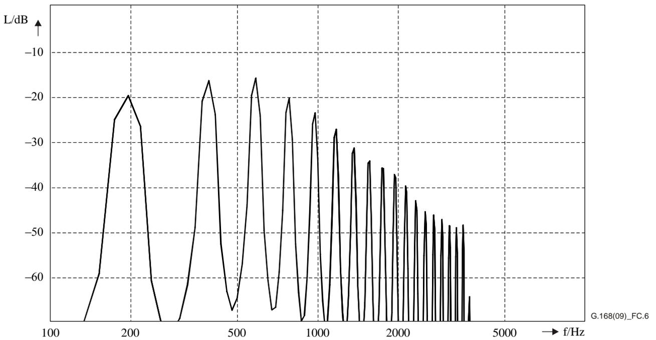
**Figure C.6 – Power density spectrum of the bandlimited double talk-voiced signal
