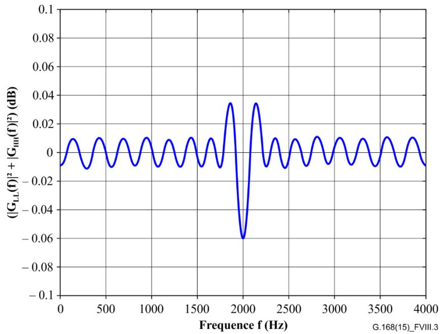
**Figure VIII.3 – Total gain resulting from  $G_{LL}(z)$ ,  $G_{HH}(z)$**
