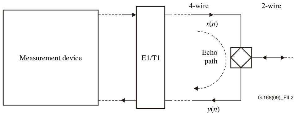
**Figure II.2 – Block diagram of intrusive measurement set-up**
