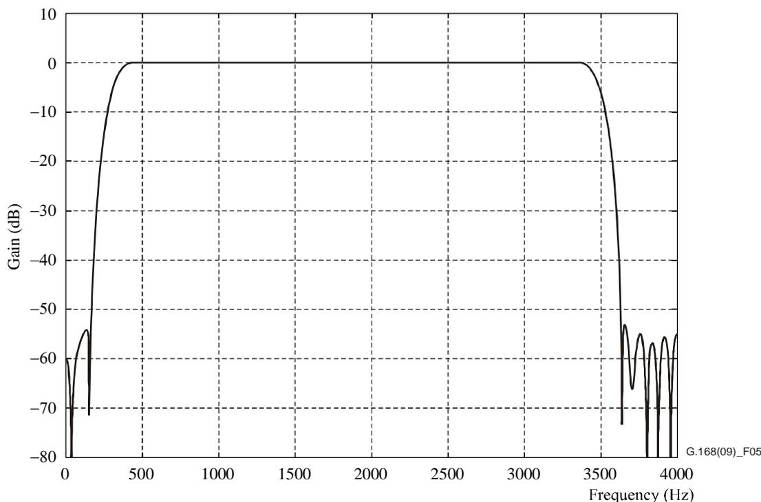
**Figure 5 – Magnitude response of frequency weighting network**
