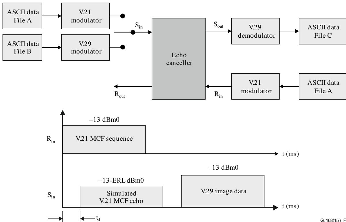
**Figure 27 – Canceller operation during page transmission and page breaks**
