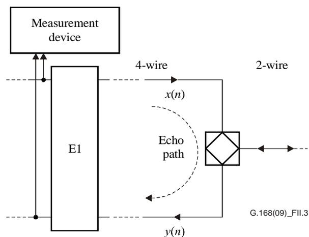
**Figure II.3 – Block diagram of non-intrusive measurement set-up**
