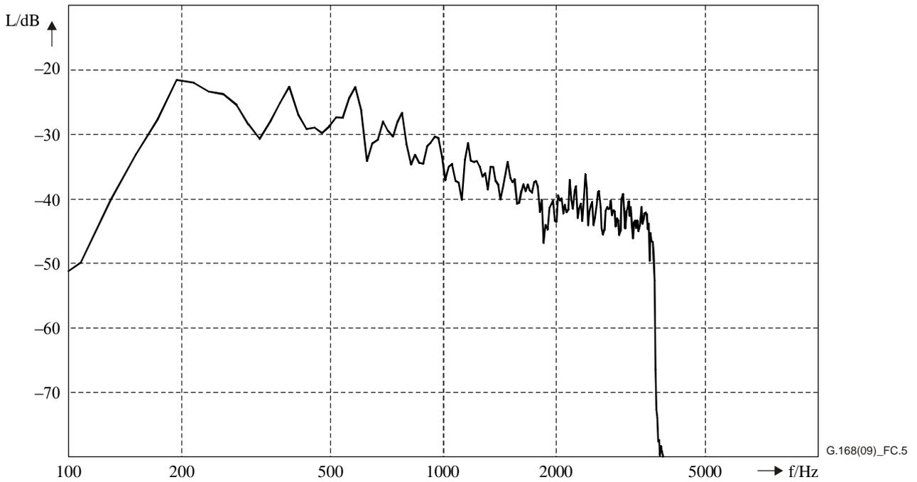
**Figure C.5 – Power density spectrum of the bandlimited double-talk CSS
