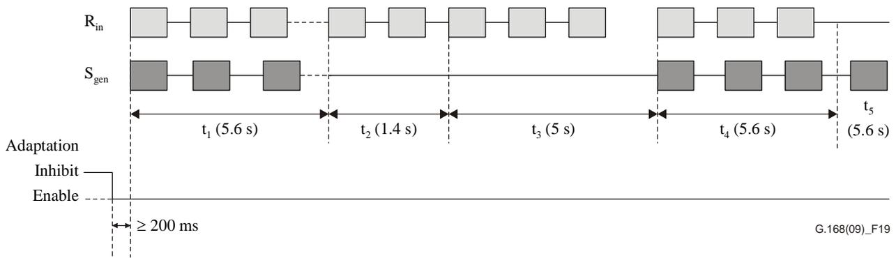
**Figure 19 – Test No. 3C signal and time relationships**
