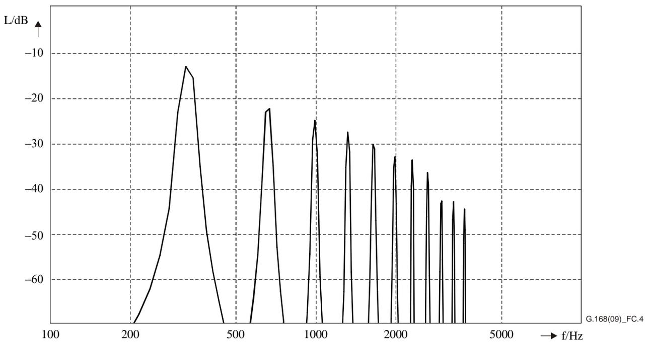
**Figure C.4 – Power density spectrum of the bandlimited voiced signal
