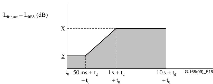
**Figure 16 – Test No. 2C Convergence requirements NLP disabled**
