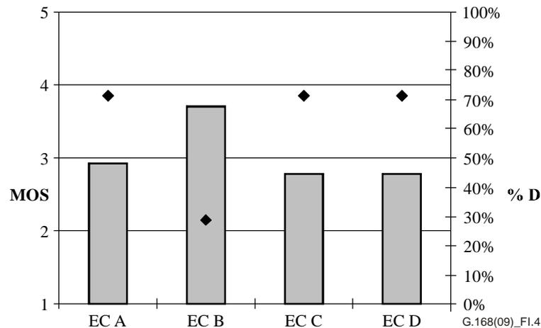
**Figure I.4 – Results from *conversational tests*, overall quality mean opinion score (MOS) and % D (rhombus) for the 4 echo cancellers, ERL 7 dB, room noise level 40 dB(A), corresponding level –61 dBm0**
