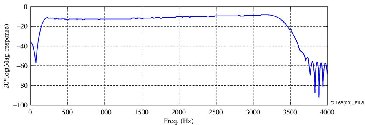
**Figure II.8 – Echo path impulse response  $g_1$ , an ERL of 12 dB was used in the magnitude response plot**
