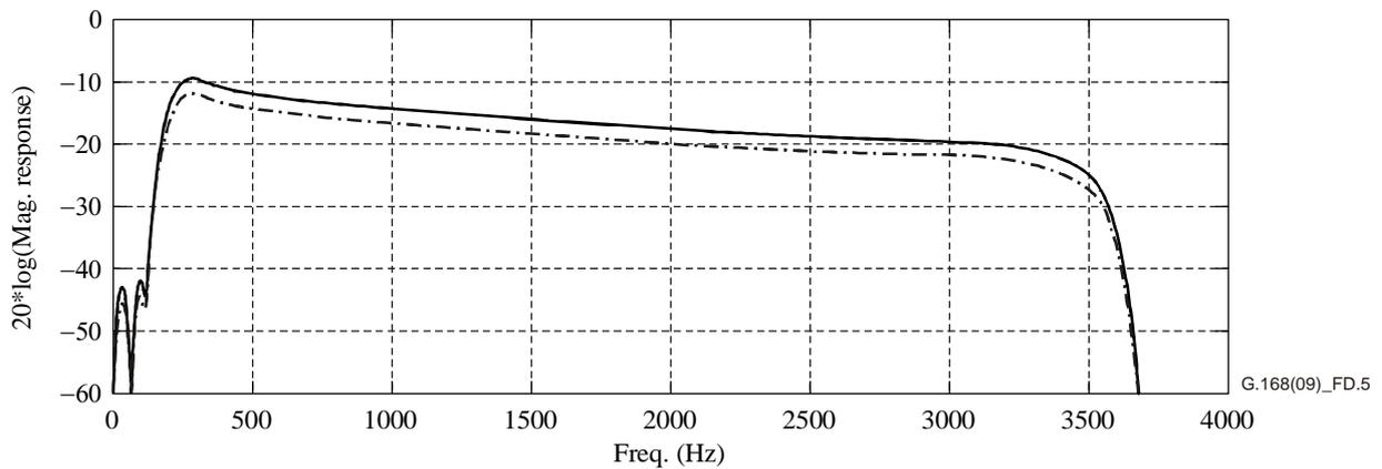
NOTE – 12 dB ERL, CSS input with scaling factor from Table D.1a (solid line), tones(s) input with scaling factor from Table D.1b (dashed line).
