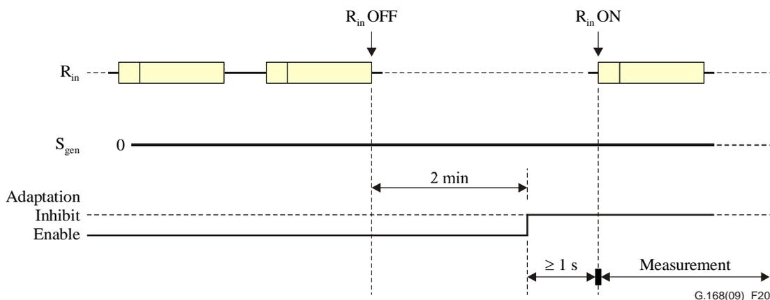
**Figure 20 – Test No. 4 signal and time relationships**
