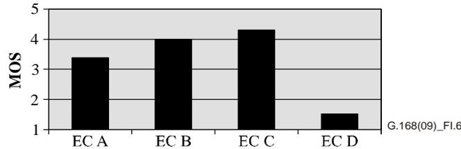
**Figure I.6 – Results from *talking and listening tests*, MOS, disturbance caused by echoes, digital echo path, ERL 6 dB, no cancelled end background noise, NLP disabled**
