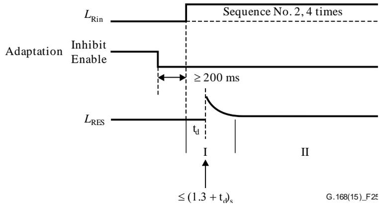
**Figure 25 – Test No. 10B signal and time relationships**
