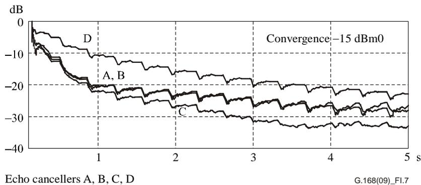
**Figure I.7 – Convergence test versus time, digital echo path, ERL 6 dB, no cancelled end background noise, receive level  $-15\text{ dBm}_0$ , NLP disabled**
