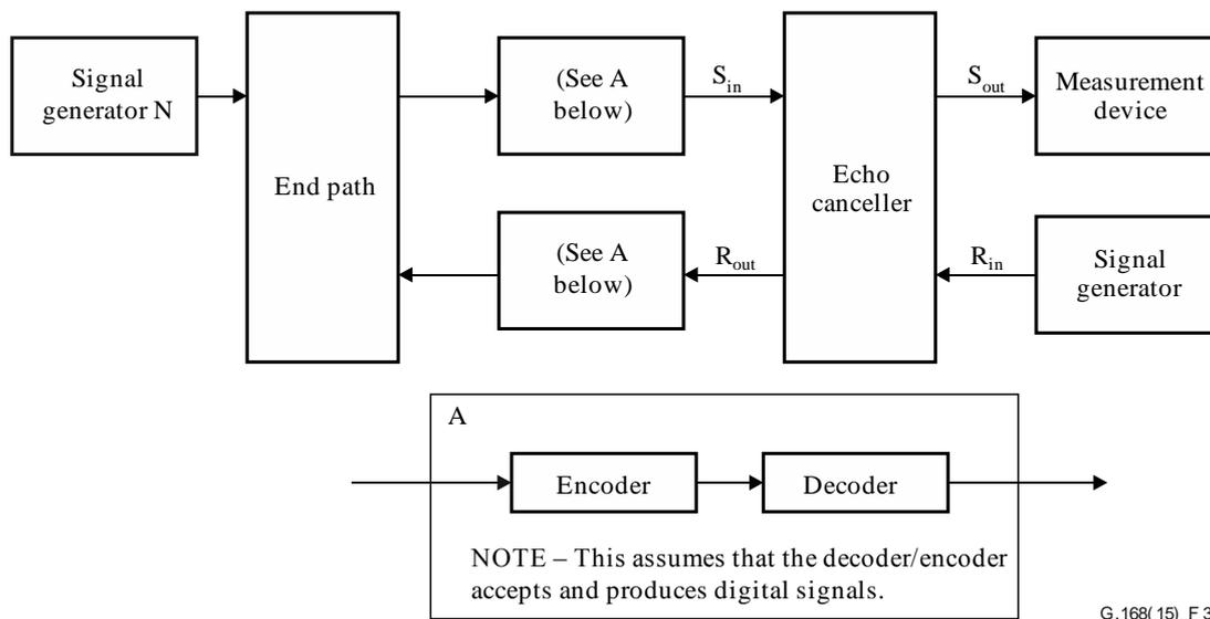
**Figure 30 – Test No. 13 configuration**
