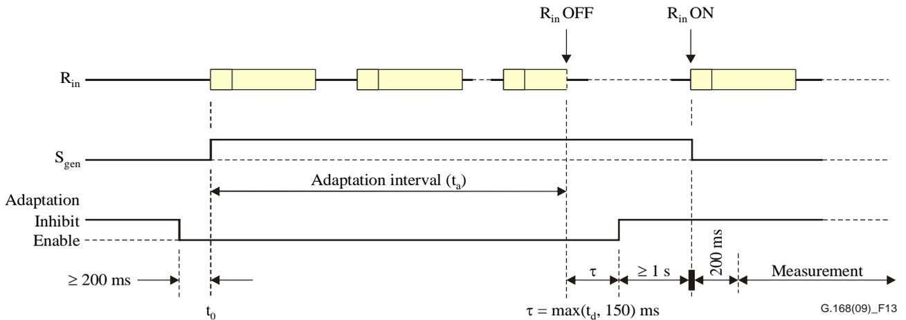
**Figure 13 – Test No. 2C signal and time relationships**
