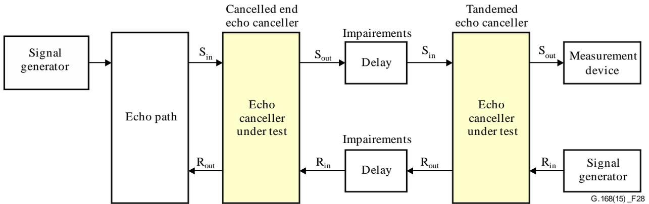
**Figure 28 – Test No. 11 configuration**
