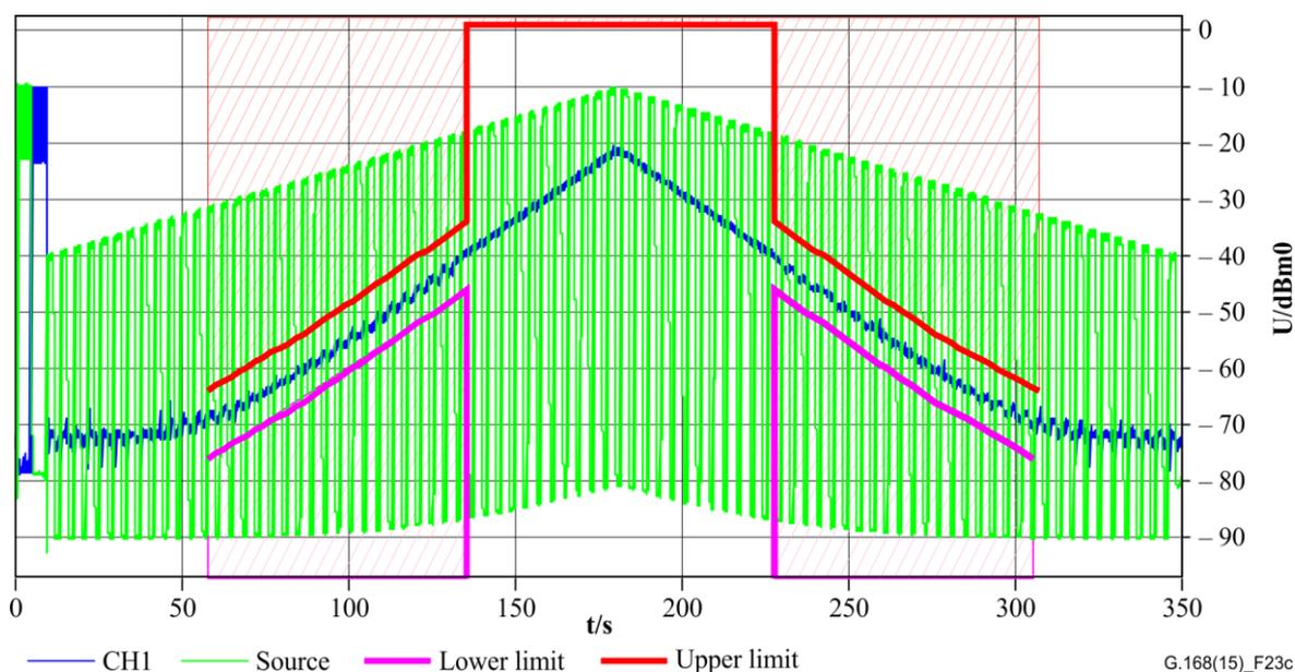
**Figure 23c – Dynamic comfort noise level matching at 6 dB ERL**
