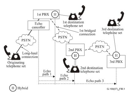
Figure III.1 – Multiple tails in a typical bridged telephone call
