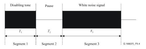
Figure II.4 – Test signal for echo-path measurement
