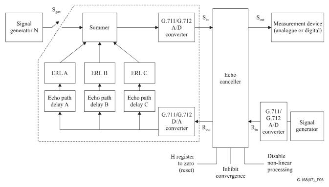
NOTE – The sum of the absolute values of the gains  $G_A$ ,  $G_B$ ,  $G_C$  that correspond to ERL A, B, C, respectively, taken in dB, should be less than or equal to -6 dB (i.e.,  $20\log(|G_A| + |G_B| + |G_C| \le -6 \text{ dB})$ , and echo path delay  $A \le \Delta$  ms, echo path delay  $B \le \Delta$  ms, and echo path delay  $C \le \Delta$  ms.
