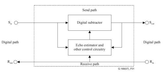
Figure 1 – Digital transmission echo canceller using digital subtraction
