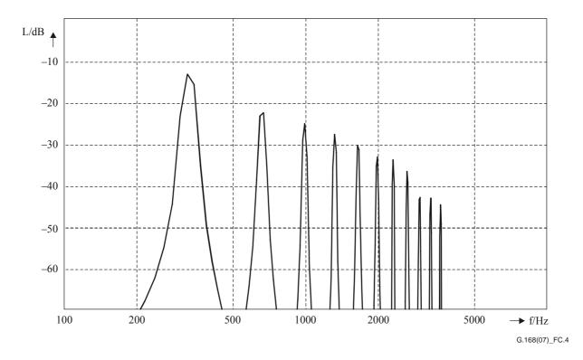
Figure C.4 – Power density spectrum of the bandlimited voiced signal (single talk signal, analysis window: Hanning)
