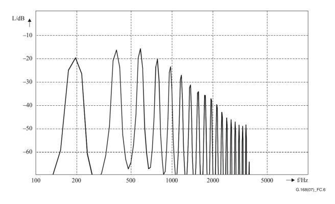
Figure C.6 – Power density spectrum of the bandlimited double talk-voiced signal (analysis window: Hanning)
