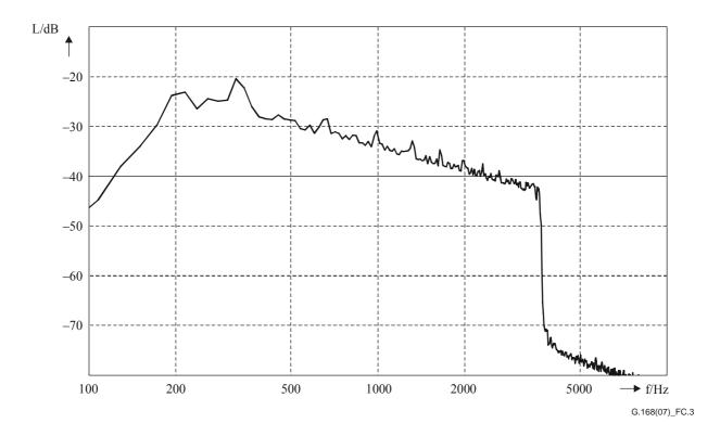
Figure C.3 – Power density spectrum of the bandlimited CSS (single talk signal, analysis window: Hanning)
