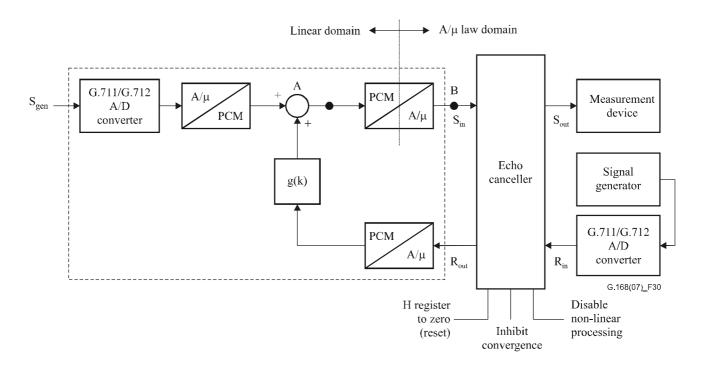
Figure 30 – Test configuration for S<sub>in</sub> PCM offset test
