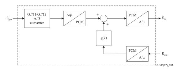
Figure 7 – Echo path model using g(k)
