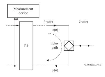
Figure II.3 – Block diagram of non-intrusive measurement set-up
