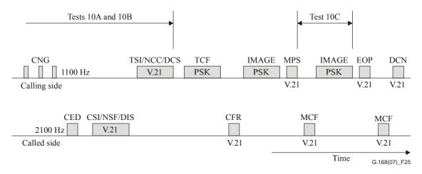
Figure 25 – Sequence of message exchange for a typical 2-page fax transmission
