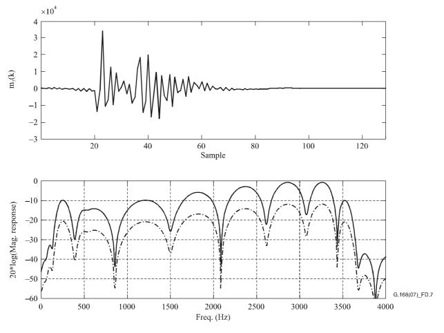
NOTE – 12 dB ERL, CSS input with scaling factor from Table D.1a (solid line), tones(s) input with scaling factor aofrom Table D.1b (dashed line).
