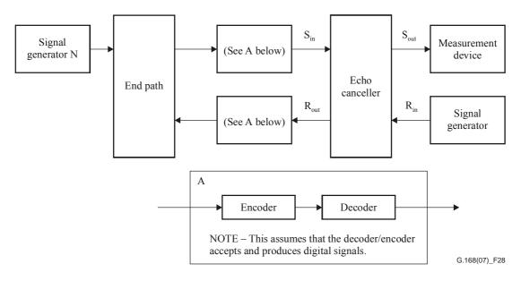
Figure 28 – Test No. 13 configuration
