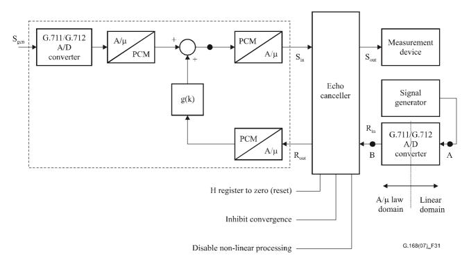
Figure 31 – Test configuration for  $R_{\text{in}}\ PCM$  offset test
