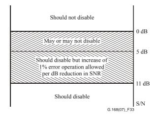
Figure 33 – Guardband and noise tolerance requirements
