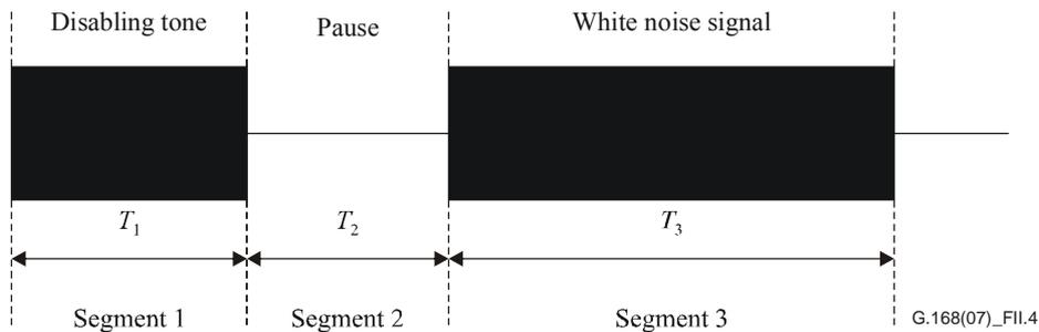
Figure II.4 – Test signal for echo-path measurement
