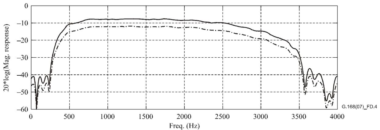
NOTE – 12 dB ERL, CSS input with scaling factor from Table D.1a (solid line), tones(s) input with scaling factor from Table D.1b (dashed line).
