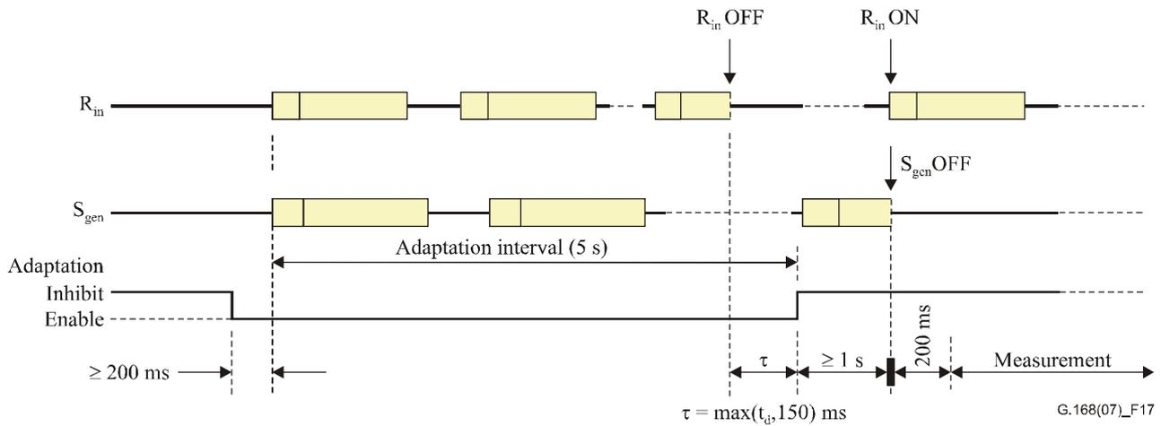
**Figure 17 – Test No. 3A signal and time relationships**
