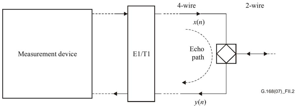
**Figure II.2 – Block diagram of intrusive measurement set-up**
