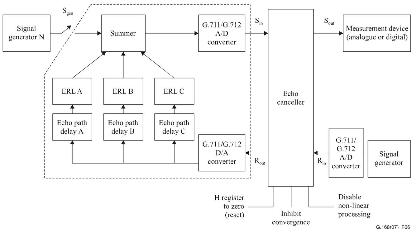
NOTE – The sum of the absolute values of the gains  $G_A$ ,  $G_B$ ,  $G_C$  that correspond to ERL A, B, C, respectively, taken in dB, should be less than or equal to  $-6$  dB (i.e.,  $20\log(|G_A| + |G_B| + |G_C|) \leq -6$  dB), and echo path delay A  $\leq \Delta$  ms, echo path delay B  $\leq \Delta$  ms, and echo path delay C  $\leq \Delta$  ms.
