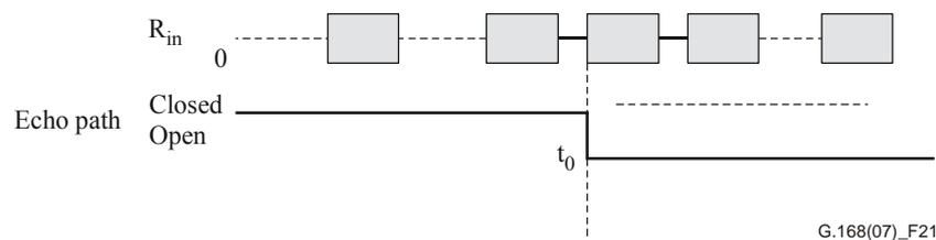
Figure 21 – Test No. 5 signal and time relationships
