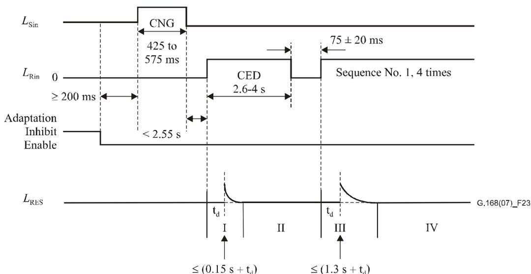
**Figure 23 – Test No. 10A signal and time relationships**
