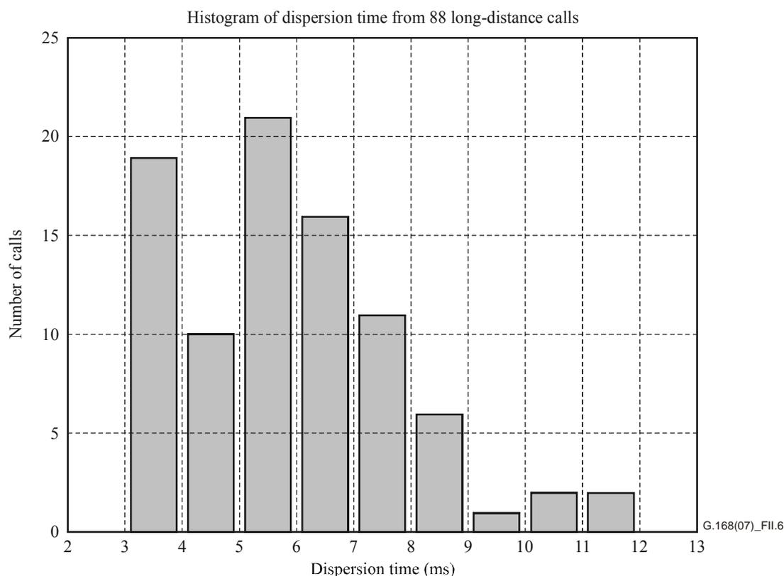
**Figure II.6 – Histogram of dispersion time for long-distance calls:
