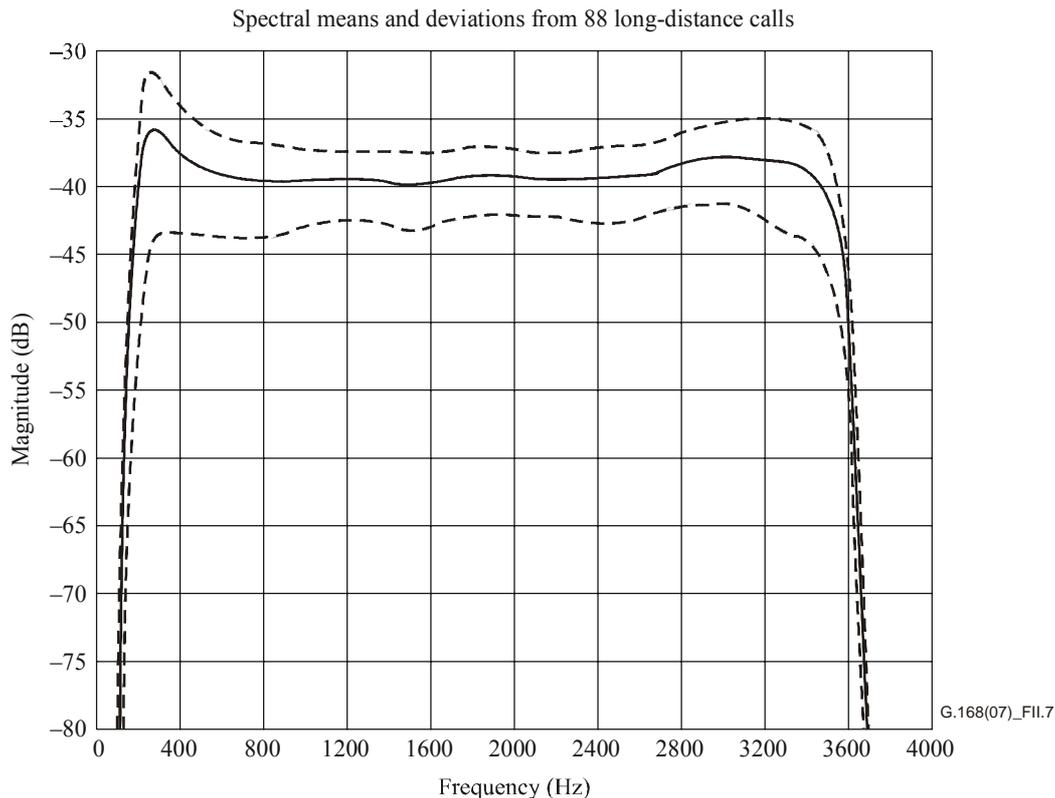
**Figure II.7 – Magnitude spectra of echo paths for long-distance calls, echo paths normalized to have unity energy**
