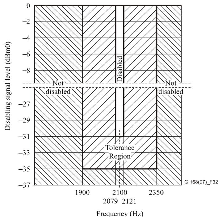
Figure 32 – Required disabling band characteristics
