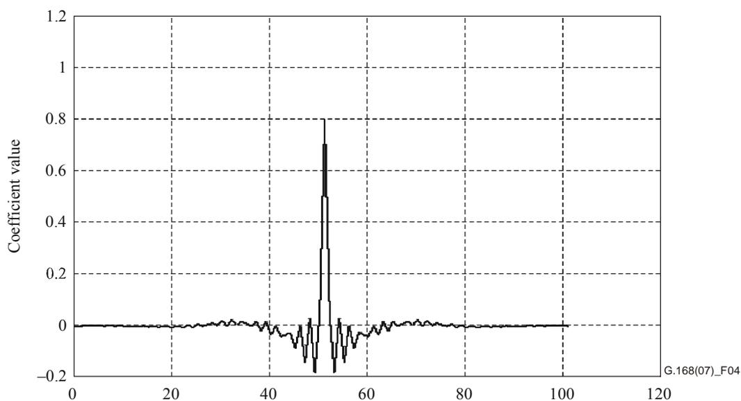
**Figure 4 – Impulse response of frequency weighting network**
