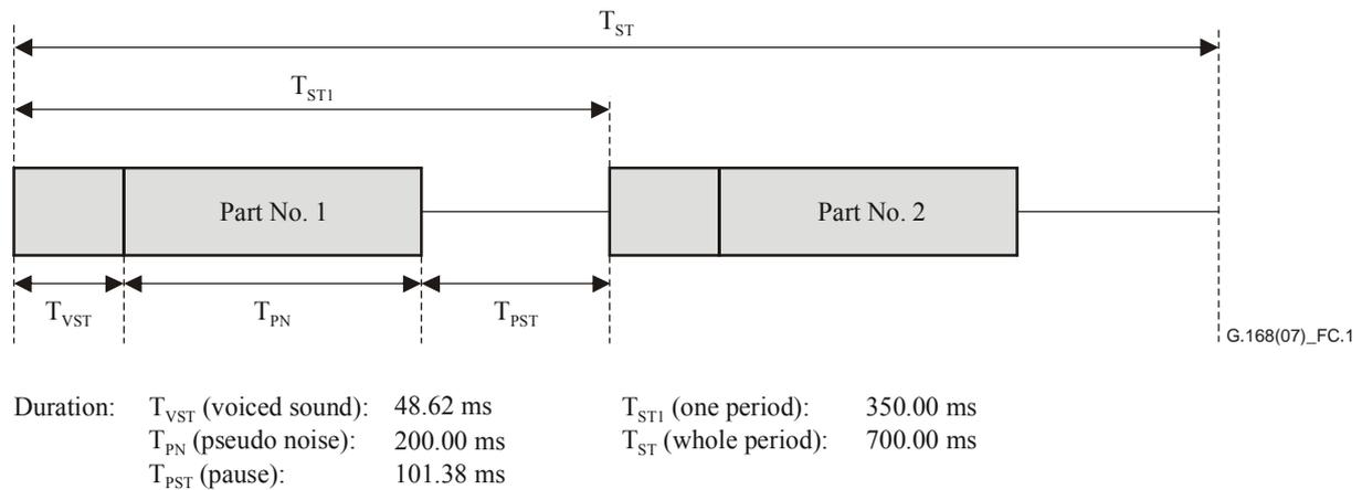
**Figure C.1 – Composite source signal for measuring echo cancellers (schematic)**
