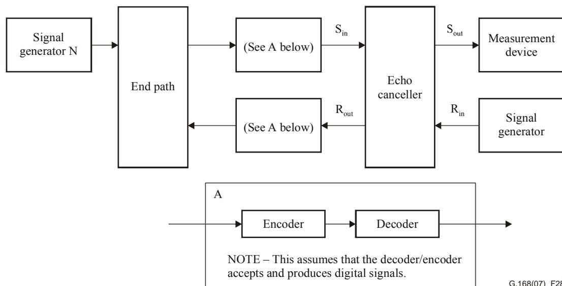
**Figure 28 – Test No. 13 configuration**
