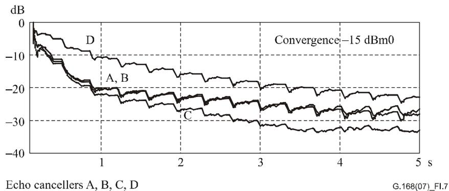
**Figure I.7 – Convergence test versus time, digital echo path, ERL 6 dB, no cancelled end background noise, receive level  $-15$  dBm0, NLP disabled**
