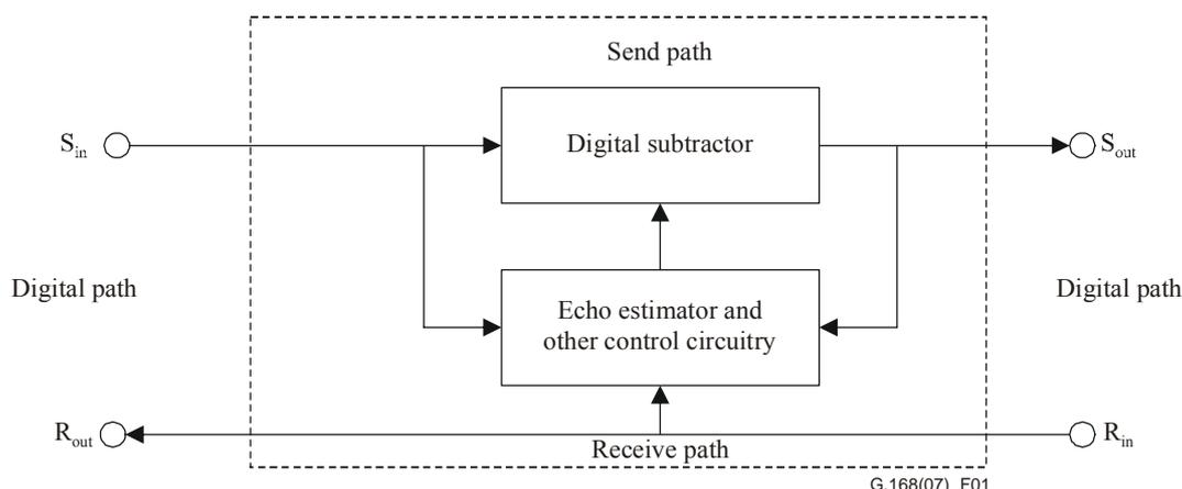
**Figure 1 – Digital transmission echo canceller using digital subtraction**
