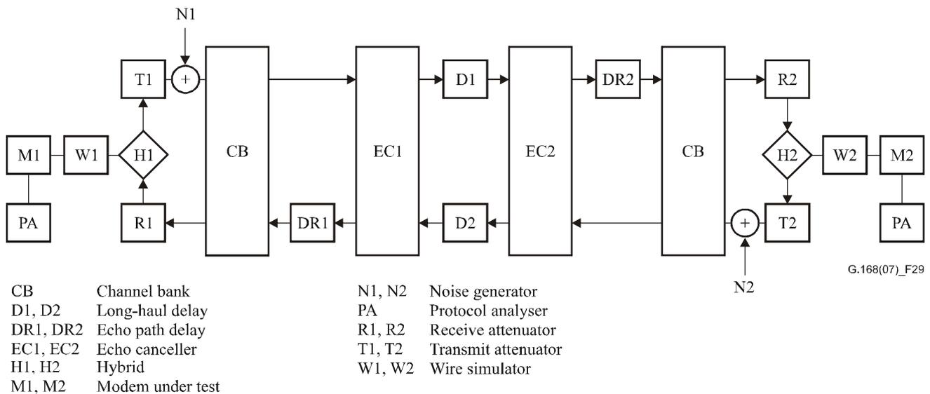
**Figure 29 – Test No. 14 configuration**
