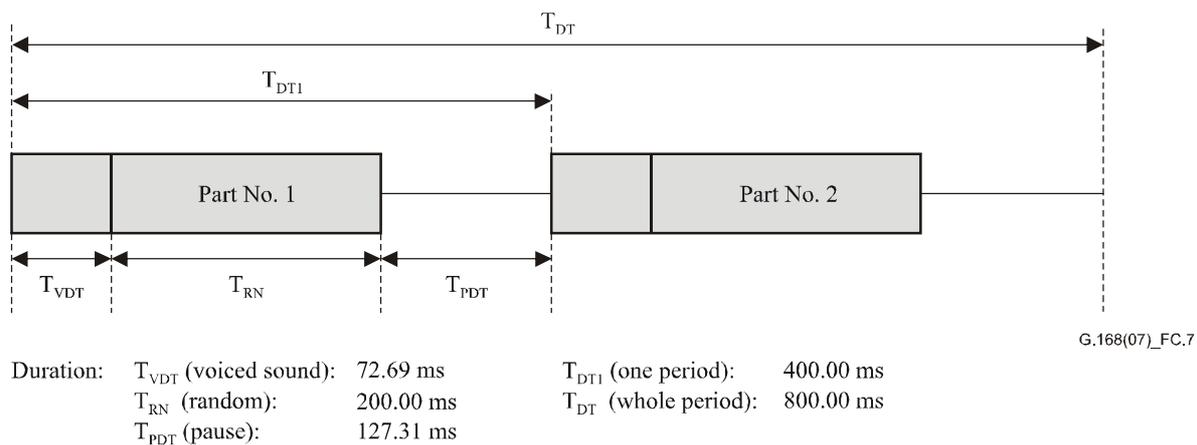
**Figure C.7 – Composite source signals to simulate double talk (schematic)**
