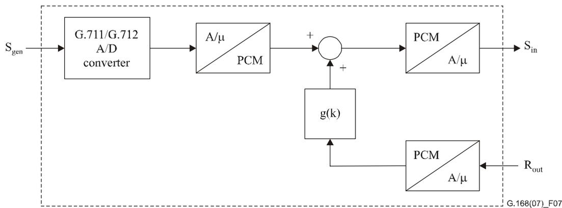
**Figure 7 – Echo path model using  $g(k)$**
