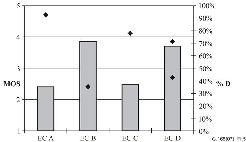
**Figure I.5 – Results from *conversational tests*, overall quality MOS and % D (rhombus) for the 4 echo cancellers, 4-wire echo path, room noise level 50 dB(A), corresponding level –55 dBm0**
