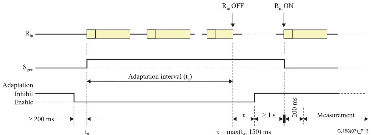
**Figure 13 – Test No. 2C signal and time relationships**
