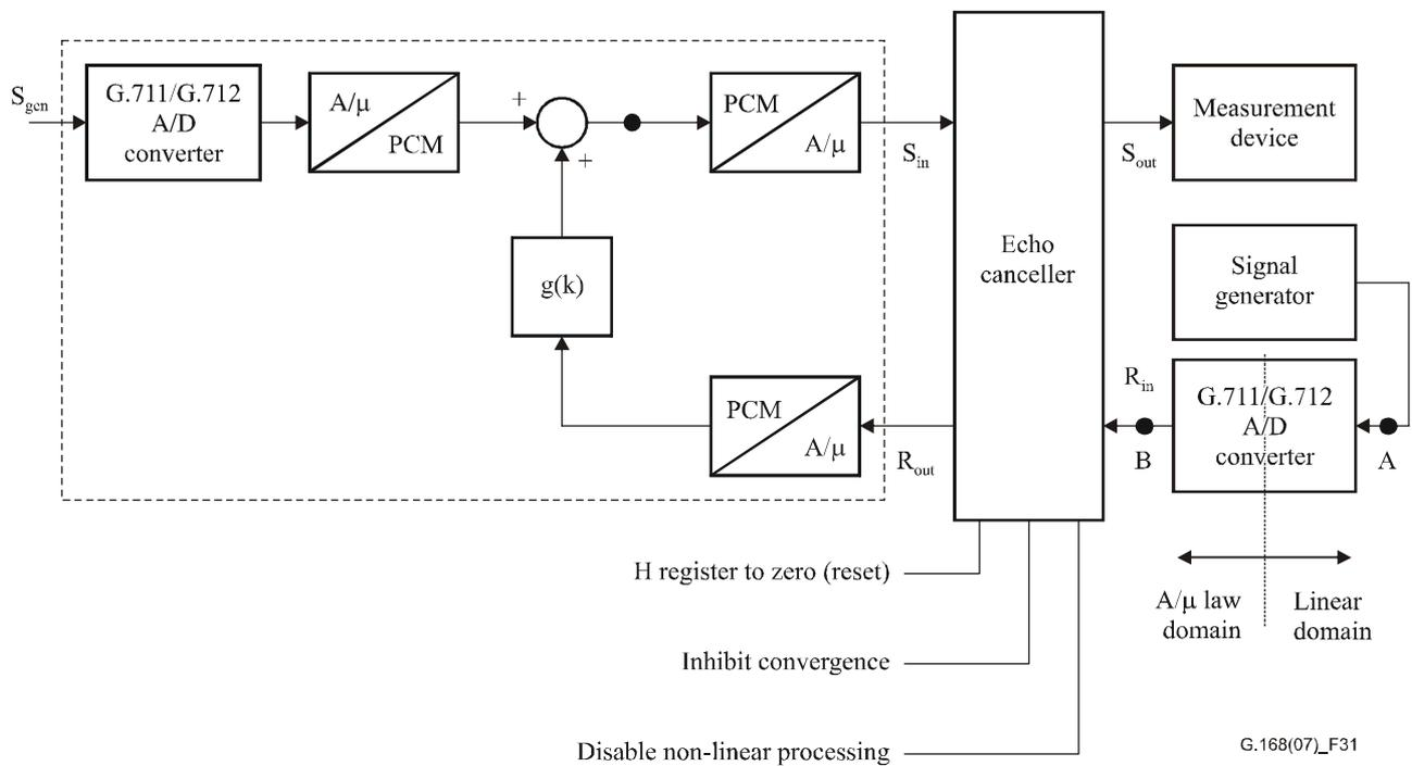
**Figure 31 – Test configuration for  $R_{in}$  PCM offset test**
