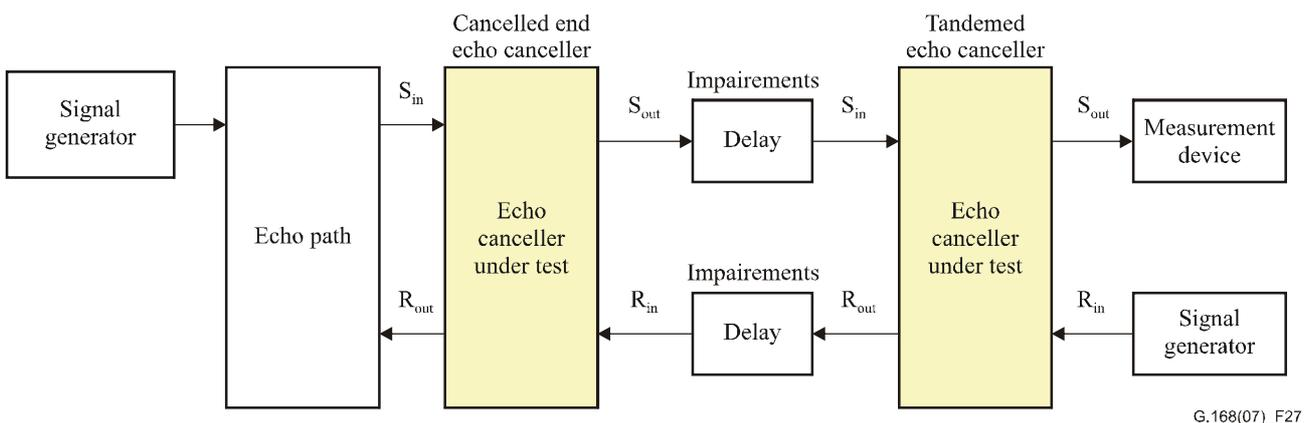
**Figure 27 – Test No. 11 configuration**
