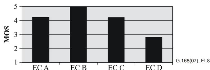
**Figure I.8 – Results from *talking and listening tests*, MOS, disturbance caused by echoes, digital echo path, ERL 6 dB, background noise –55 dBm0, NLP enabled**
