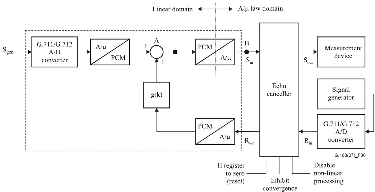
**Figure 30 – Test configuration for  $S_{in}$  PCM offset test**
