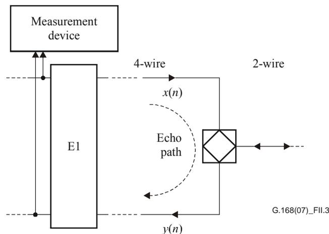
**Figure II.3 – Block diagram of non-intrusive measurement set-up**
