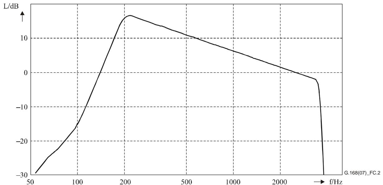
**Figure C.2 – Transfer function of the filter for bandlimiting the PN-sequence**
