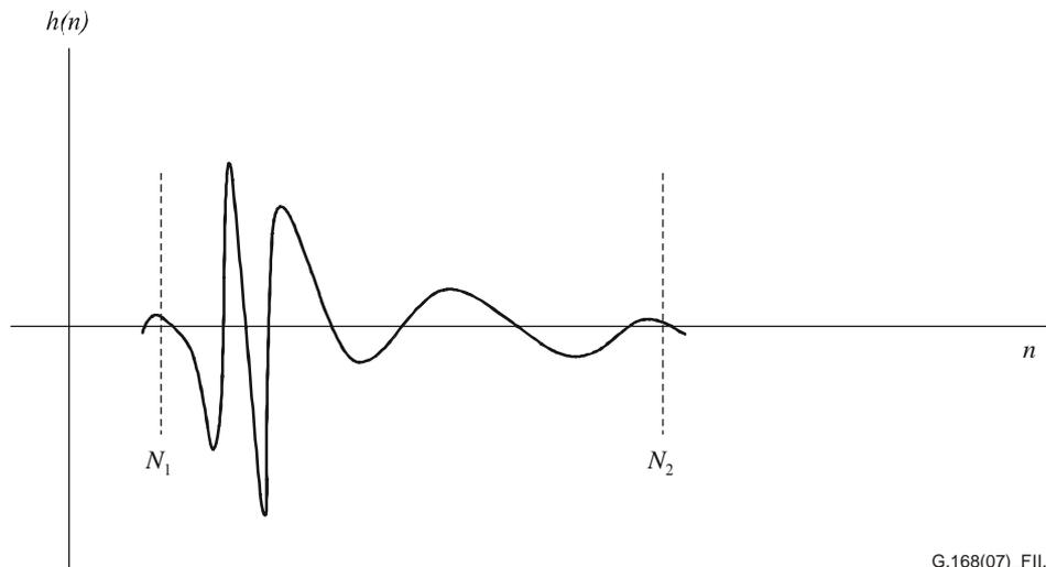
Figure II.5 – Echo-path truncation for dispersion time estimate
