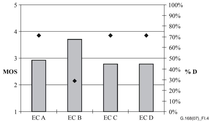
**Figure I.4 – Results from *conversational tests*, overall quality MOS and % D (rhombus) for the 4 echo cancellers, ERL 7 dB, room noise level 40 dB(A), corresponding level –61 dBm0**
