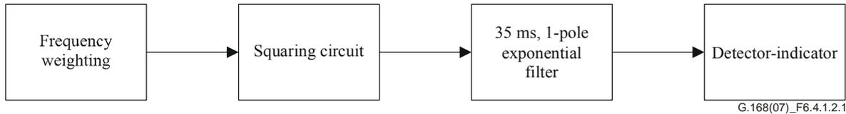
This frequency weighting network is used to provide a greater attenuation of the frequencies outside the band of interest that can be achieved by the filters identified in [IEC 61672-1]. This filter is required because of D.C. effects due to the bias induced by A-law encoding. The filter is a 101-element finite impulse response bandpass filter with the impulse response shown in Figure 4 and the frequency response shown in Figure 5. The coefficients of the filter are:
