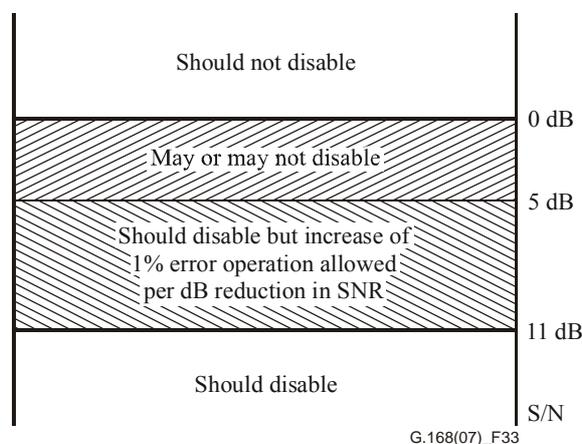
**Figure 33 – Guardband and noise tolerance requirements**
