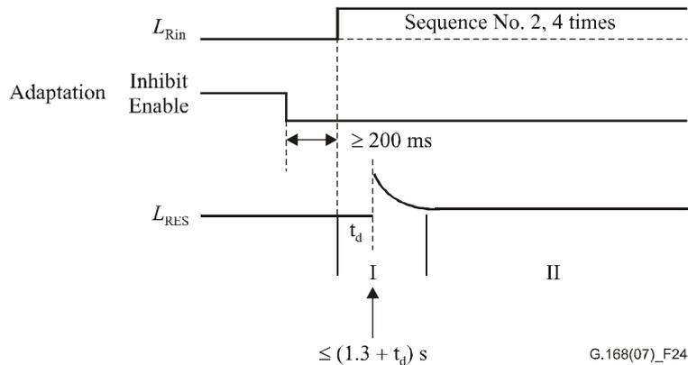
Figure 24 – Test No. 10B signal and time relationships
