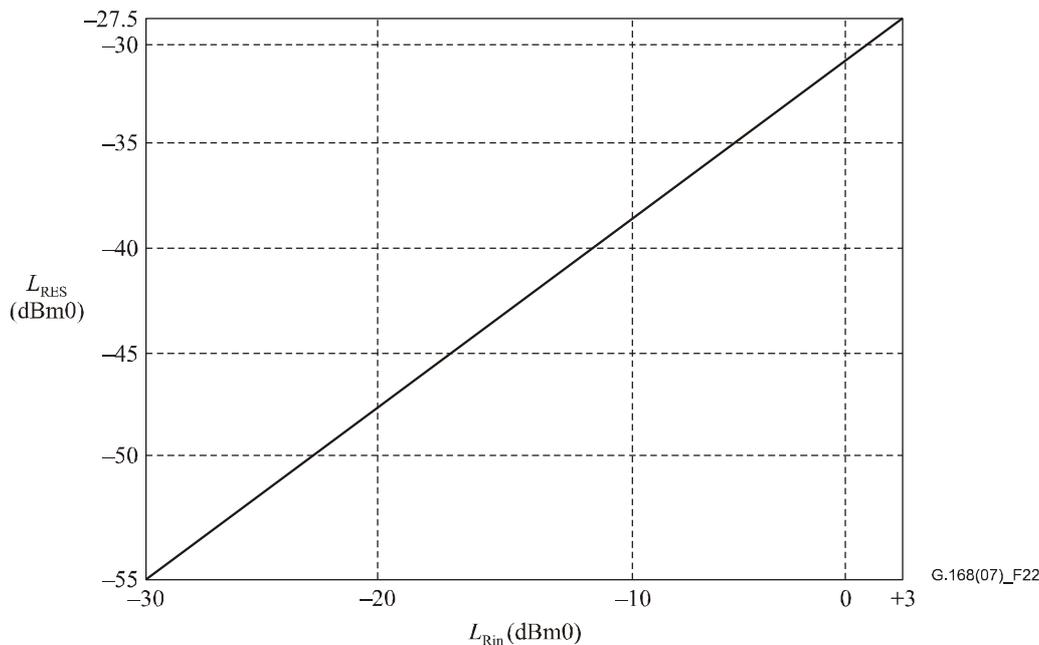
Note that the equation for the line in Figure 22 is:  $L_{RES} = 0.83L_{Rin} - 30$ .
