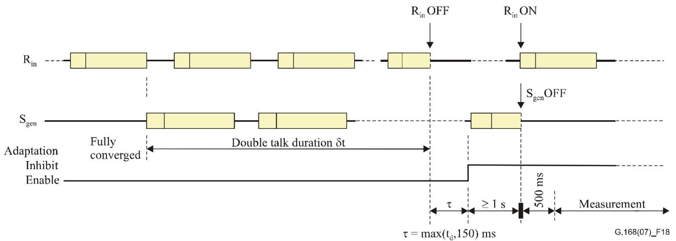
**Figure 18 – Test No. 3B signal and time relationships**
