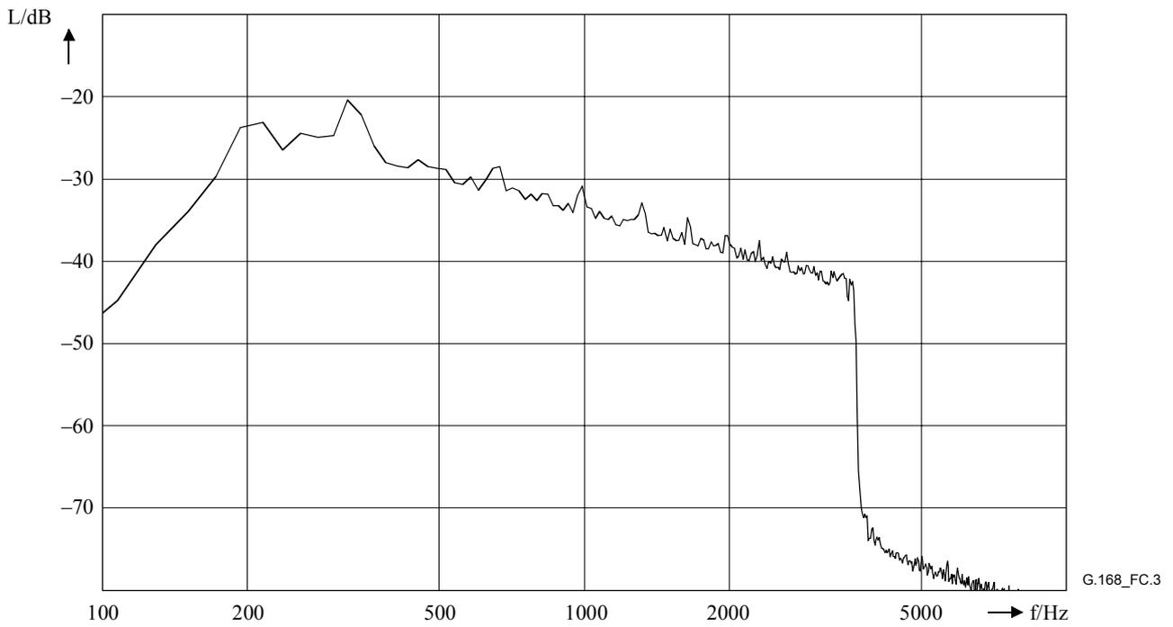
**Figure C.3/G.168 – Power density spectrum of the bandlimited CSS (single talk signal, analysis window: Hanning)**
