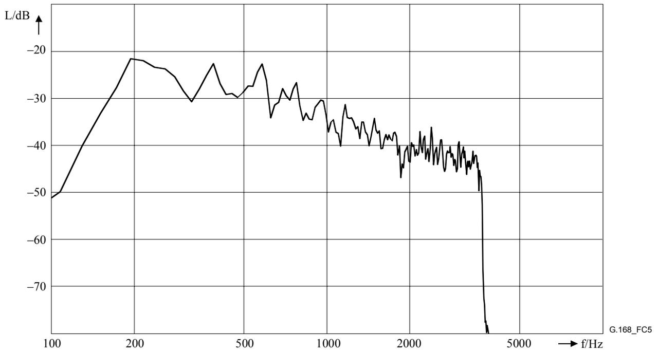
**Figure C.5/G.168 – Power density spectrum of the bandlimited double talk CSS
