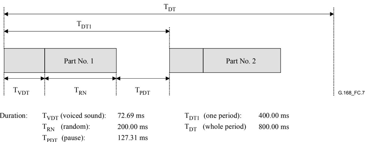
**Figure C.7/G.168 – Composite Source Signals to simulate double talk (schematic)**
