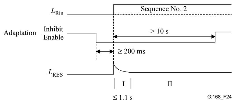
Figure 24/G.168 – Test No. 10B signal and time relationships
