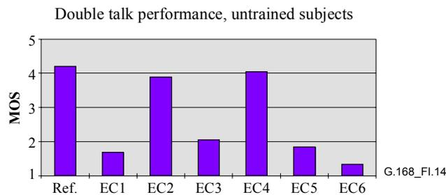
**Figure I.14/G.168 – Results from listening-only tests, untrained subjects, double talk performance MOS, ERL 24 dB, receive level  $-15$  dBm0, double talk level  $-30$  dBm0**
