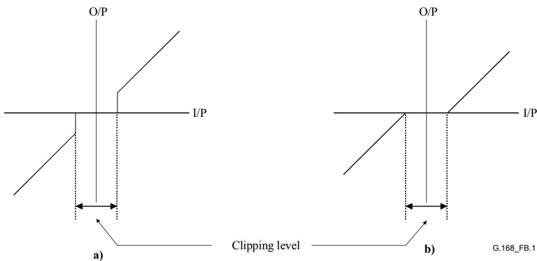
**Figure B.1/G.168 – Two examples of idealized center clipper transfer function**
