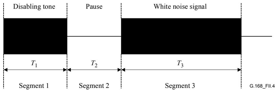
Figure II.4/G.168 – Test signal for echo-path measurement
