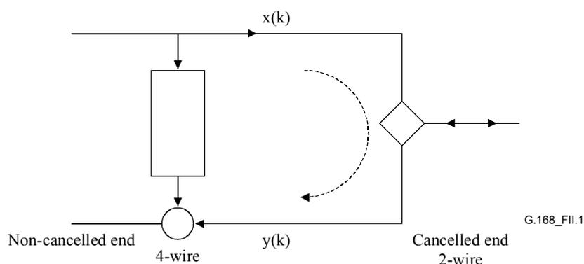
Figure II.1/G.168 – A typical call connection
