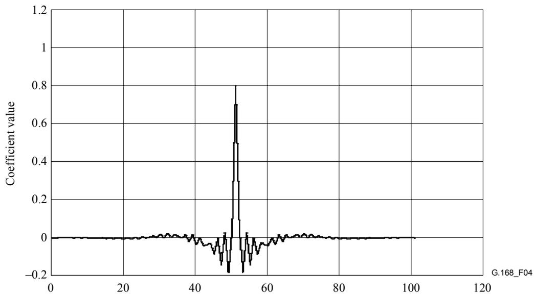
**Figure 4/G.168 – Impulse response of frequency weighting network**
