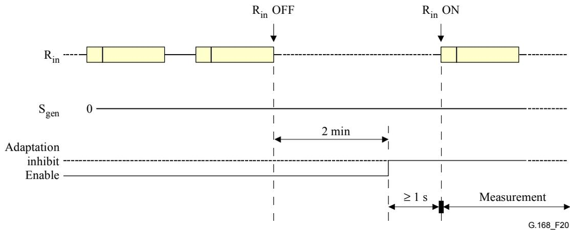
**Figure 20/G.168 – Test No. 4 signal and time relationships**
