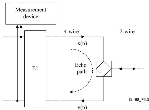
Figure II.3/G.168 – Block diagram of non-intrusive measurement set-up
