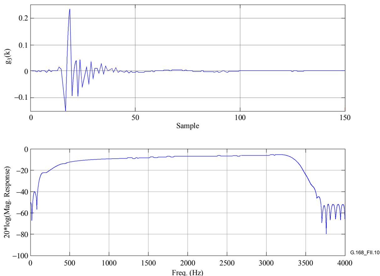
**Figure II.10/G.168 – Echo path impulse response  $g_3$ , an ERL of 12 dB was used in the magnitude response plot**
