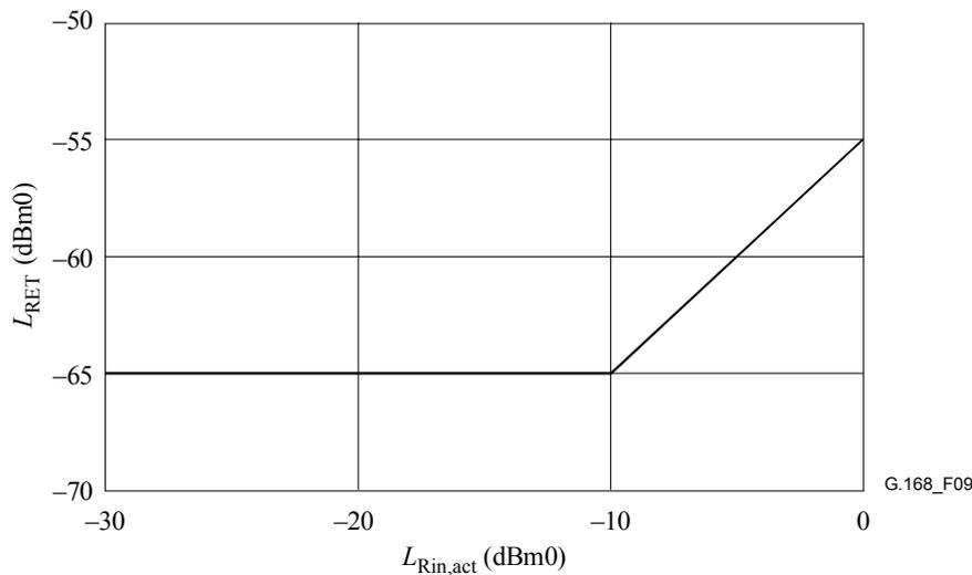
**Figure 9/G.168 – Relationship between receive input level ( $L_{Rin,act}$ ) and return echo level ( $L_{RET}$ ) with NLP enabled**
