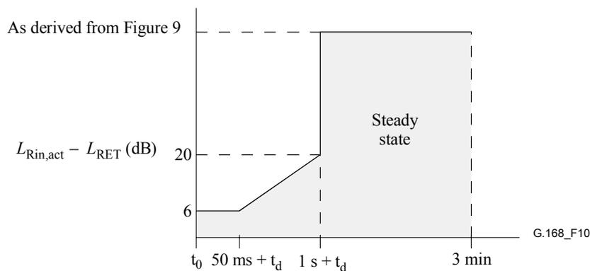
**Figure 10/G.168 – Convergence characteristics with NLP enabled**
