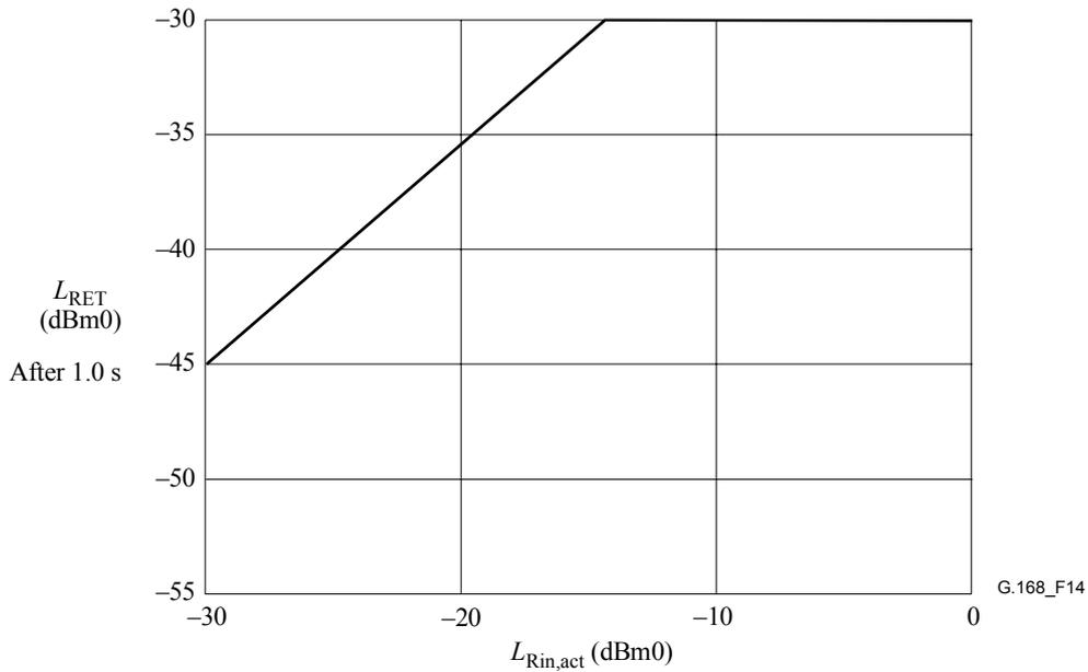
Figure 14/G.168 – Test No. 2C requirements NLP enabled
