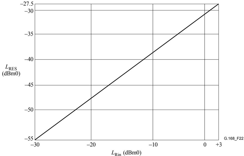
**Figure 22/G.168 – Performance requirements for test 7**
