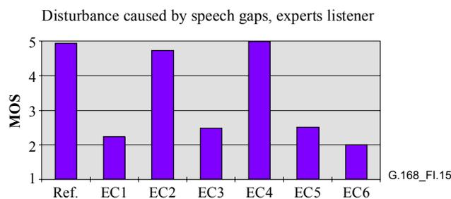
**Figure I.15/G.168 – Results from listening-only tests, experts, disturbances during double talk caused by speech gaps MOS, ERL 24 dB, receive level  $-15$  dBm0, double talk level  $-30$  dBm0**
