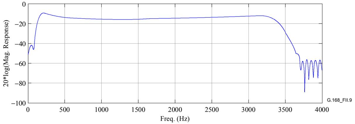
**Figure II.9/G.168 – Echo path impulse response  $g_2$ , an ERL of 12 dB was used in the magnitude response plot**
