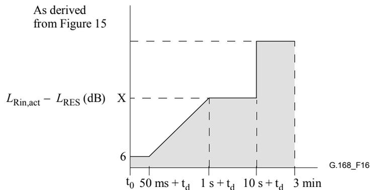
**Figure 16/G.168 – Test No. 2C Convergence requirements NLP disabled**
