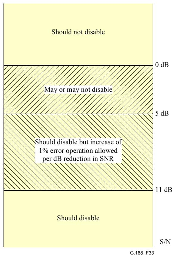
**Figure 33/G.168 – Guardband and noise tolerance requirements**
