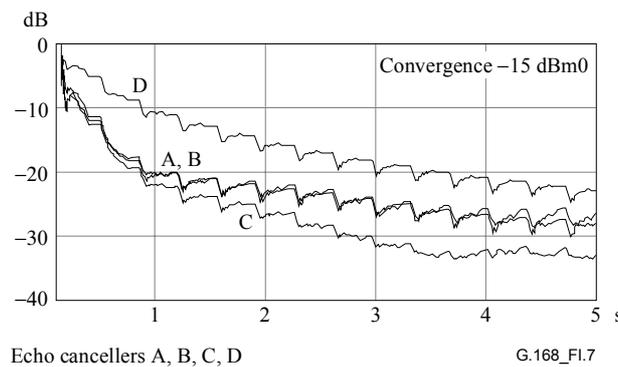
**Figure I.7/G.168 – Convergence test versus time, digital echo path, ERL 6 dB, no cancelled end background noise, receive level -15 dBm0, NLP disabled**
