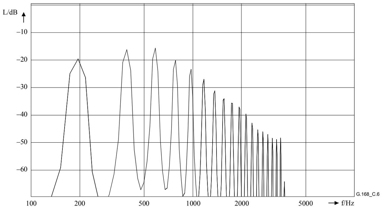
**Figure C.6/G.168 – Power density spectrum of the bandlimited double talk voiced signal
