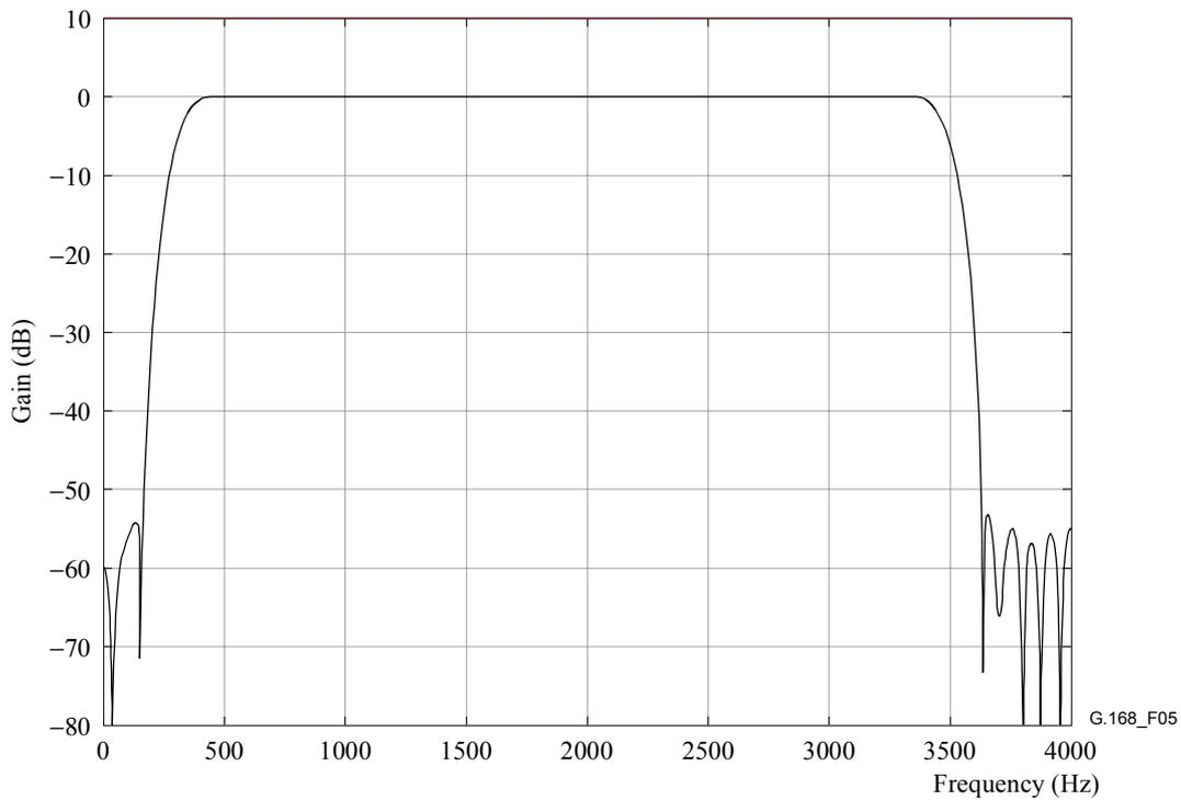
**Figure 5/G.168 – Magnitude response of frequency weighting network**
