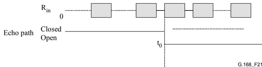
**Figure 21/G.168 – Test No. 5 signal and time relationships**
