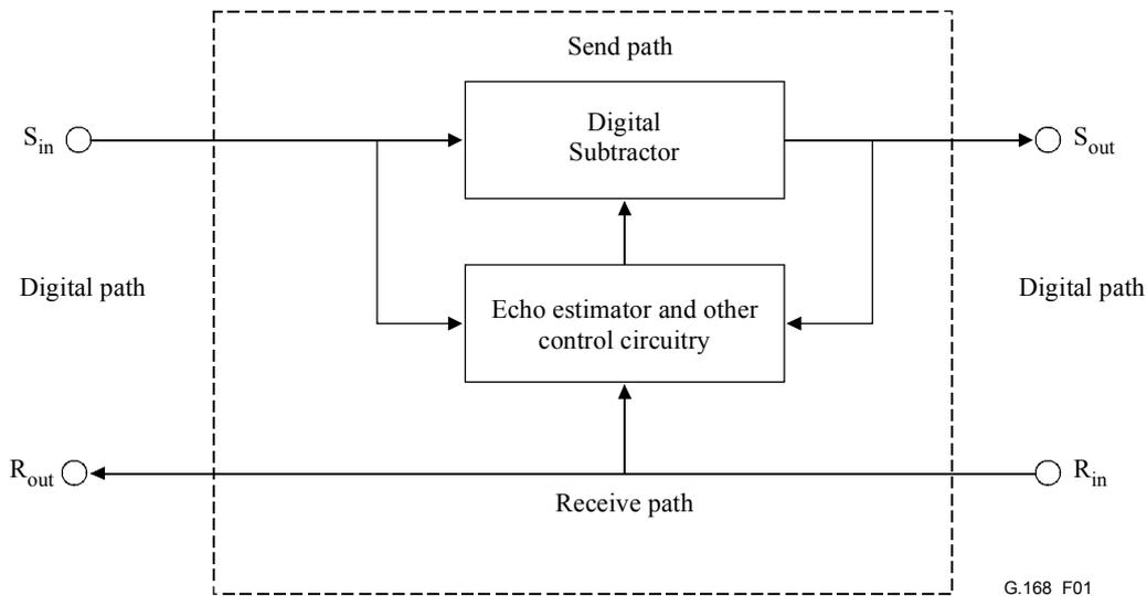
Figure 1/G.168 – Digital transmission echo canceller using digital subtraction
