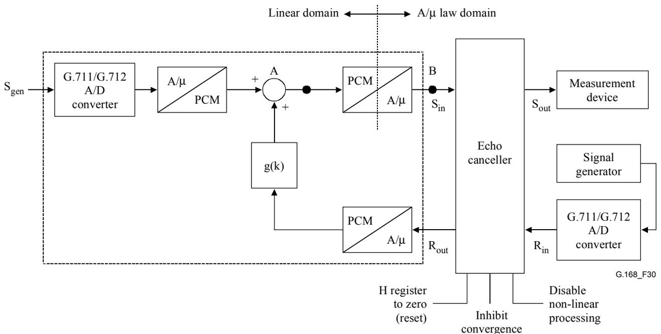
Figure 30/G.168 – Test configuration for  $S_{in}$  PCM offset test
