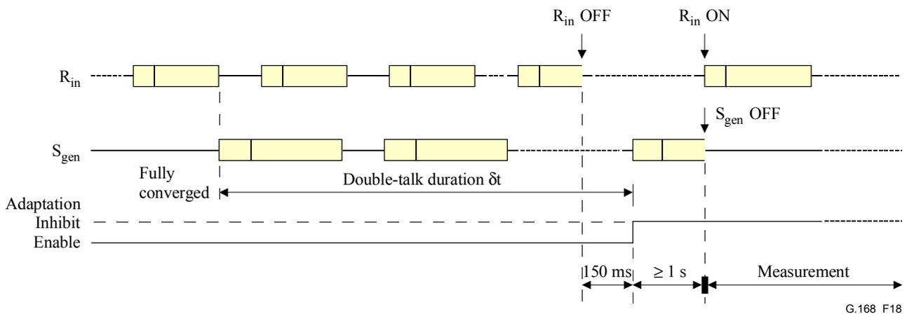
**Figure 18/G.168 – Test No. 3B signal and time relationships**
