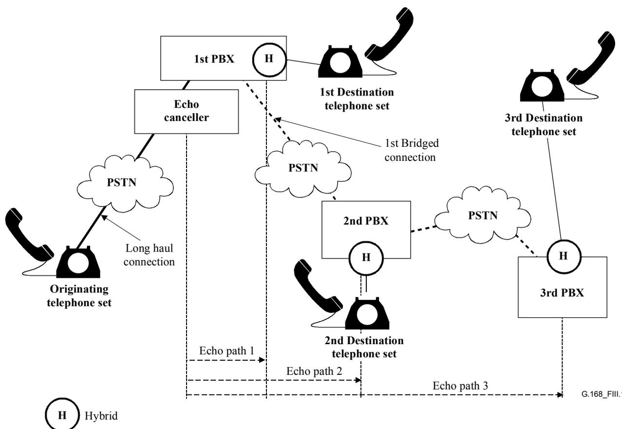
Figure III.1/G.168 – Multiple tails in a typical bridged telephone call
