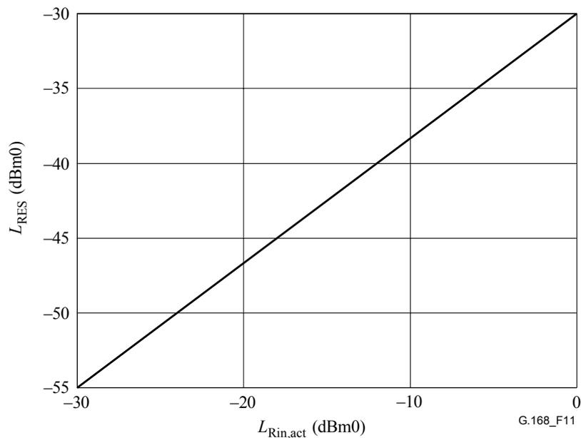
**Figure 11/G.168 – Relationship between receive input level ( $L_{Rin,act}$ ) and residual echo level ( $L_{RES}$ ) with NLP disabled**
