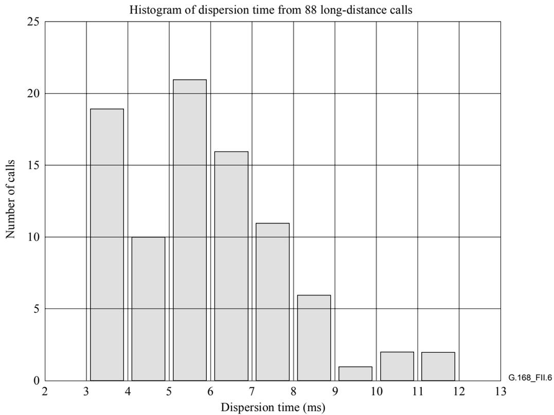
**Figure II.6/G.168 – Histogram of dispersion time for long-distance calls:
