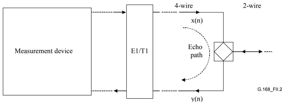
Figure II.2/G.168 – Block diagram of intrusive measurement set-up
