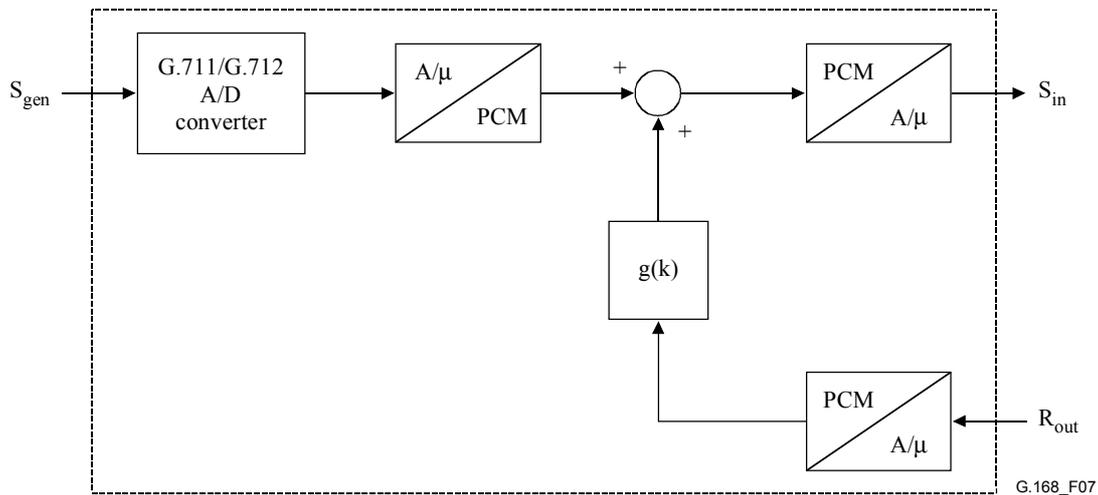
**Figure 7/G.168 – Echo path model using  $g(k)$**
