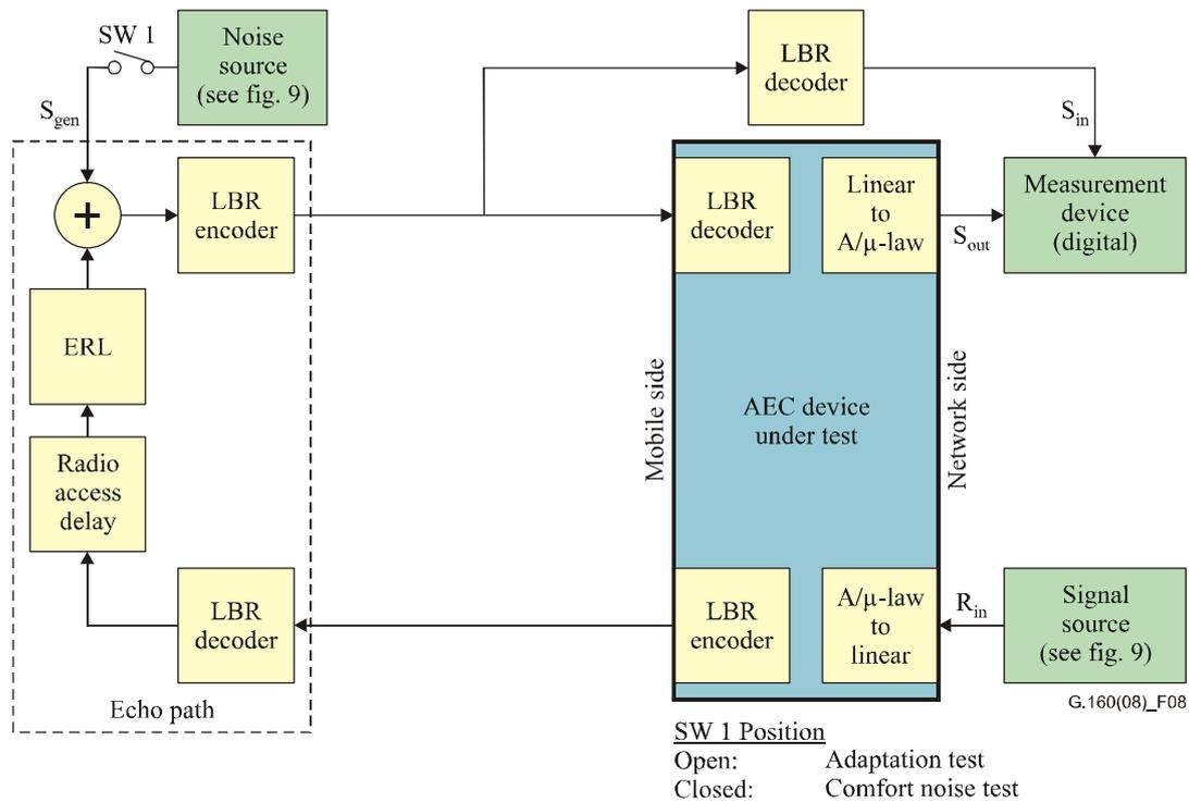
**Figure 8 – Test set-up in which AEC provides LBR encoded connection to mobile direction**
