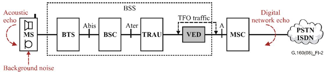
NOTE – Dedicated configuration located on the A interface. If TFO protocol is not terminated, the VED will provide a transparent channel for each connection in TFO mode. The referring OMC is the BSS-OMC.
