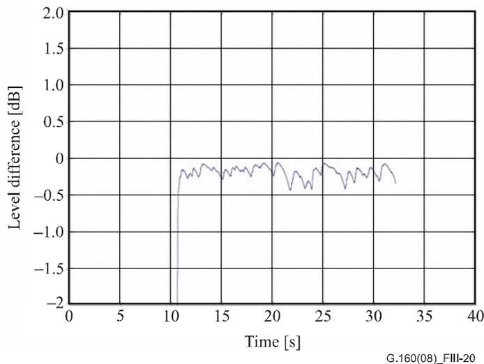
**Figure III.20 – Difference between the NR output and clean signal from Figure III.19**
