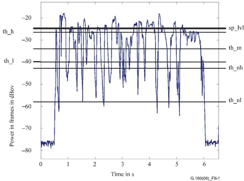
**Figure II.1 – Power in frames of clean speech as a function of time – Classification into power classes**
