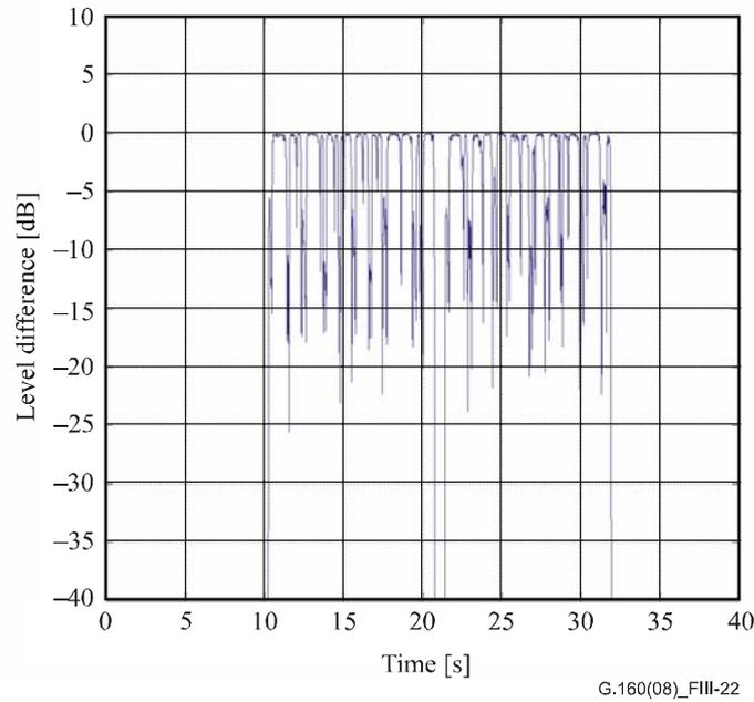
**Figure III.22 – Difference between the NR output and clean signal from Figure III.21**
