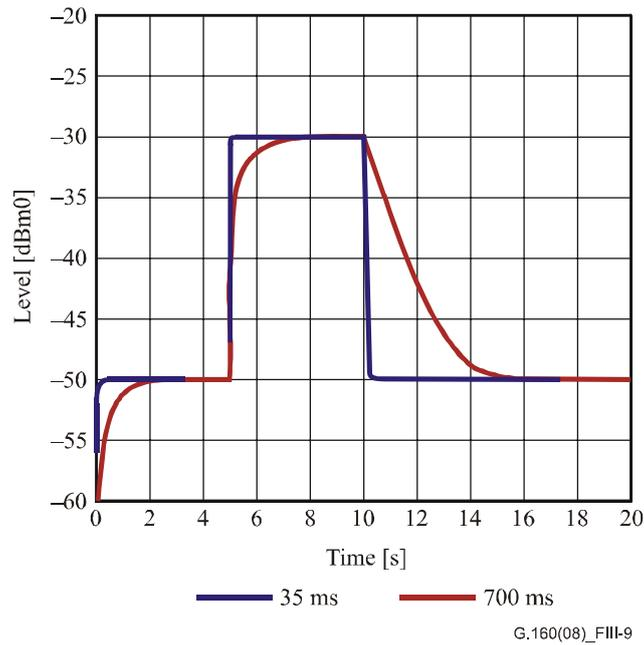
**Figure III.9 – Reaction of exponential level measurement device to step changes (logarithmic scale)**
