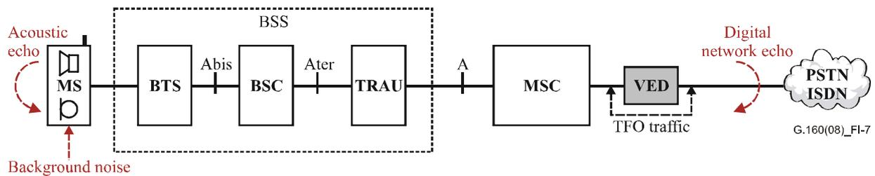
NOTE – Dedicated located on the PSTN interface. This configuration does not allow voice enhancement for mobile-to-mobile calls. No interaction is possible with TFO protocol. The referring OMC is the MSC-OMC.
