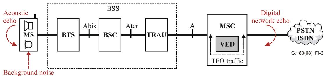
NOTE – Dedicated or pool configuration located inside MSC. If TFO protocol is not terminated, the VED will provide a transparent channel for each connection in TFO mode. The referring OMC is the MSC-OMC.
