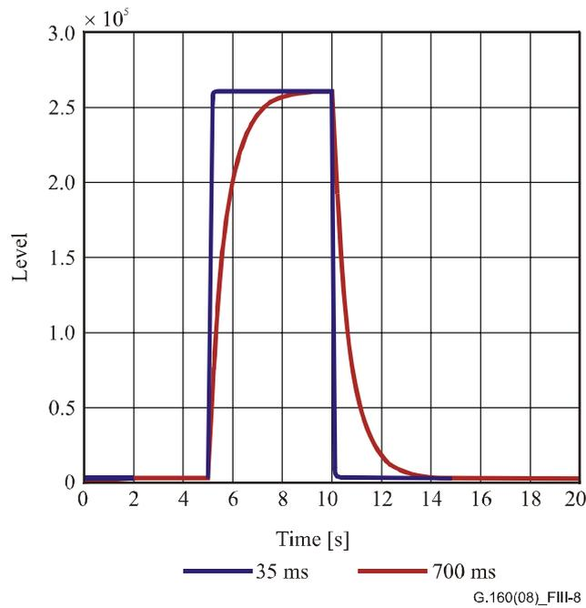
**Figure III.8 – Reaction of exponential level measurement device to step changes (linear scale)**
