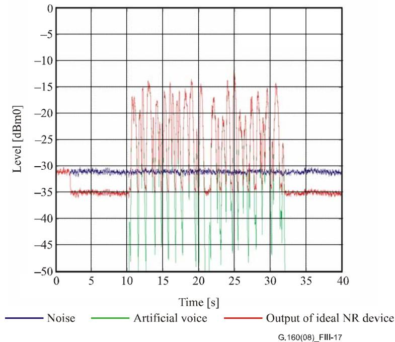
**Figure III.17 – Level measurement using exponential averaging and 35 ms time constant**
