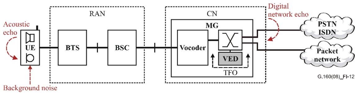
**Figure I.12 – Block diagram of VED location in CDMA2000 3G mobile network, configuration 1**
