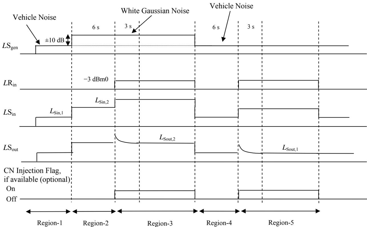
NOTE – The  $S_{in}$  signal is the sum of the  $S_{gen}$  signal and the acoustic echo resulting from  $R_{in}$ . Hence, the level of  $S_{in}$  is higher than the level of  $S_{gen}$  when  $R_{in}$  is not silence.
