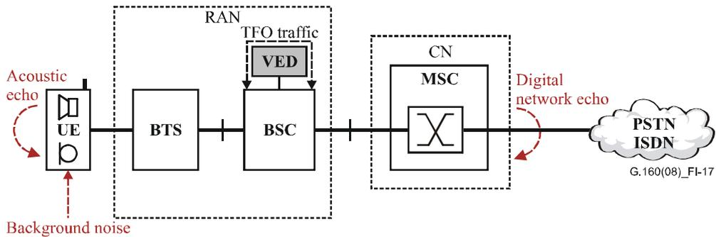
NOTE – The CDMA selection function and vocoder are both in BSC in this case.
