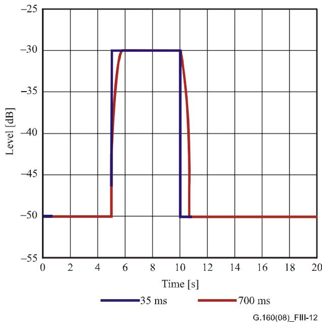
**Figure III.12 – Reaction of RMS level measurement device to step changes (logarithmic scale)**
