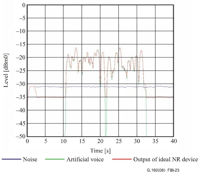
**Figure III.23 – Level measurement using RMS method with 700 ms window**
