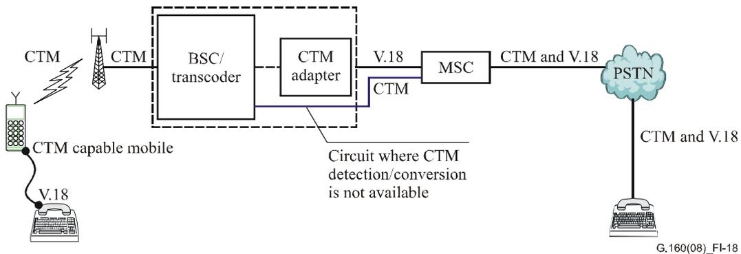
**Figure I.18 – CTM adapter present on specific A-interface circuits – 2G mobile network**
