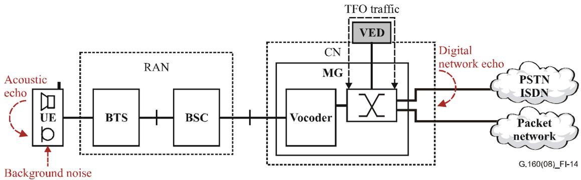
**Figure I.14 – Block diagram of VED location in CDMA2000 3G mobile network, configuration 3**
