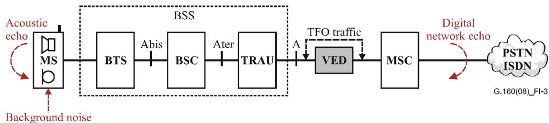
NOTE – Dedicated configuration located on the A interface. If TFO protocol is not terminated, the VED will provide a transparent channel for each connection in TFO mode. Same location as Figure I.2, but, in this case, the referring OMC is the MSC-OMC.
