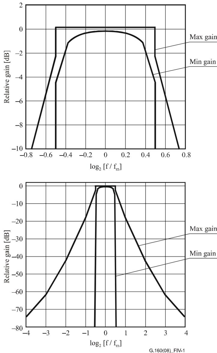
**Figure IV.1 – Specification of the class 0 attenuation characteristics for the octave-band filters**
