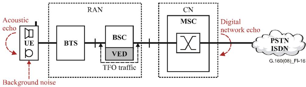
NOTE – The CDMA selection function and vocoder are both in BSC in this case.
