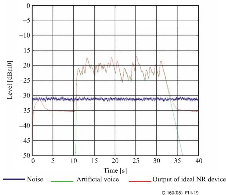
**Figure III.19 – Level measurement using exponential averaging and 700 ms time constant**
