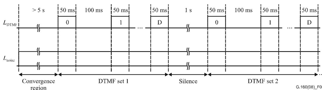
**Figure 2 – Timing relationships for the DTMF tones test
