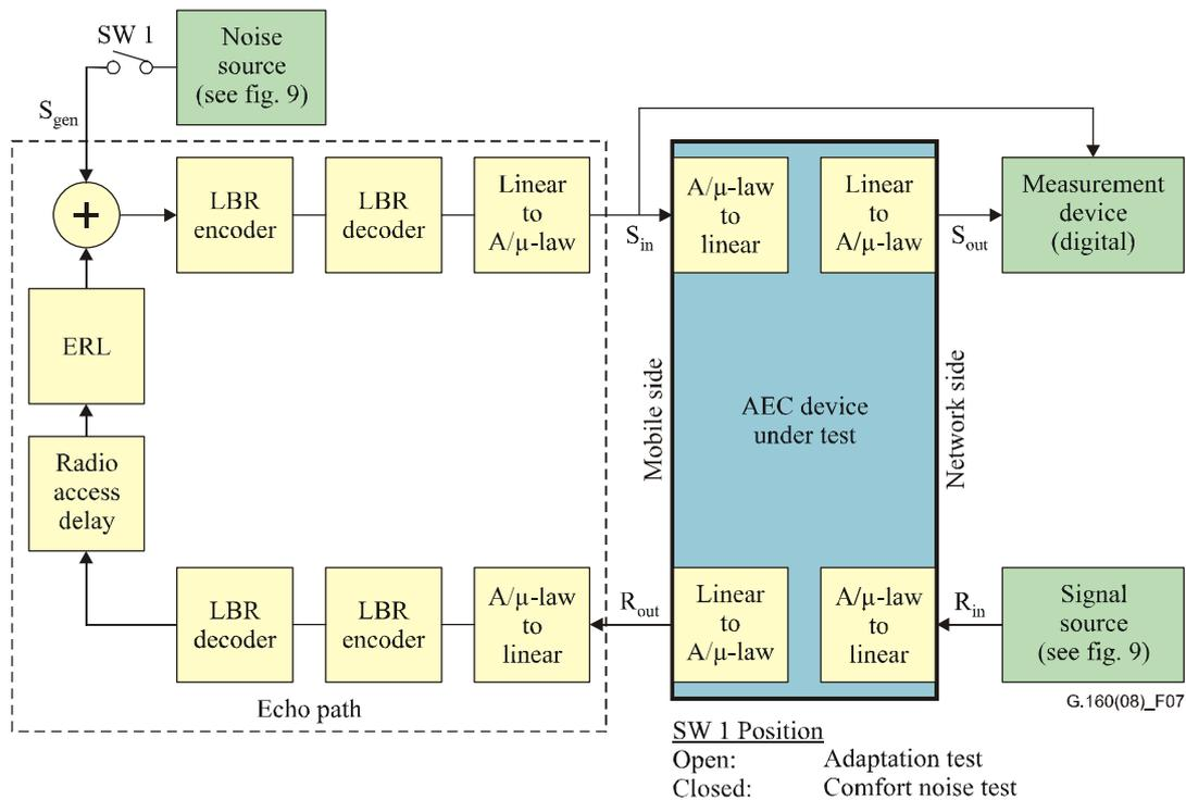
**Figure 7 – Test set-up in which AEC provides G.711 connection to mobile direction**
