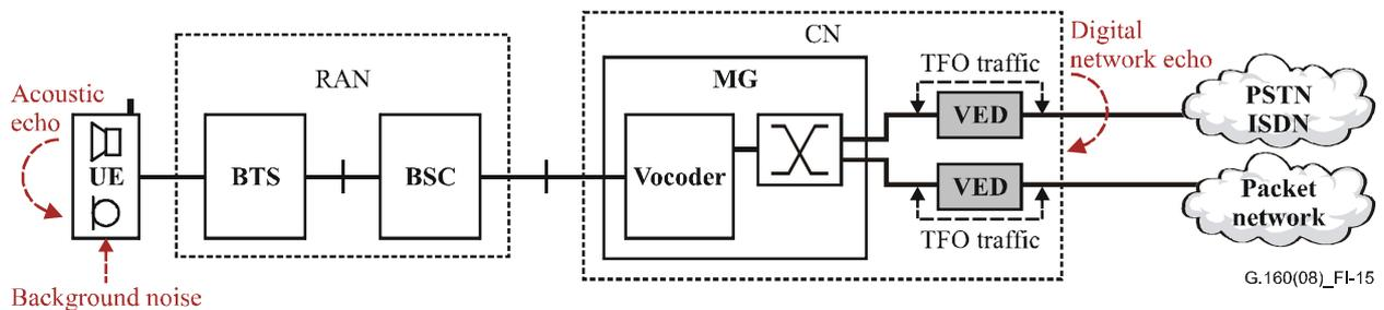
**Figure I.15 – Block diagram of VED location in CDMA2000 3G mobile network, configuration 4**
