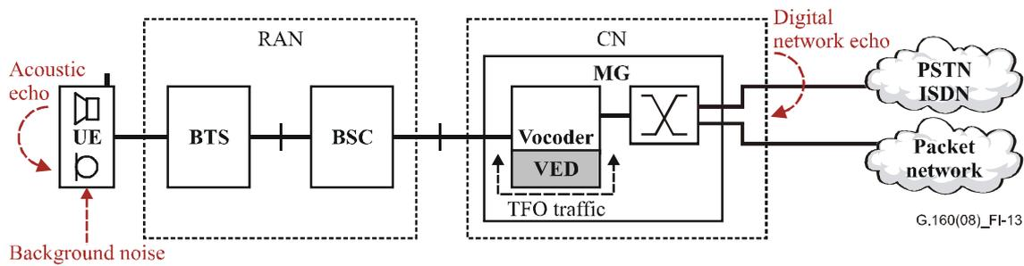
**Figure I.13 – Block diagram of VED location in CDMA2000 3G mobile network, configuration 2**
