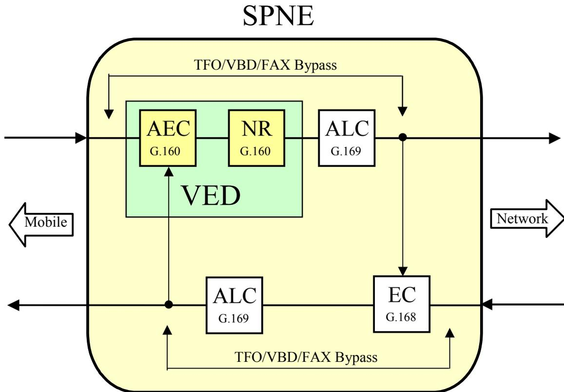
Figure I.1 – Example block diagram showing the presence of a VED in a SPNE
