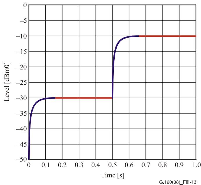
**Figure III.13 – Measured levels of two signals delayed by 1 ms**
