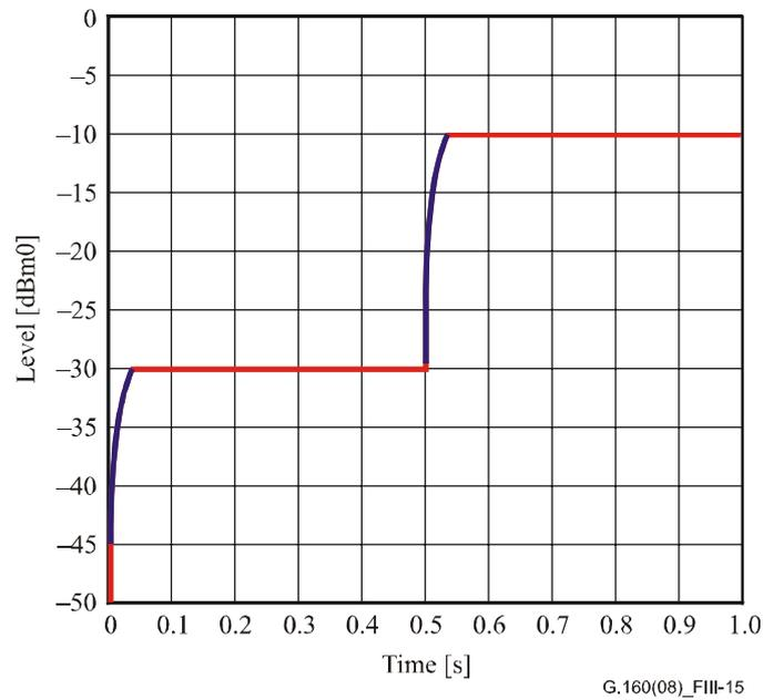
**Figure III.15 – Measured levels of two signals delayed by 1 ms with RMS method**
