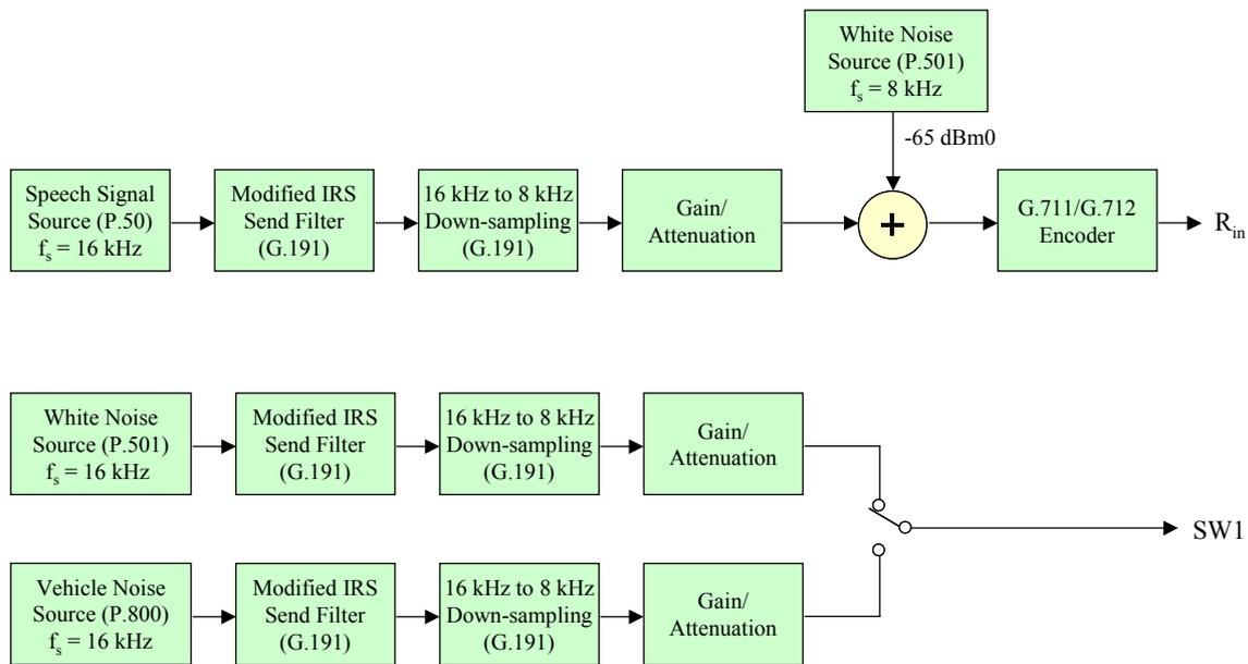
**Figure 9 – Details of signal and noise source pre-processing**
