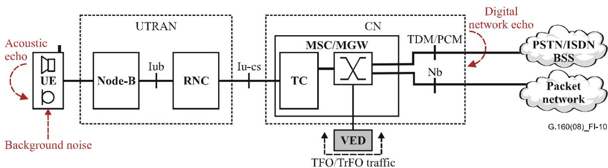
NOTE 1 – VED in dedicated or pool configuration with external equipment connected to MGW. The referring OMC is the MGW-OMC.
