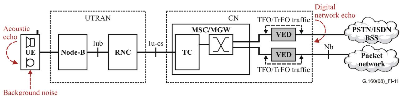
NOTE 1 – Dedicated configuration located on the PSTN interface. On packet-oriented interface, there is the possibility to have compressed speech. In such a case, the VED will provide a transparent channel. The referring OMC is the MSC/MGW-OMC.
