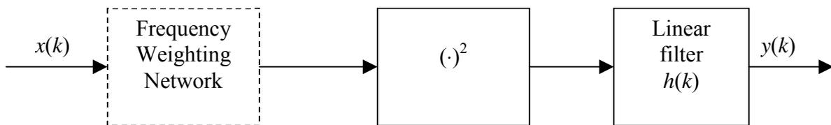
Figure III.1 – Level measurement device
