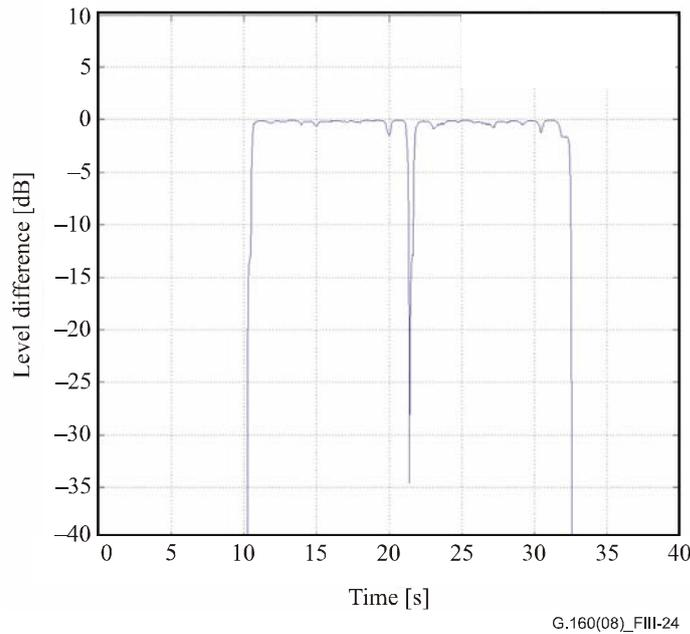
**Figure III.24 – Difference between the NR output and clean signal from Figure III.23**
