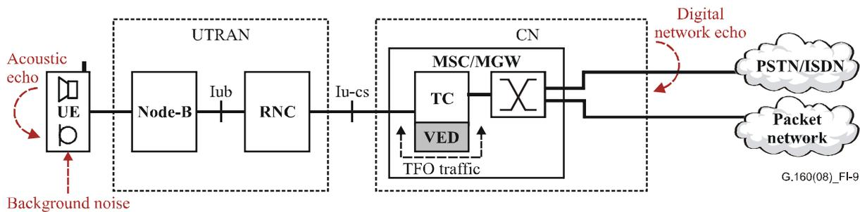
NOTE 1 – Dedicated configuration located on the TC equipment. The referring OMC is the MGW-OMC. In this scenario, the VED may be located anywhere within the TC, and its exact location will determine whether or not it needs to implement TFO detection.
