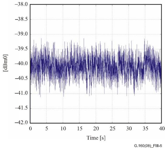
**Figure III.5 – Level measurement of a white Gaussian noise realization using exponential averaging and 35 ms time constant**
