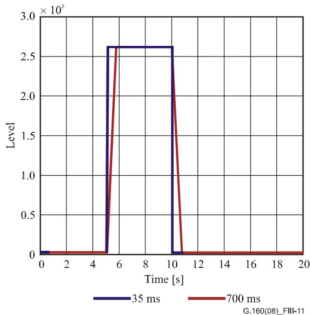
**Figure III.11 – Reaction of RMS level measurement device to step changes (linear scale)**
