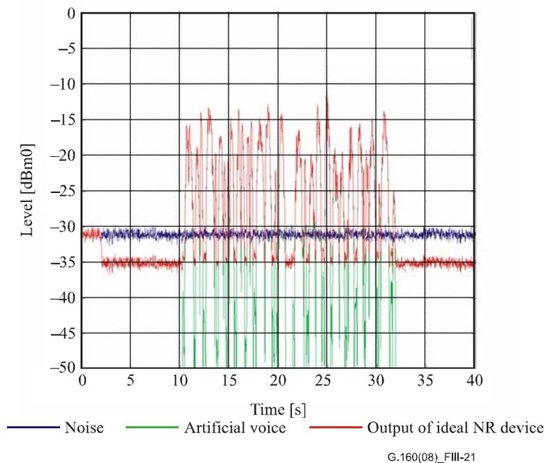
**Figure III.21 – Level measurement using RMS method with 35 ms window**
