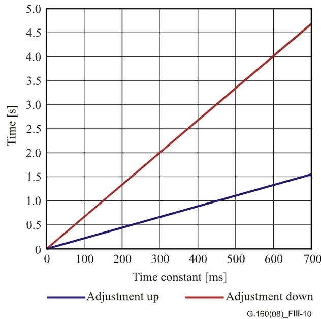
**Figure III.10 – Transition time into 0.5 dB vicinity from the target as a function of time constant**
