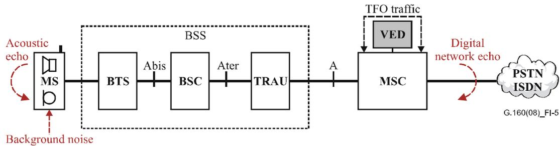
NOTE – Dedicated or pool configuration with external equipment connected to MSC. If TFO protocol is not terminated, the VED will provide a transparent channel for each connection in TFO mode. The referring OMC is the MSC-OMC.
