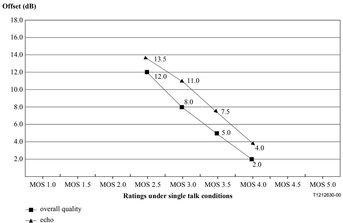
**Figure II.3/G.131 – Echo level offset during double talk to achieve the same MOS values compared to the single talk condition (transmission time: 100 ms)**
