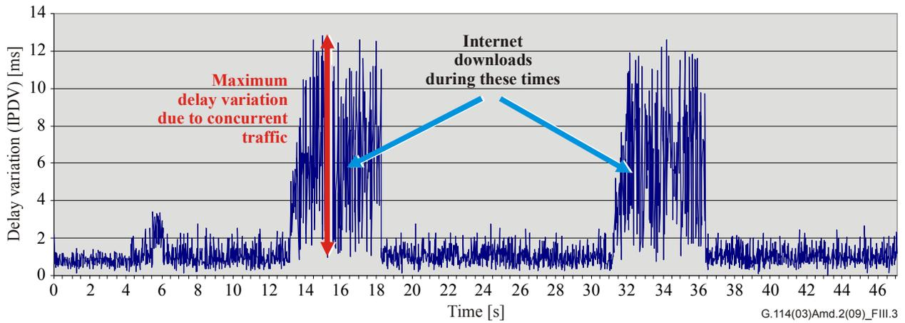
**Figure III.3 – Delay variation (IPDV) of a call A to B, with parallel download at B**
