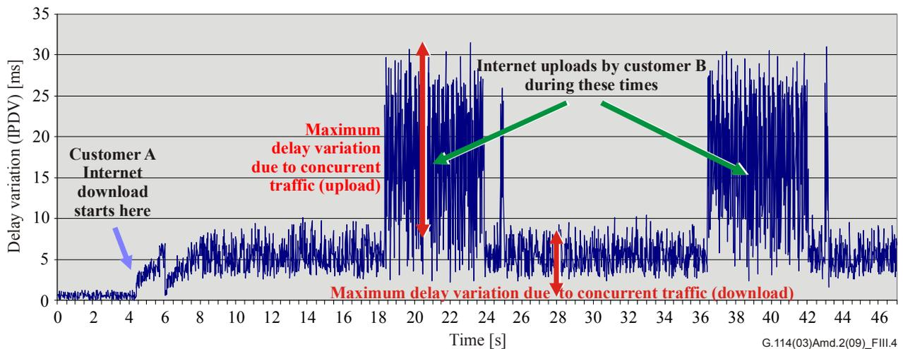
**Figure III.4 – Delay variation (IPDV) of a call B to A with parallel download at A and upload at B**
