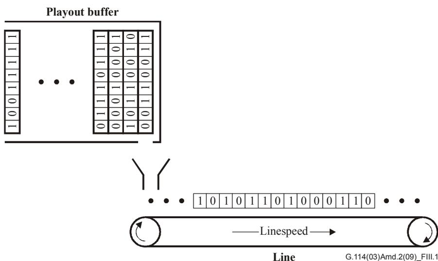
Figure III.1 – Serialization delay
