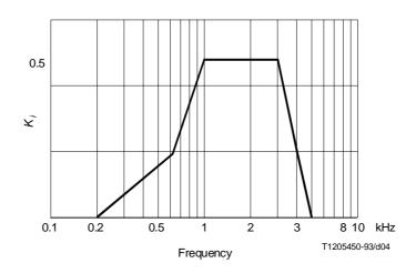
FIGURE A.2/G.111 Sidetone weighting  $K_i$  as given in Table A.1
