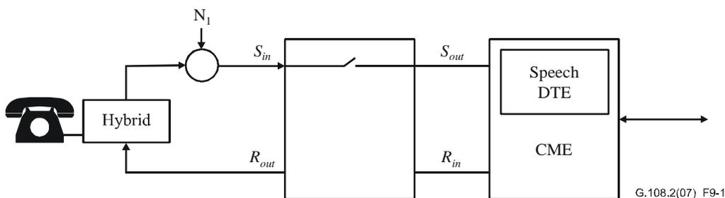
**Figure 9-1 – Speech detector/echo control device interaction**
