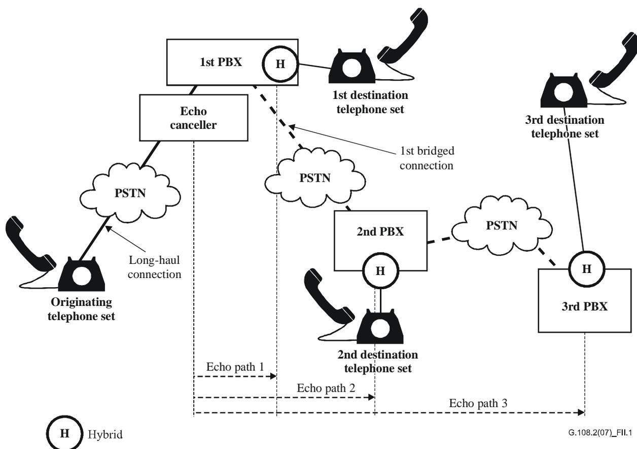
Figure II.1 – Multiple tails in a typical bridged telephone call
