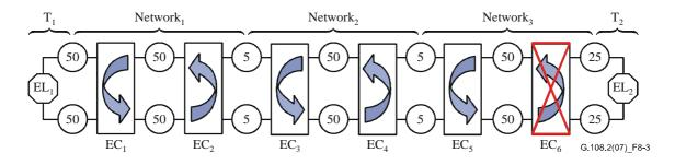
Figure 8-3 – Example of connection via three concatenated networks including a cellular network
