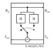
Figure 8-5 – Possible implementation of echo canceller with two independent H echo-path estimators
