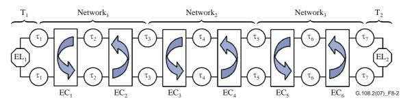
Figure 8-2 – Reference connection for tandem ECs
