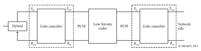
Figure 8-1 – Low bit-rate coder between tandem cancellers
