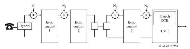
Figure 9-2 – Multiple echo control devices in a CME network configuration
