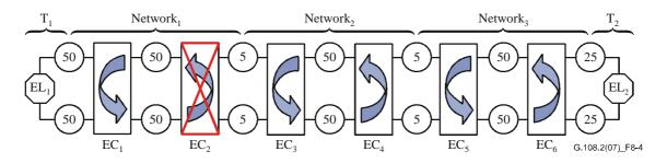
Figure 8-4 – Example of connection via three concatenated networks including a private network
